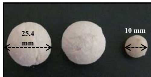
Figure 3.4 Octadecane-sand lumps (before and after ablation)
