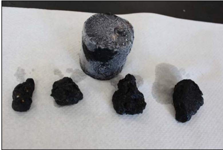
Figure 4.2 Oil sand lumps remaining after different ablation experiments
