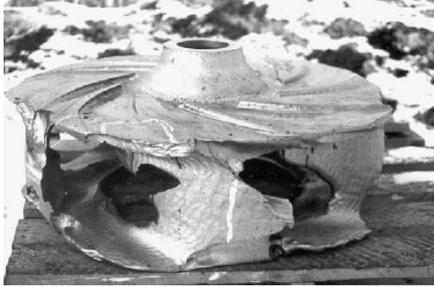
Figure 2.13: A HCCI worn impeller after 3 months of use in oil sands slurry pumps [4].
