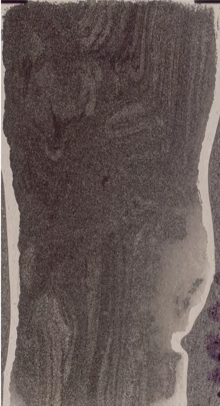
**Figure 1-25** Thin section image showing a central conical shaped laminae disturbance interpreted as *Lingulichnus*. This sample is from 1986 m depth within well d-48-A/94-b-9.
