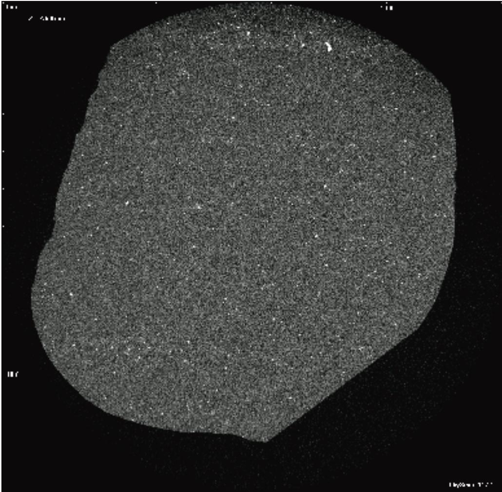
**Figure 2-1** Greyscale image taken using micro-ct. Shade is determined by density via atomic number; the denser the mineral, the lighter the grey. Note the bright white spots are pyrite, the most dense of the observable mineral phases. Calcite appears as light grey and is seen to be concentrated within laminae. Dolomite, quartz and feldspar are more difficult to distinguish within this image because the attenuation coefficients are closer in value.
