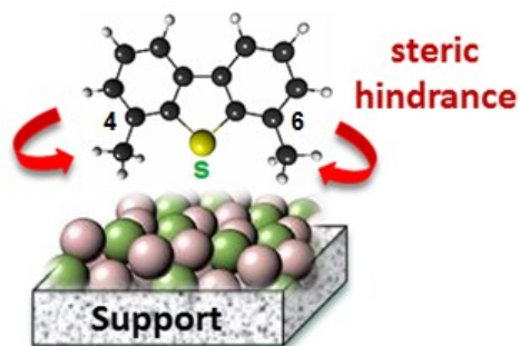
Scheme 1.1. Steric hindrance effects of alkyl groups on the adsorption of 4,6-DMDBT on the active sites.
