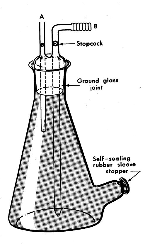
Figure 5.6. Schematic diagram of the anaerobic culture flask
