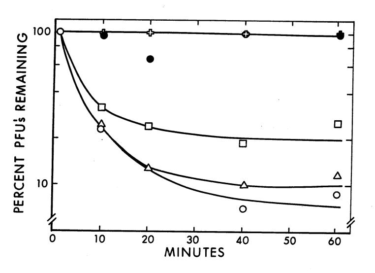
Figure 5.12. The effect of sodium arsenate on the ability of E. coli K12 (grown in glycerol TMM) to uncoat R17 RNA
