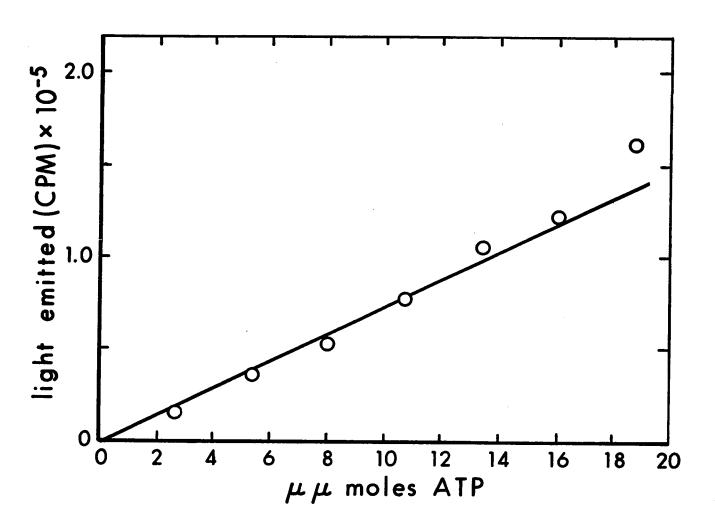
Figure 5.3. Calibration curve for the assay of  $\mu\mu$ mole quantities of ATP
