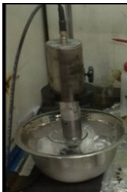
Figure 30. The sonication of GNP under the ice bath.
