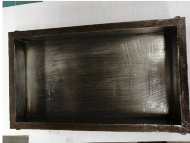
Figure 35. The shape of the custom-made cuboid steel mold.
