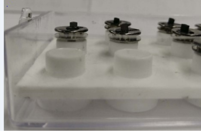
Figure 6. Gold-coated tensile fractured specimens for SEM testing.
