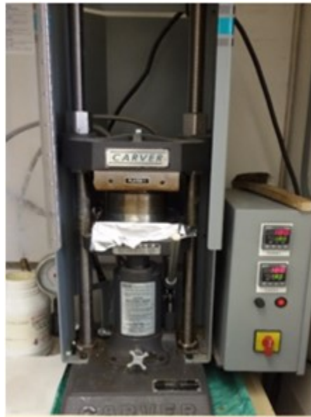
Figure 34. Hot pressing GNP/PLA samples.
