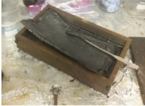
Figure 33. Evaporating the solvent in steel mold.
