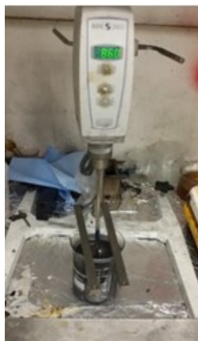
Figure 32. The mechanical stirring of GNP/PLA/chloroform mixture.
