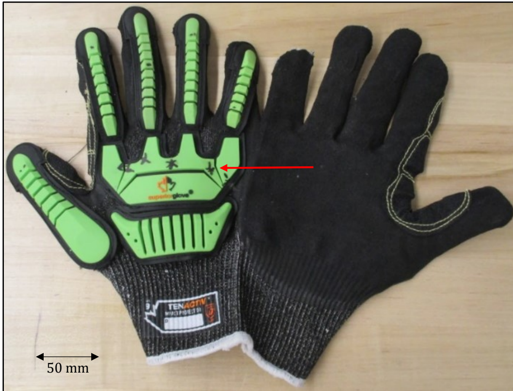
Figure 2.2: A glove specimen prepared for testing. The impact test sites have been marked (red arrow indicates one marking) for testing and the glove has been cut open to allow the glove to lie flat on the apparatus.
