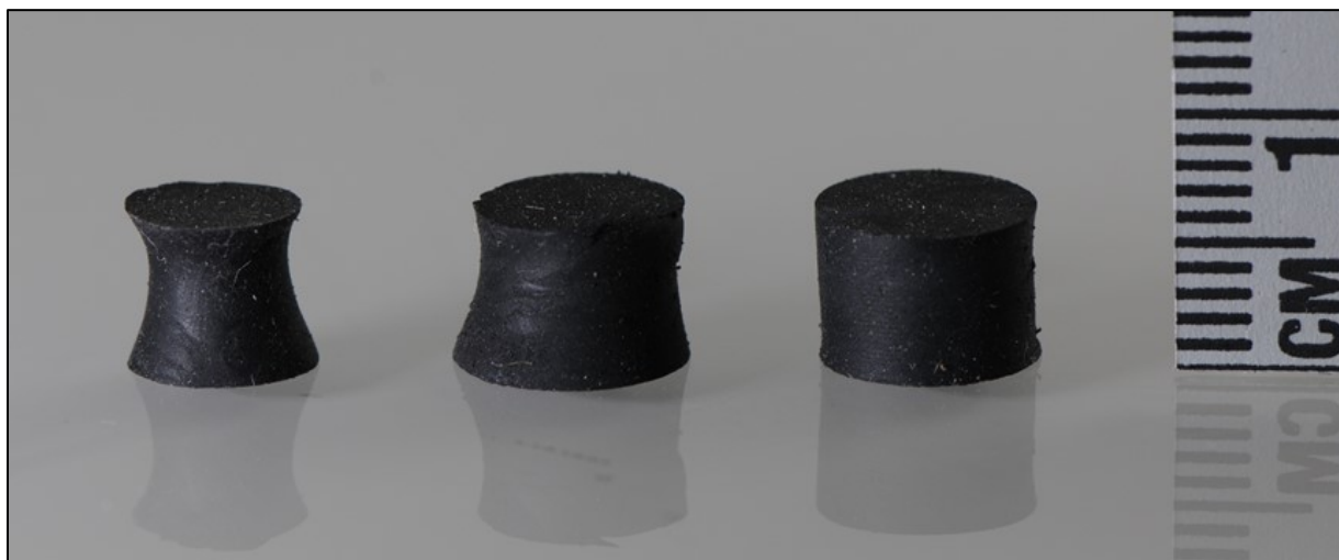
Figure 3.12: the results of the specimens being hand cut (far left) and cut with the drill press without a water bath (middle) and with a water bath (far right). The specimen that was cut with a drill press and water bath was used in DMA testing due to the uniform profile.
