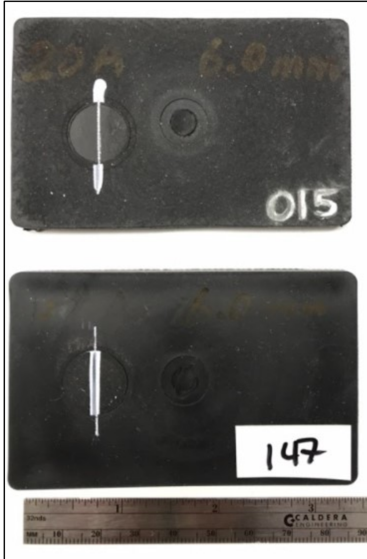
Figure B.15: The specimens used for swapping plugs. The top specimen is a 20 A TPR 6 mm thick and the bottom specimen is a 50 A TPR 6mm thick. The plugs were marked with a paint pen to ensure the same orientation was kept when they were swapped.
