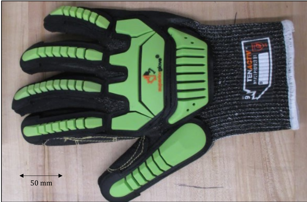
Figure 1.1: A impact resistant glove. The bumpers (green) are used to absorb the impacts.
