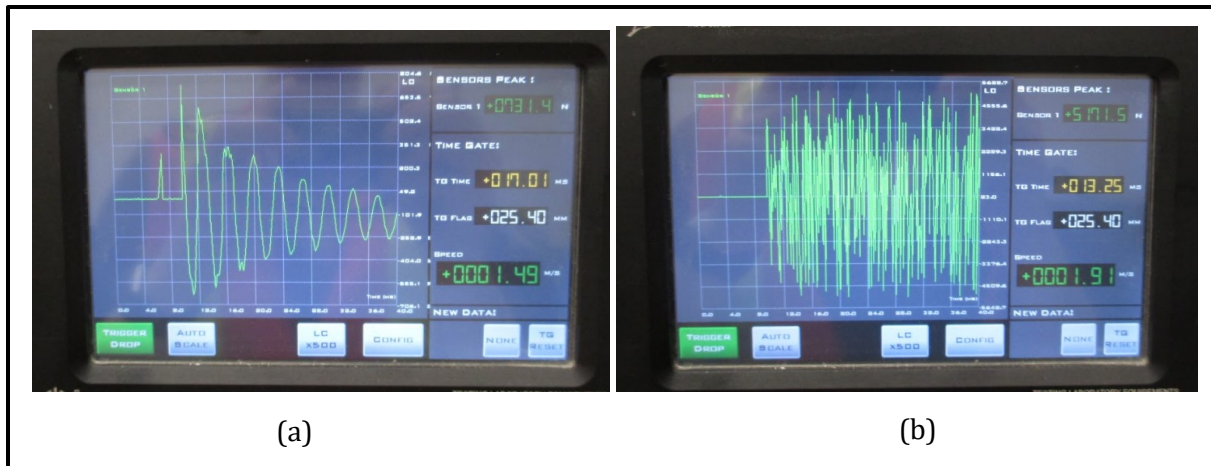
Figure 3.7: Examples of incorrect readings. If a test produced a reading shown in the Figure, it was deemed void.
