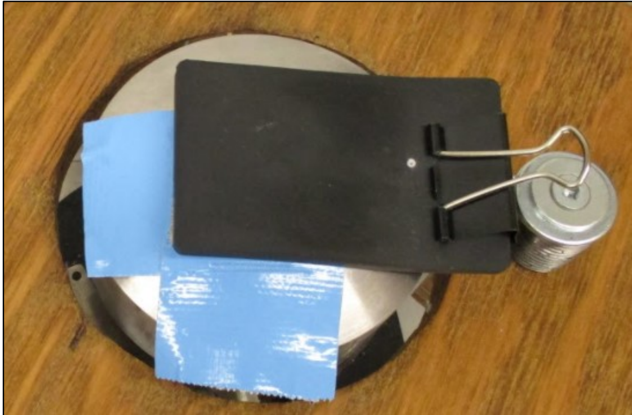
Figure 3.9: A example of how the ARIT tests were set up. A clip was used to hold the specimen in place and two pieces of tape were aligned along the edges to ensure minimal movement of the specimen.
