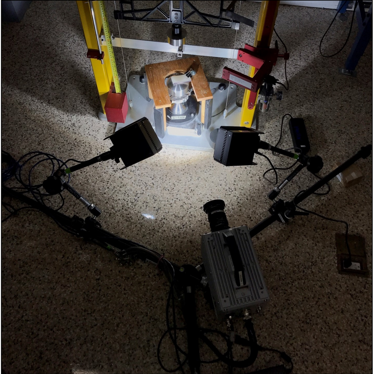
Figure 3.11: A photograph of the HSV set up for the drop testing.
