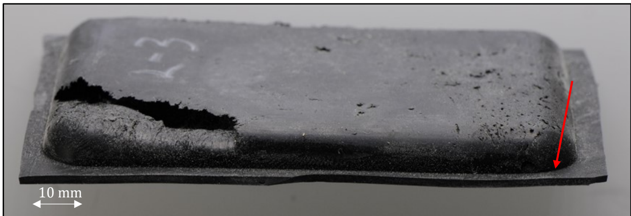
Figure 4.9: The result of the heat pressed halobutyl rubber. The specimen displayed large voids and a lack of thickness precision, as seen from the flashing that developed on the specimen (indicated).
