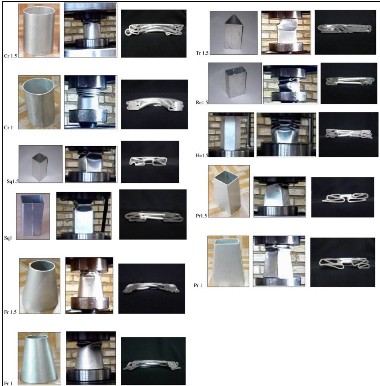
Figure 2.19: The different geometries of specimens tested by Alavi, Nia and Hamedani [31].
