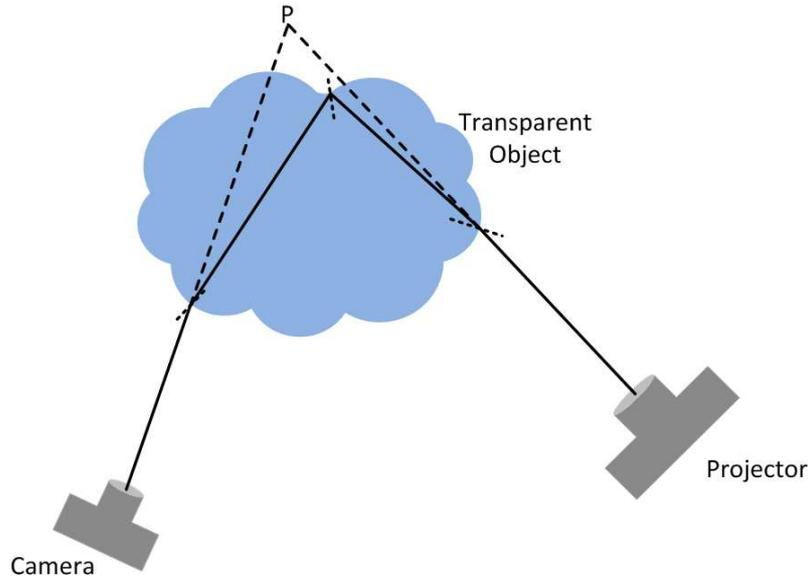
Figure 3.2: Points generated by triangulation may not exist. Other optical effects are not illustrated here.
