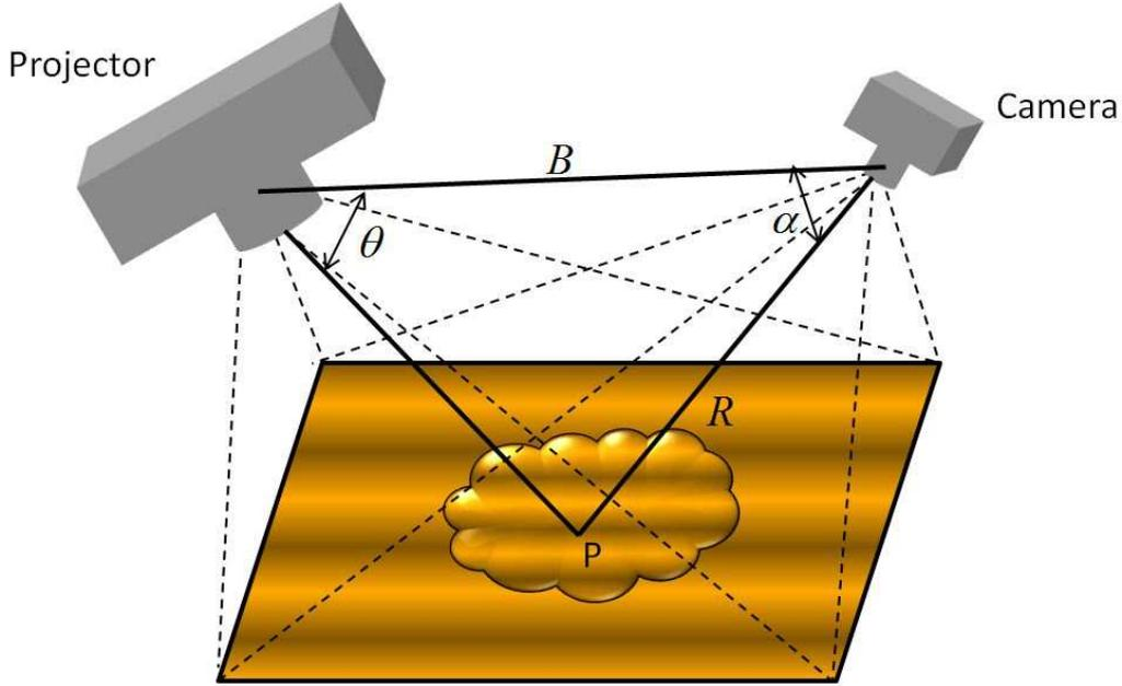
Figure 2.2: An illustration of structured light (redrawn based on [2]).
