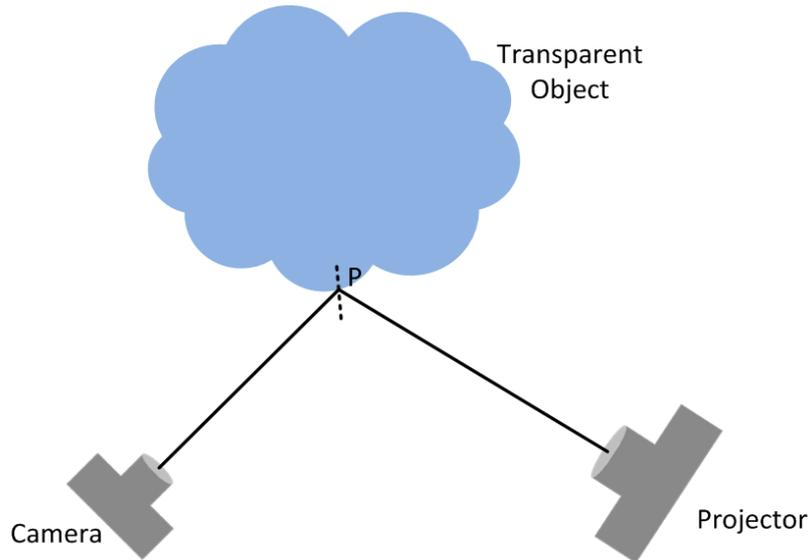
Figure 3.1: First-order reflection. Other optical effects are not illustrated here.
