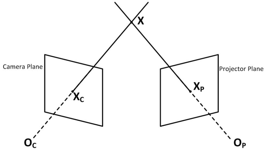
Figure 1.1: An illustration of triangulation.  $O_C$  is the camera center.  $O_P$  is the projector center.  $X_C$  and  $X_P$  are the corresponding points, respectively, on the camera plane and the projector plane.  $X$  is the intersection point on the surface of the object.
