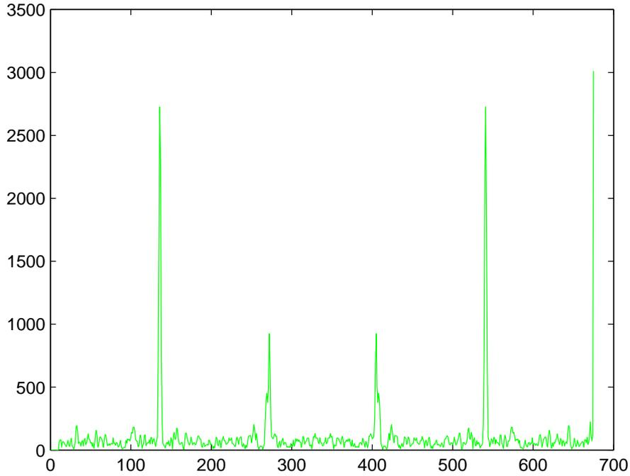
Figure 4.1: An example of frequency analysis for the trophy with multiple faces at pixel ( $i=432$ ,  $j=321$ ).
