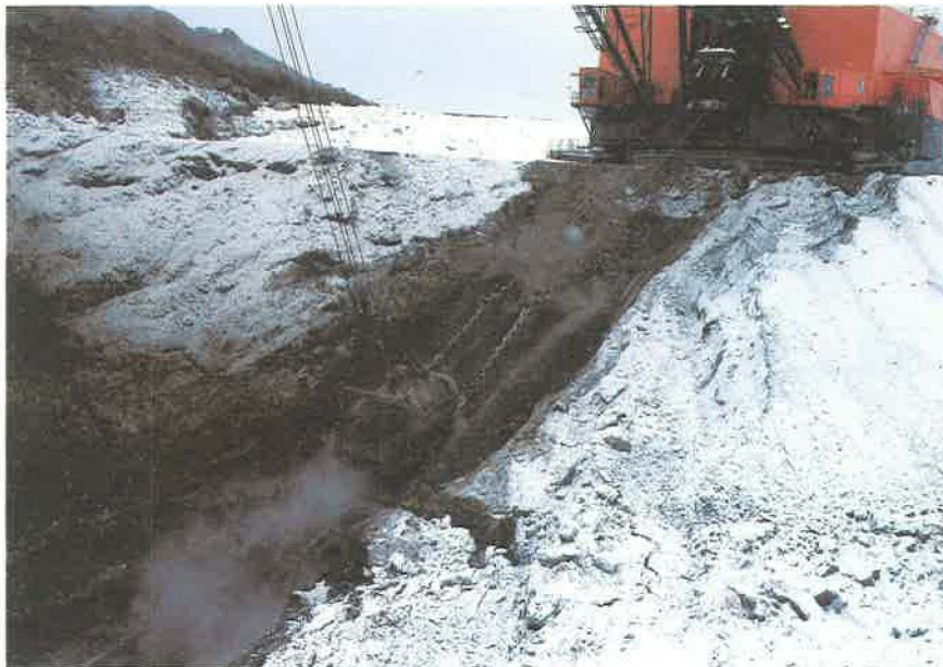
Figure 1.3.3-8 A dragline bucket being filled with oil sands by dragging along the working face.
