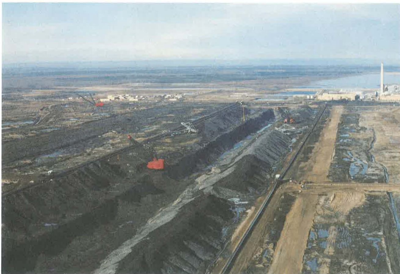
Figure 1.3.3-7 A single bench dragline mining and bucket wheel reclaimer loading belt conveyor at the Syncrude mine.
