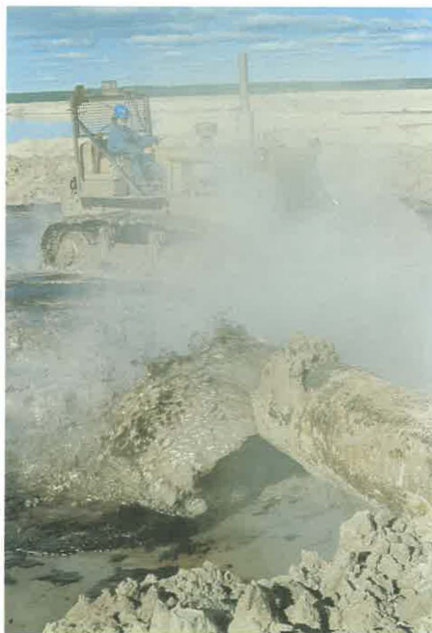
Figure 1.3.3-18 Tailings being dumped into cells from one of the tailings pipelines.
