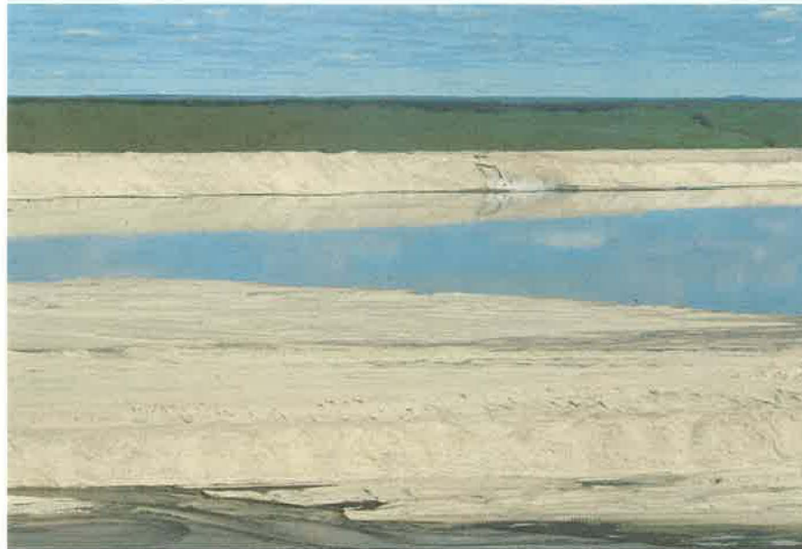
Figure 1.3.3-21 Tailings pond beach (in foreground); spigotting of slurry into pond (in background)
