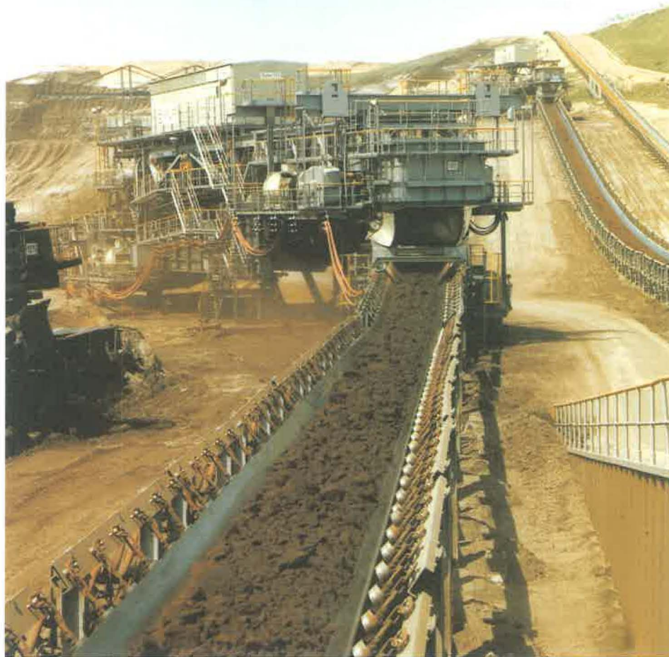
Figure 1.3.3-11 A conveyor transfer point with conveyor drive station.
