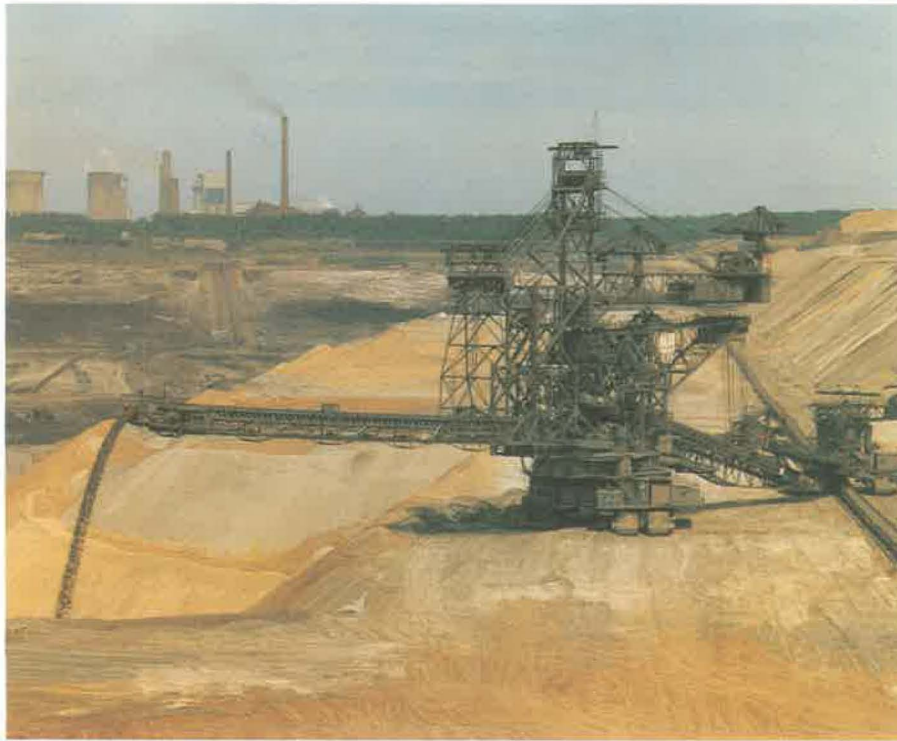
Figure 1.3.3-13 Spreader operating in low dump mode.
