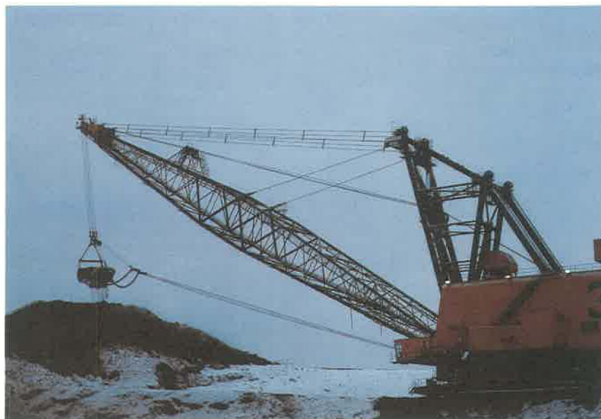
Figure 1.3.3-9 A dragline swinging into position to drop oil sands from bucket into a windrow.
