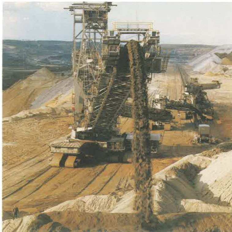
Figure 1.3.3-14 Spreader operating in high dump mode.
