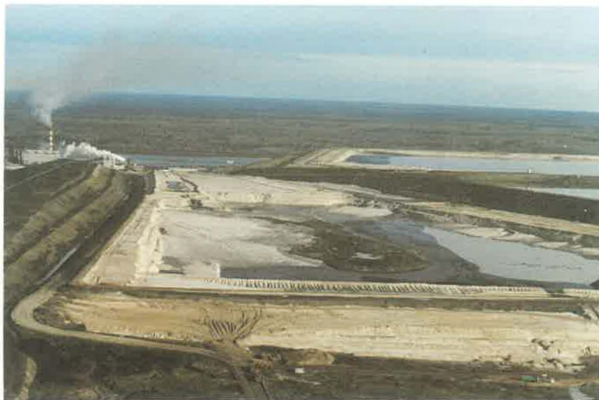
Figure 1.3.3-20 In-pit dyke construction at the G.C.O.S. mine will allow tailings to be back-filled into the empty pits.
