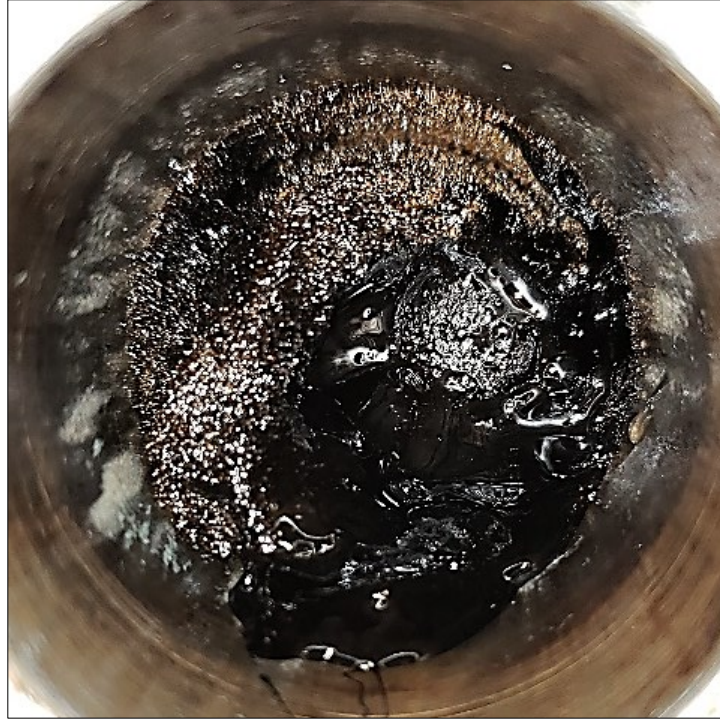
Figure 2.4 —Remaining heavy oil saturation at the injection port.
