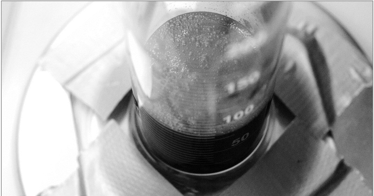
Figure 2.9 —Foamy oil collected at the production end.
