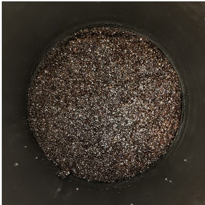
Figure 2.5 —Remaining heavy oil saturation at the production port.
