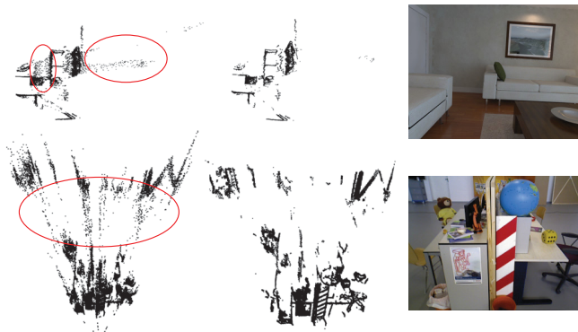
Figure 4.3: The proposed adaptive filter on semi-dense depth map. From left to right: (back-projected) semi-dense depth map from LSD-SLAM, filtered semi-dense depth map, and keyframe image.
