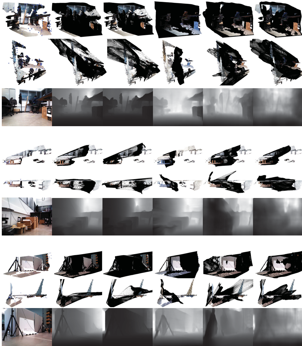
Figure 5.7: A qualitative comparison of the back-projected point clouds (shown in black) between (from left to right) ground truth depth with SVO map points (in blue), MiDaS v2.1, MiDaS v3.0, DiverseDepth, pre-trained Monodepth2, and our online adapted Monodepth2. From top to bottom: first and second viewpoint of the back-projected depth maps and the predicted depth maps by the aforementioned CNN models. Our proposed method’s overall online adapted depth prediction accuracy compares favourably with MiDaS and DiverseDepth, which have been trained on an extensive collection of datasets. The predicted depth maps are scaled to ground truth. Best viewed digitally.
