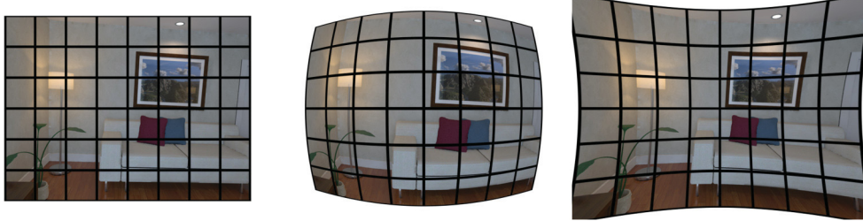
Figure 2.3: Examples of distorted images. From left to right: image with no distortion, image with barrel distortion and image with pincushion distortion. Image taken from the ICL-NUIM dataset [5].
