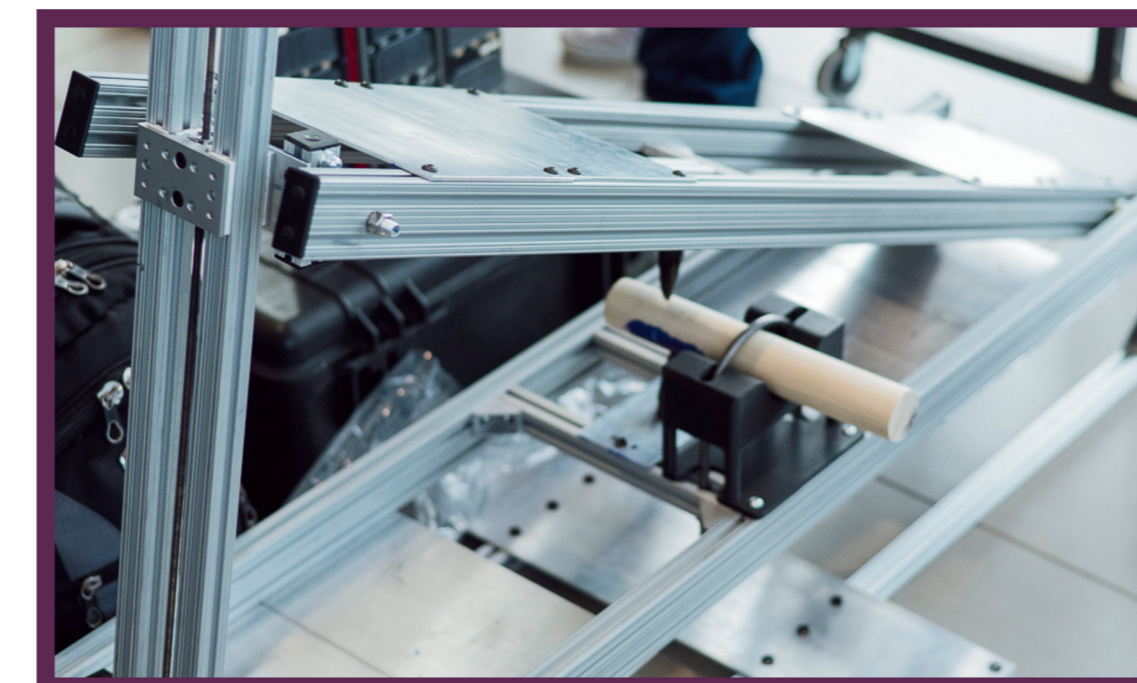
Figure 3, Photo of Mechanical biting rig ("Chomp-E") Photo by Taia Wyenberg-Henzler
