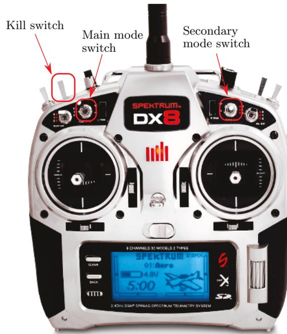
Figure 2.11: The spektrum DX8 radio transmitter.
