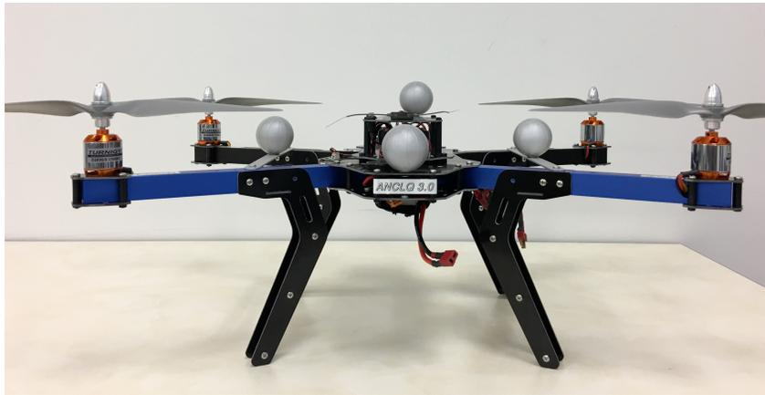
Figure 2.9: ANCL quadrotor version 3 (ANCLQ 3.0).
