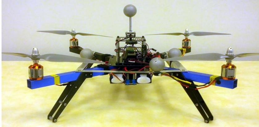
Figure 2.7: ANCL quadrotor version 1 (ANCLQ 1.0).
