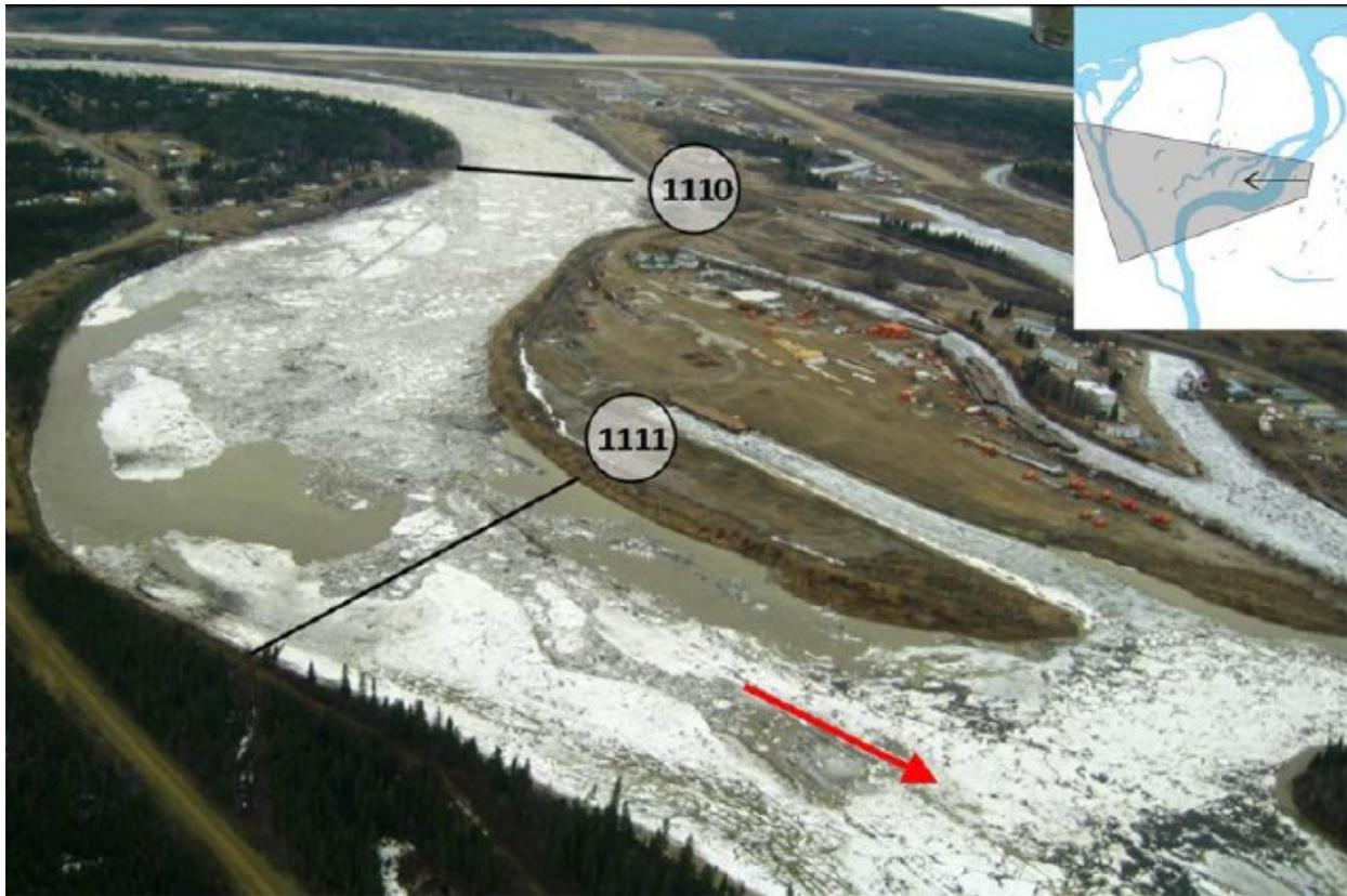
Figure 3.3 Example aerial photo of ice jam in the East Channel of the Hay River Delta taken May 5, 2008 (Brayall 2011).
