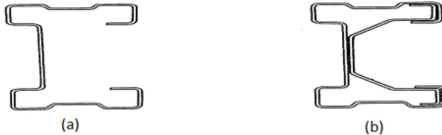
**Figure 18: Cross Sectional View of Light Weight Steel Gauge With and Without Torsion Sleeve (Boot, 1994)**
