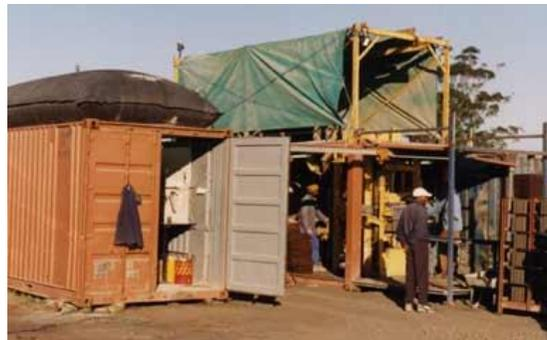
**Figure 4 - Sparlock mobile production container (Sparlock, 2010)**
