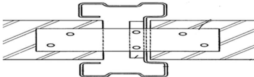
**Figure 19: Prefabricate Masonry Connected to a Fence Post by Means of Steel Plate (Boot, 1994)**
