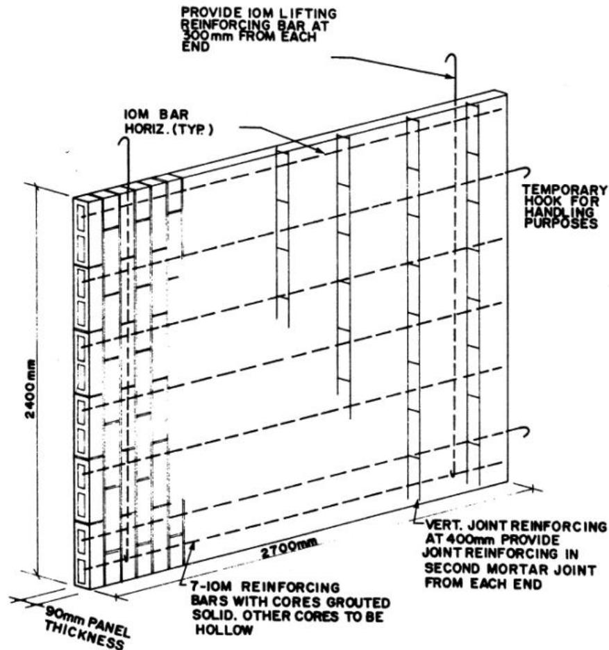
Figure 12: Reinforcing Detail for Masonry Panel (Adapted from Hatzinikolas & Pacholok)
