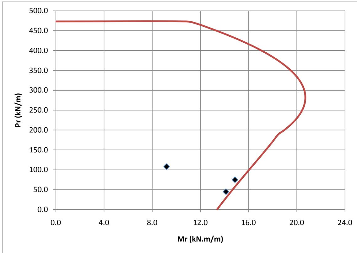
**Fig.4.3 Interaction diagram for AAC wall in Example No.2**
