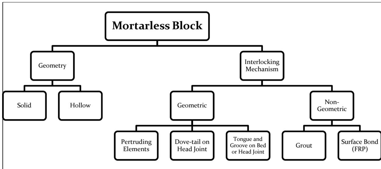
**Figure 1 - Classification of Block Mortarless Masonry**
