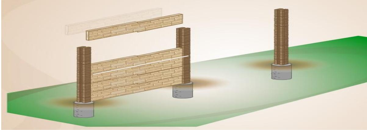
**Figure 15: Installation of Prefabricated Panels Between Pilasters (Artisan, 2010)**
