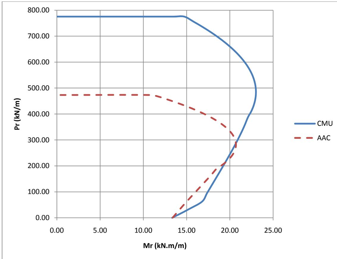
**Fig.4.6 comparison of Interaction diagrams of CMU and AAC walls reinforced with 20M@600**
