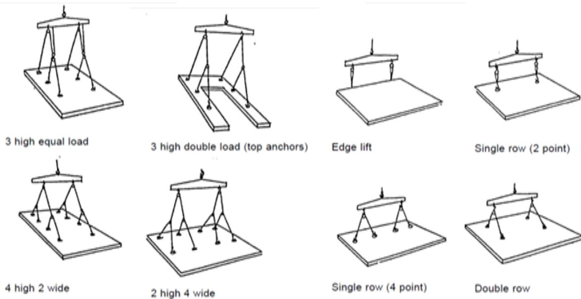
**Figure 9: Common Methods of Lifting Prefabricated Panels (OSHS,2002)**
