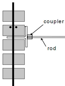
**Figure 22: Lateral Connection for Prefabricated Panels (Tawresey, 2004)**
