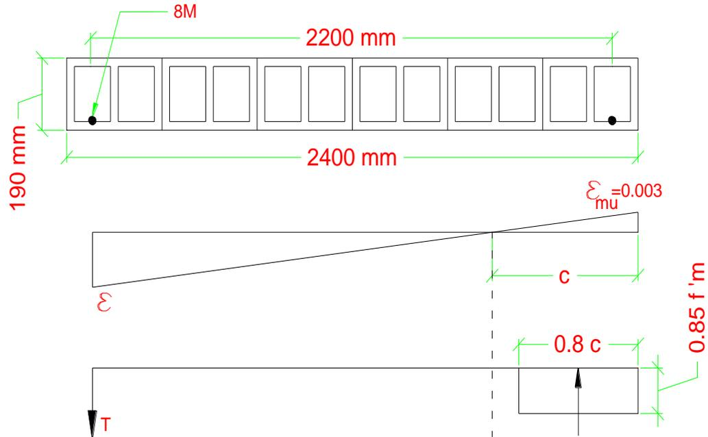
**Figure (8): Wall Section, strain distribution and stress distribution**
