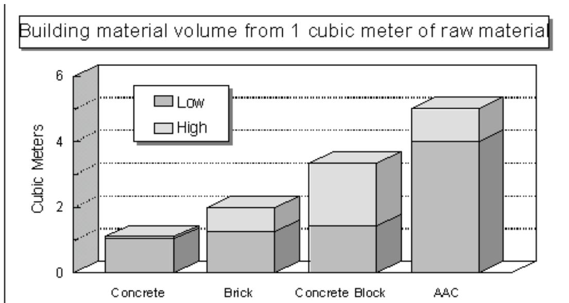
**Fig. 2.2: Comparison of different building materials by volume** <sup>(2.7)</sup>
