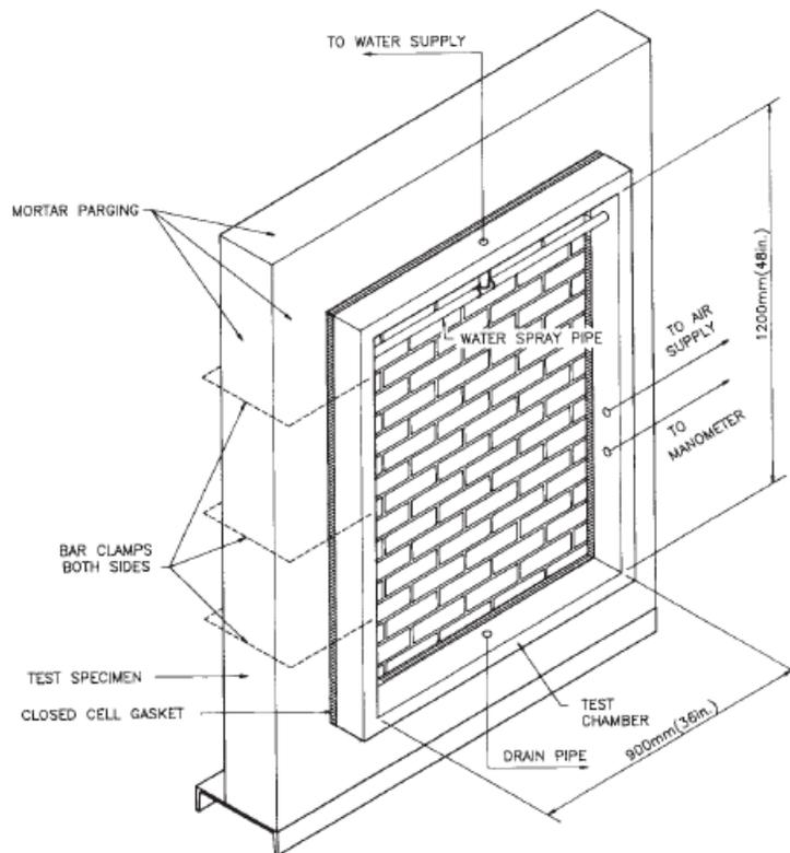
**Figure 9 - Isometric projection of testing chamber (ASTM E514-04)**
