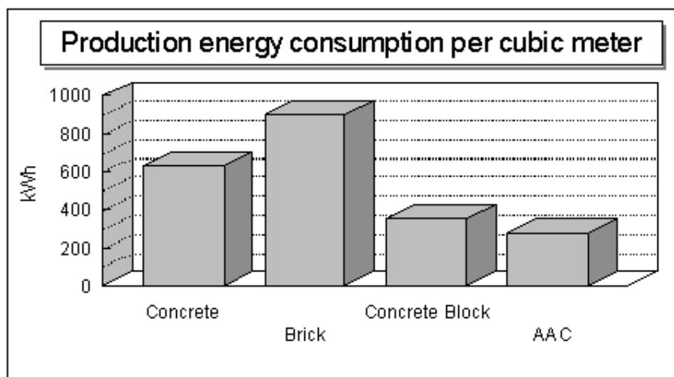
**Fig. 2.3: Comparison of production energy consumption for different type of building materials** <sup>(2.7)</sup>
