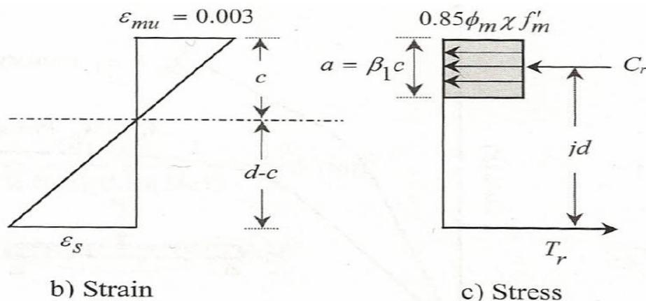
**Figure 10: Stress and Strain Distribution Along the Thickness of the Panel (Korany & Hatzinikolas, 2005)**
