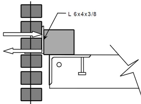
**Figure 21: Gravity Connection Illustrating Forces Perpendicular to Plane of Wall (Tawresey, 2004)**
