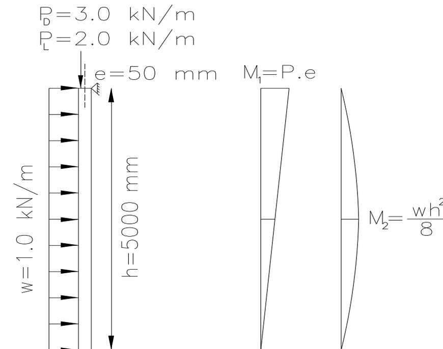
**Fig.4.1 AAC masonry wall in example No.1**
