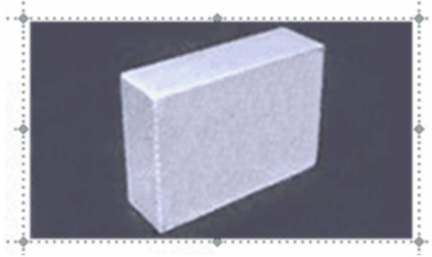
**Fig. 5.2 AAC Semi Jumbo Block** <sup>(3.6)</sup>
