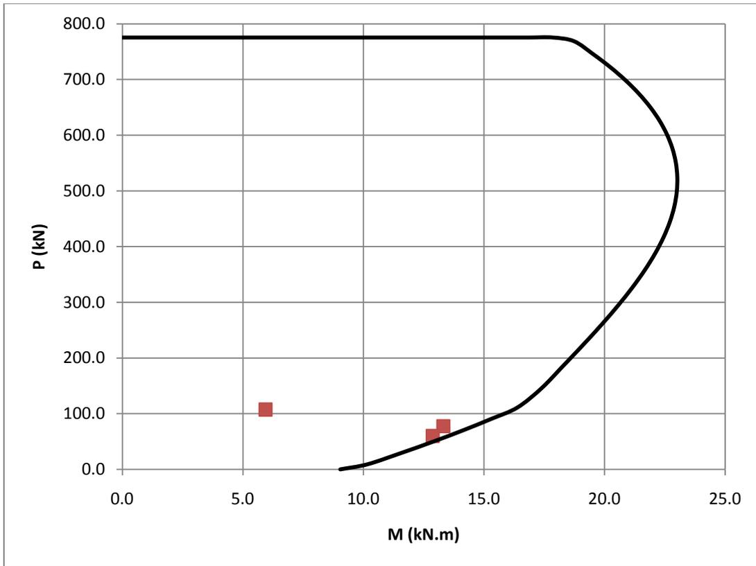
**Fig.4.5 Interaction diagram for CMU wall with 15M@600 for the second example**
