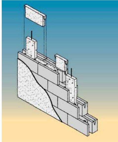
**Figure 2 - Cutaway of an IMSI Wall (VanderWerf, 1999)**
