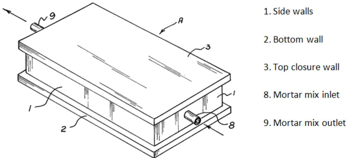
**Figure 5: Forming Box for a Prefabricated Masonry Wall (Brandt, 1972)**
