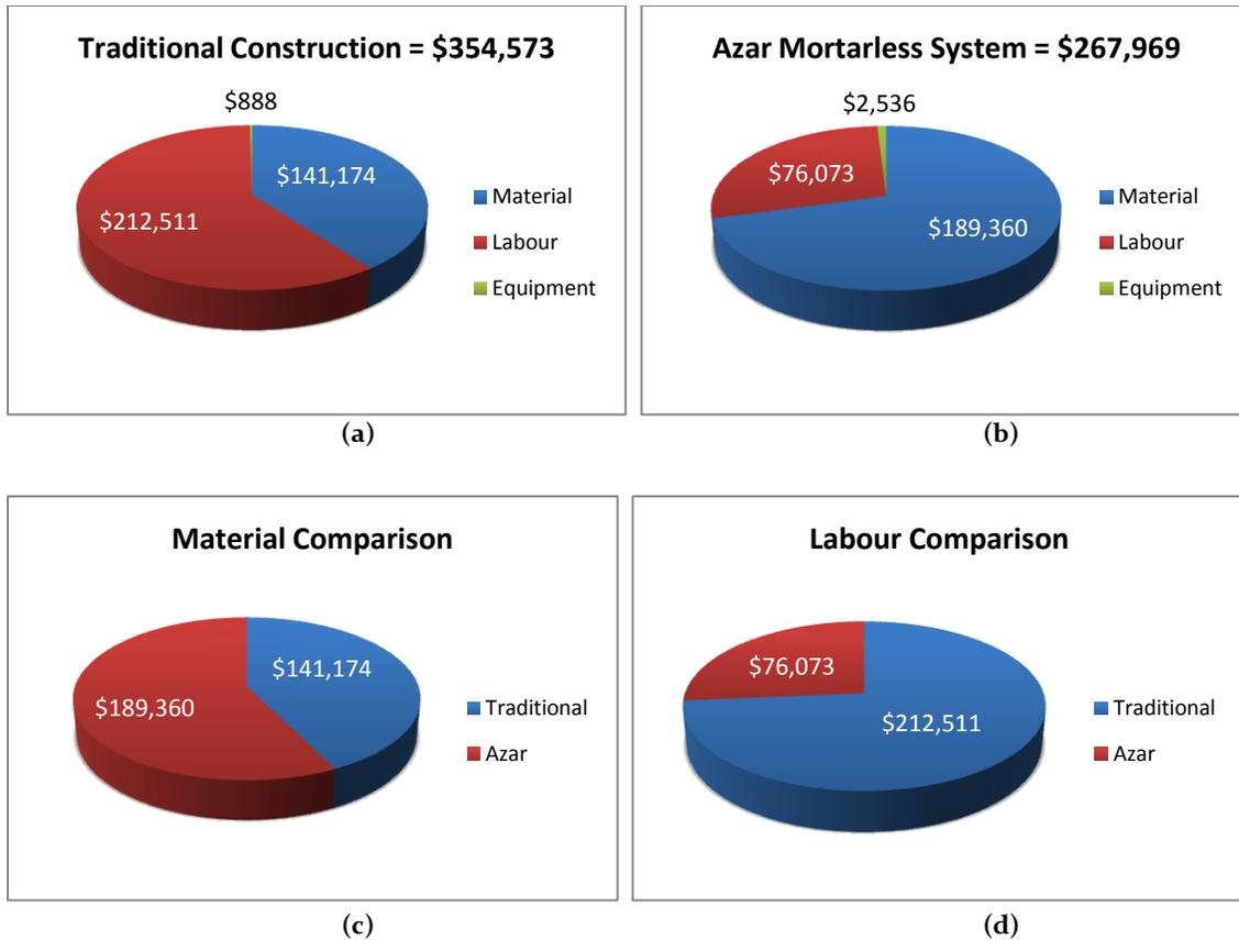
**Figure 5 – Construction costs associated with traditional and Azar mortarless construction**
