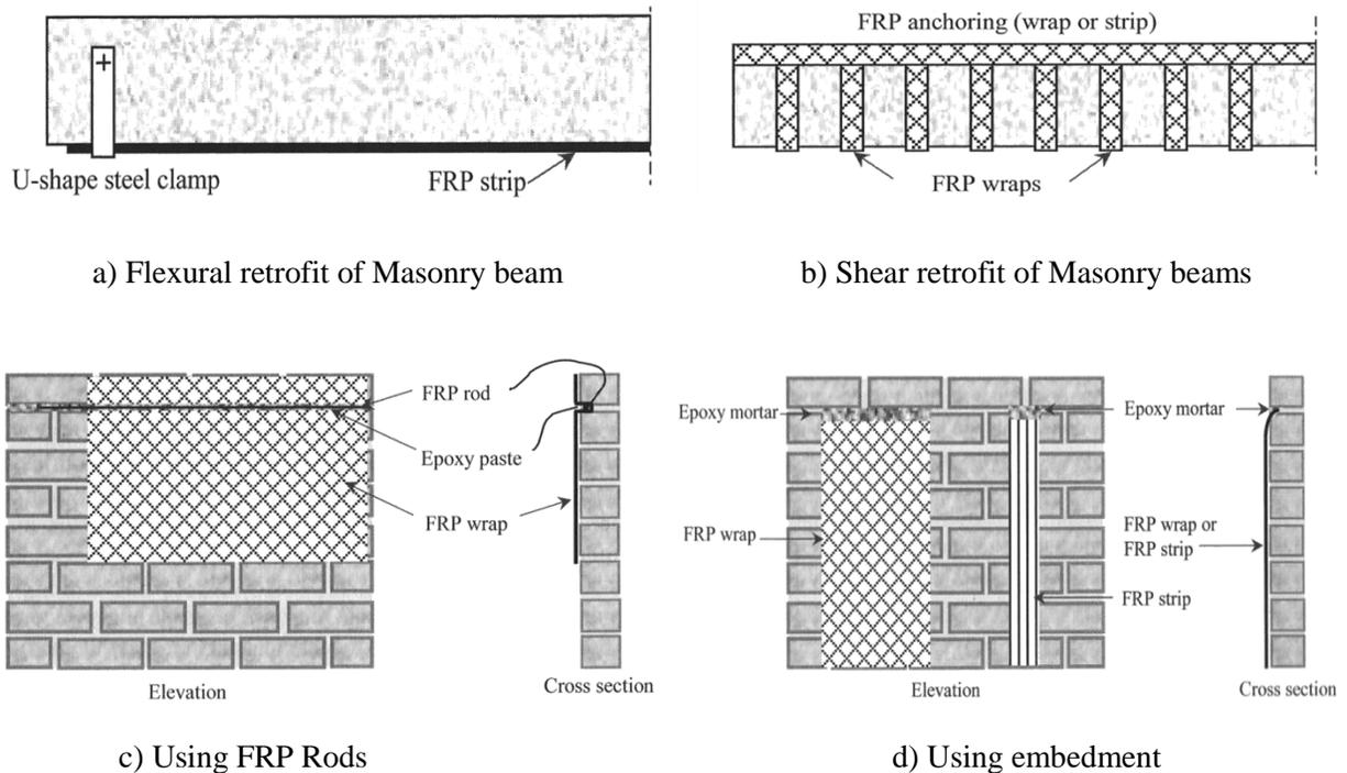
**Figure (3) Anchorage system for external FRP Reinforcement. (Hatzinikolas and Korany, 2005)**
