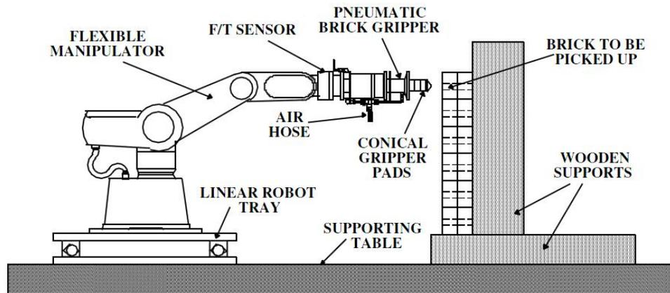
**Figure 7: Robotic Masonry Arm Used to Stack and Move Brick (Rihani, 2006)**
