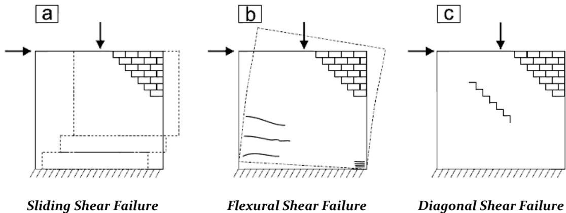
**Figure 8 - Types of masonry wall failures induced by in-plane lateral loads (Marzahn, 1998)**
