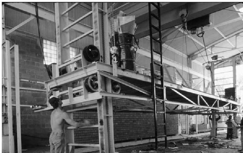
**Figure 2: Automated Scaffolding at the Vet-O-Vitz Manufacturing Plant (BIA, 2001)**
