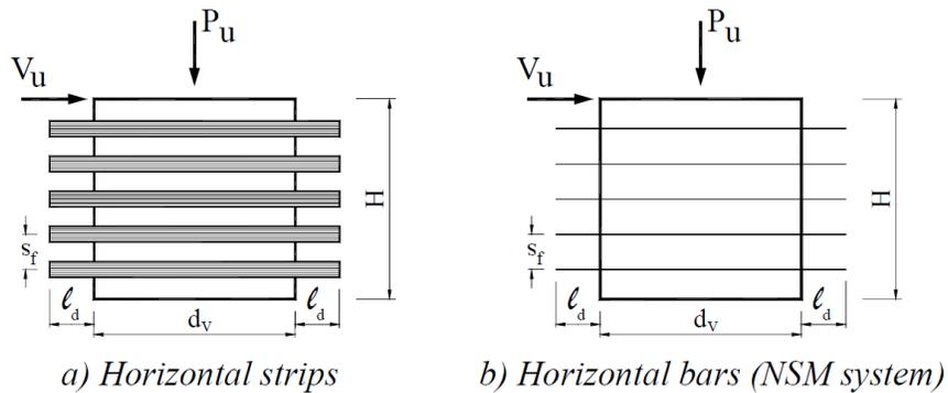
**Figure (4): FRP strengthening for shear controlled walls**
