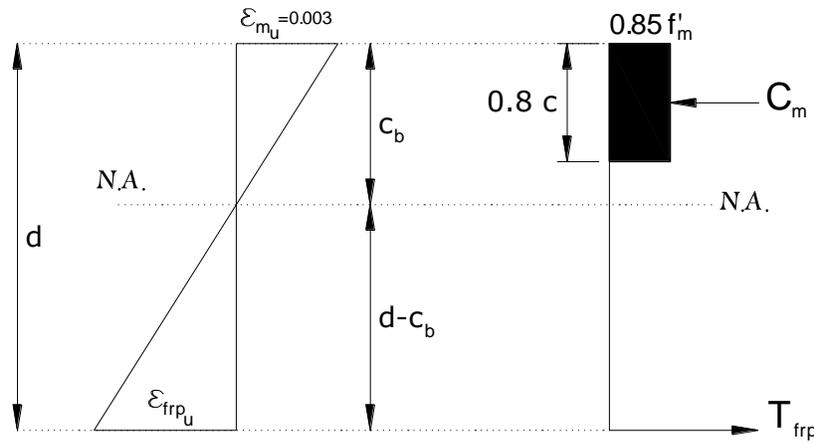
**Figure (6): Strain distribution and stress distribution on the wall**
