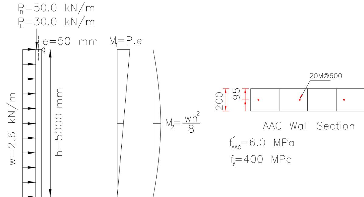
Fig.4.2 AAC masonry wall in example No.2
