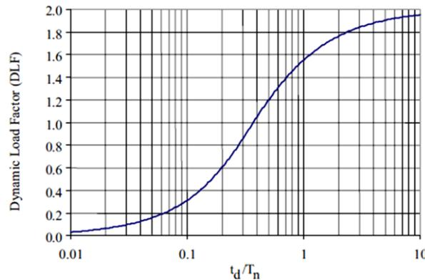
**Figure (9): Dynamic Load Factor for the Equivalent Triangular Pulse (Tan and Patoary (2009))**
