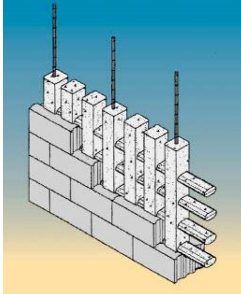
**Figure 3 – Cutaway of a Faswall wall (Adapted from VanderWerf, 1999)**
