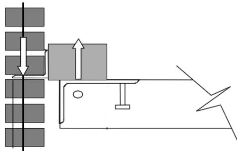
**Figure 20: Gravity Connection Illustrating Vertical Forces (Tawresey, 2004)**
