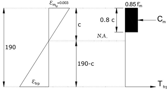
**Figure (7): Strain and stress distribution on the wall**
