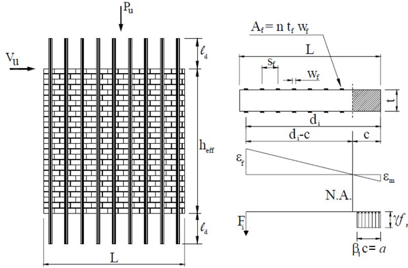
**Figure (5): FRP strengthening for flexural**
