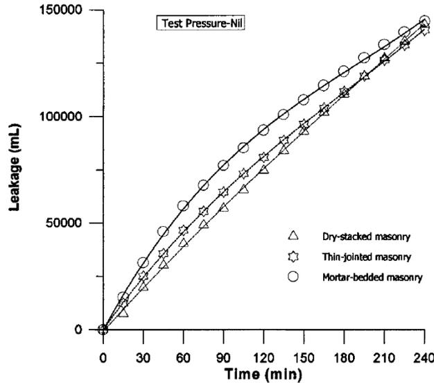
**Figure 11 - Variation in leakage – no surface finish (Anand and Ramamurthy 2001)**
