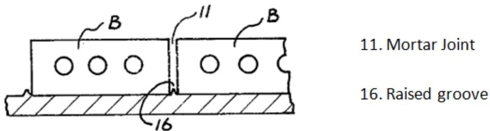
**Figure 613: Illustration of Raised Grooves to Align Brick Inside Forming Box (Brandt, 1972)**
