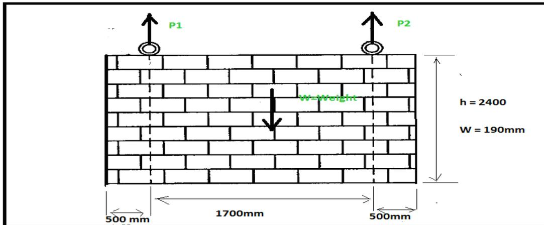
**Figure 11: Hoisting Loads Acting on the Masonry Panel (Sutter, 2001)**
