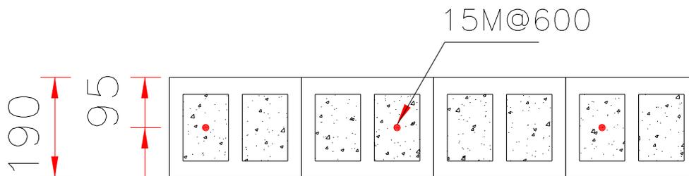
**Fig.4.4 Reinforcement of CMU wall for the second example**
