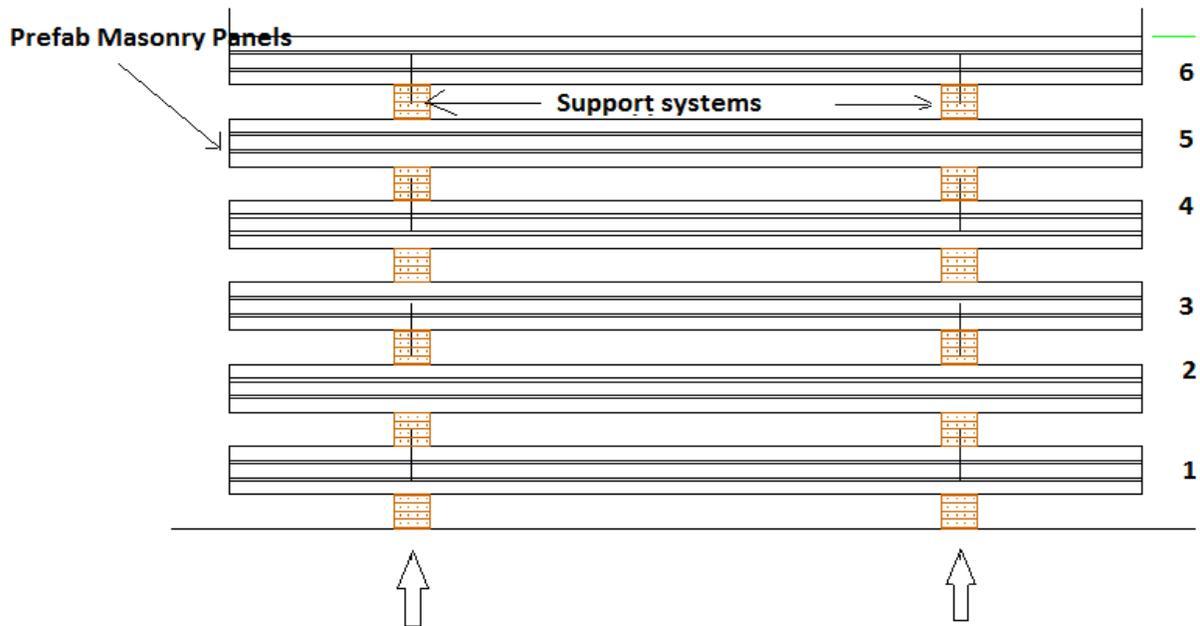
Figure 13: Stacking of Prefabricated Masonry Panels (Adapted from ACP, 2002)
