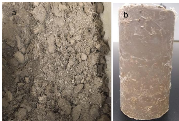
Figure 1: Fiber-reinforced soil adopted for testing a) Soil lot; b) Fiber-reinforced soil sample
