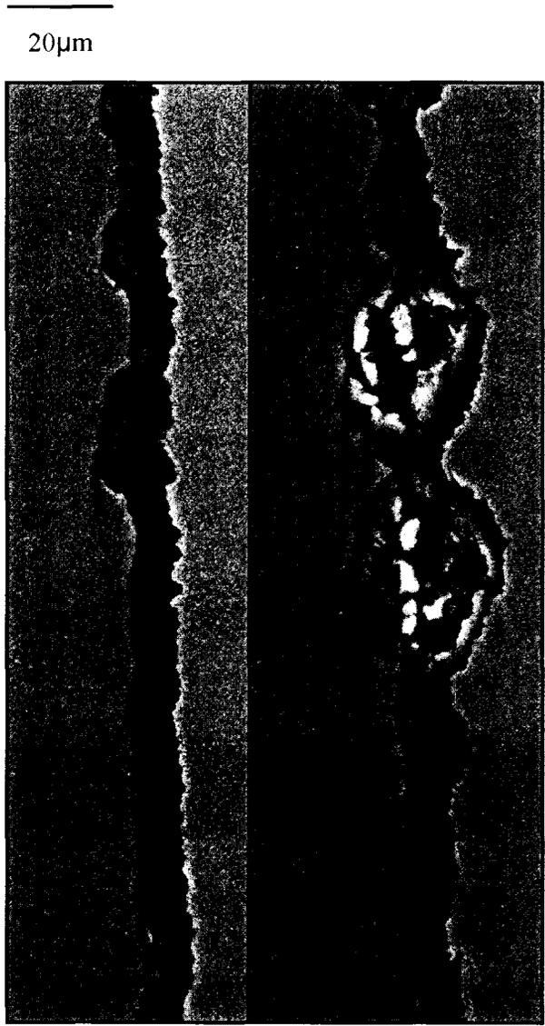
Figure 4-21. Two Distinct Regions of the Oxide Scale on the 430 Thin As-Is Specimen.
