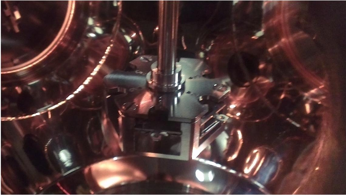
Figure 2.3: Tips and Samples are stored in this carousel by sliding them in to holding tabs.
