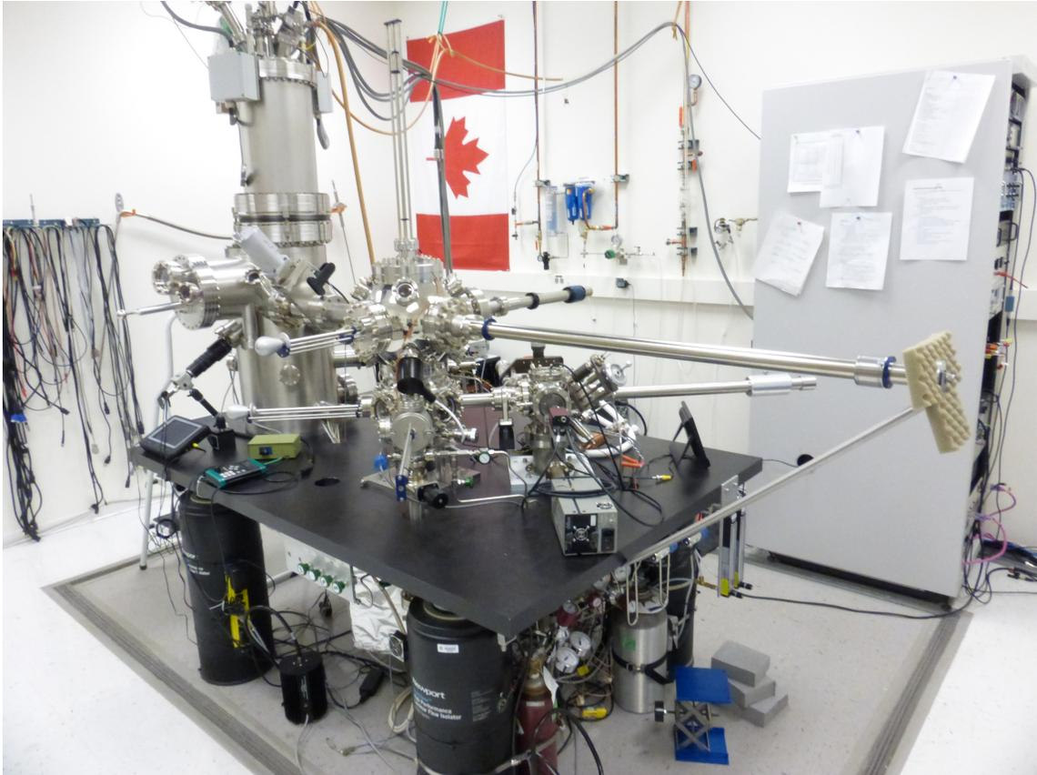
Figure 2.1: Omicron STM/AFM
