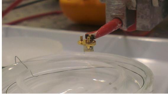
Figure 2.17: qPlus sensor mounted in the fine control motor above the NaOH etching solution
