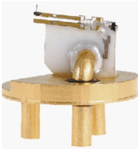
Figure 2.12: A commercially ordered qPlus sensor. The quartz tuning fork has one prong glued to a ceramic stage, while the other has a conductive metal tip glued to the conductive gold patterning on the side.
