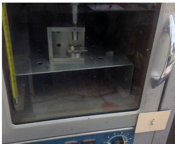
Figure 2.14: Detachable tip placement device with epoxied tip curing in the oven.
