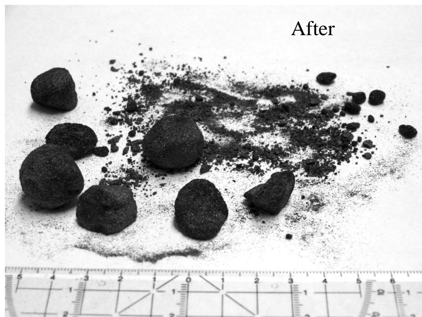
Figure 4.15: Photos of 15mm and 10% AVR concentration agglomerates before and after reaction
