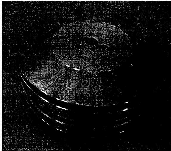
Figure 4.4. Magnet rotor ( \phi 8'' \times 2'' ) composed of (from top to bottom) yoke plane, magnet holder, gap (8 mm), magnet holder and yoke plane.
