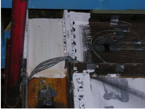
(j) North top connection, Cycle 20-Push
