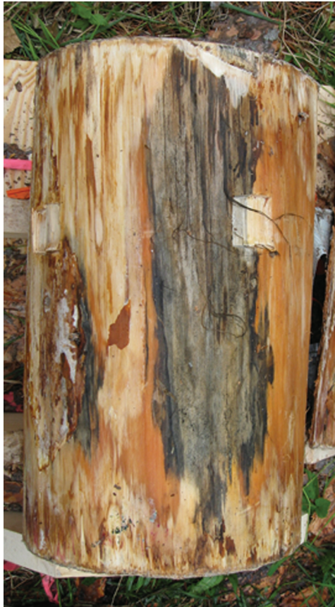
Figure 4.1: An example of the extent of fungal spread at the end of May for fungal symbionts of the mountain pine beetle. The fungi visible in the centre and on the left were inoculated into the waxed bolt the previous fall (September 2009).
