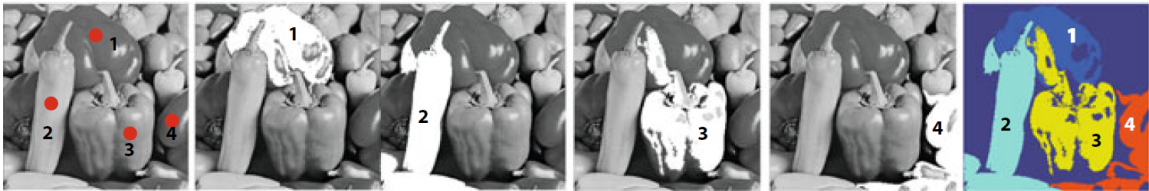
Figure 2.12: From left to right: the original image with four selected seeds, the extraction of four regions based on thresholds T = 0.05 to 0.2 , and the final segmentation result [11].
