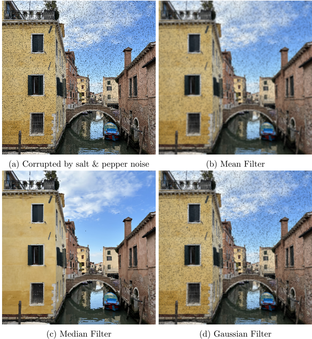
Figure 2.3: Examples of filtering operations applied to an image corrupted by salt & pepper noise.
