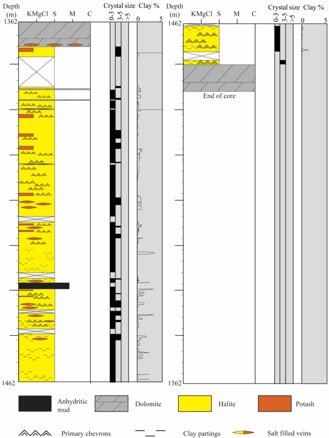
Figure 5 Core log of Well #1 depicting lithology, sedimentary features, and clay %
