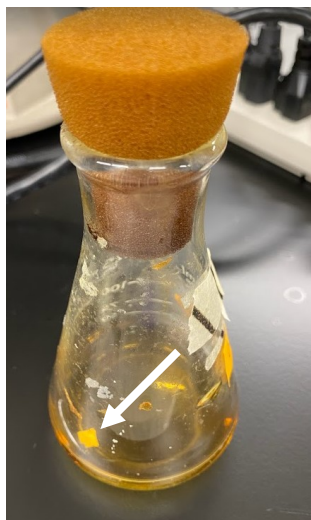
Figure 4.15. Sterilized flask with bacterial culture and wafer being tested.
