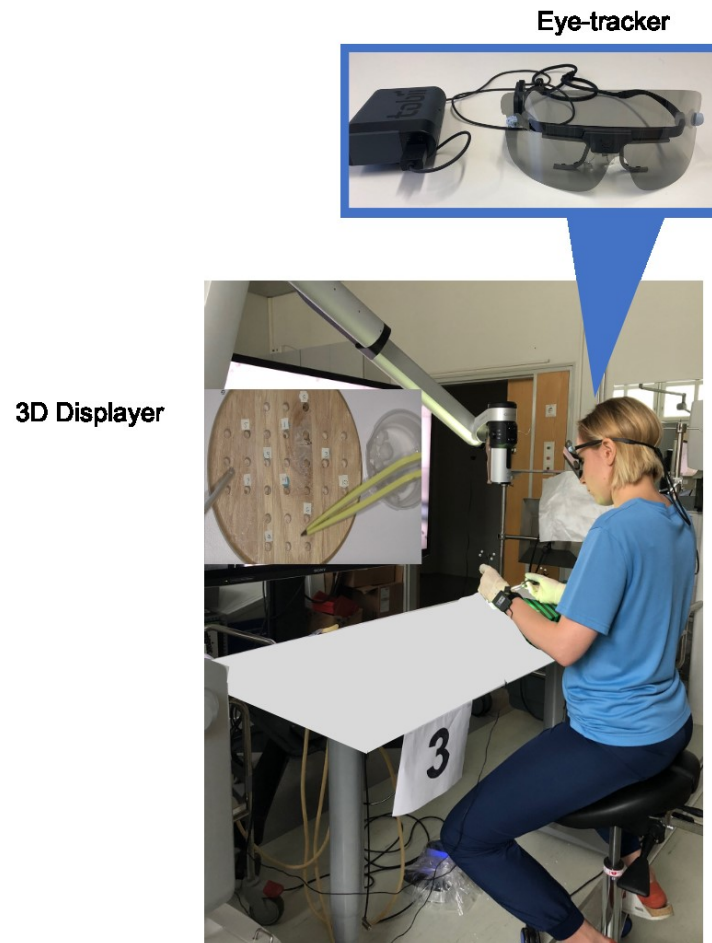
Figure 3.2 Display of the surgical task, the Olympus ORBEYE – 4K 3d surgical microscope and the Tobii Pro 2 Glasses wearable eye tracker with the CFV-E30D 3D EYE Shield
