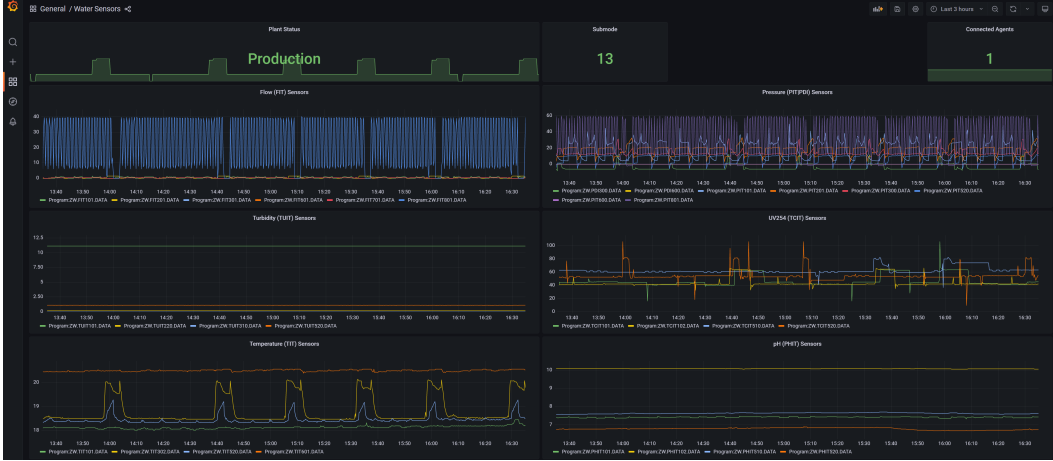
Figure 3.8: The Grafana dashboard shows real-time information about the pilot, including current operation mode, number of agents connected and important sensory readings.
