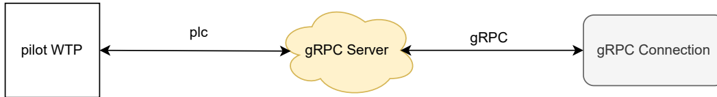
Figure 3.5: Block diagram of the connection to the pilot WTP. This implementation of Connection creates a secure duplex channel to the gRPC server, which runs on a high-performance computer physically connected to the PLC controller of the pilot WTP.
