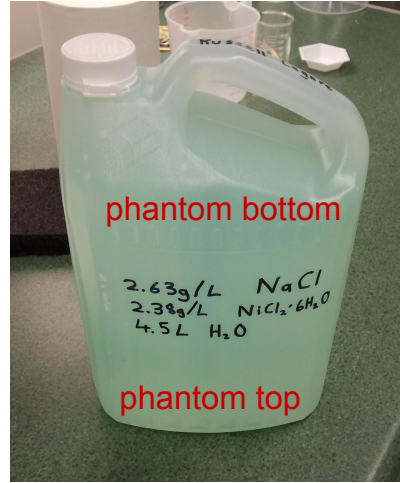
Figure 22: Phase Shift Phantom for phase shifting experiments. The top of the phantom refers to the portion which is oriented towards +Z along the magnet bore, and the bottom is towards -Z.
