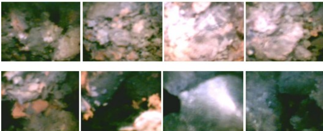
Figure 3-37 Experiment 5: post burn images from all the available holes captured by mini inspection camera.
