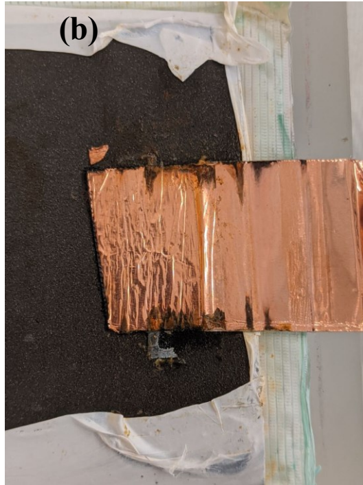
Figure 3.10 Oxides on the surface of the (a) nichrome/alumina layer and (b) Copper tape
