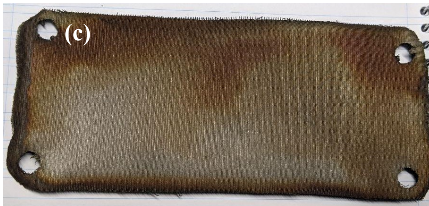
Figure 2.5 Oxidation of the substrates when (a) No cooling system was used, (b) Direct exposure to the cooling system, and (c) Indirect exposure to the cooling system (aluminum foil attached)
