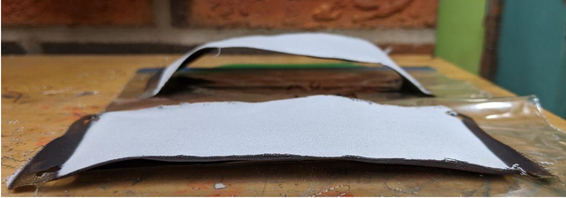
Figure 2.4 Effect of spray parameters on the thermally induced deformation of the substrate
