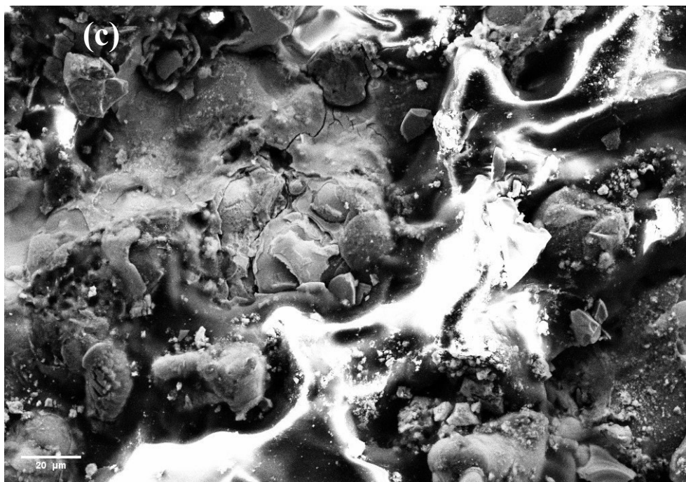
Figure 3.11 Top view images of the nichrome/alumina layer after being used in the MD process (a) 40x, (b) 40x, and (c) 500x
