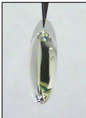
Figure 2.5: HAMA gel adhered to glass coverslip with PLL coating to allow gel manipulation and stability during media changes
