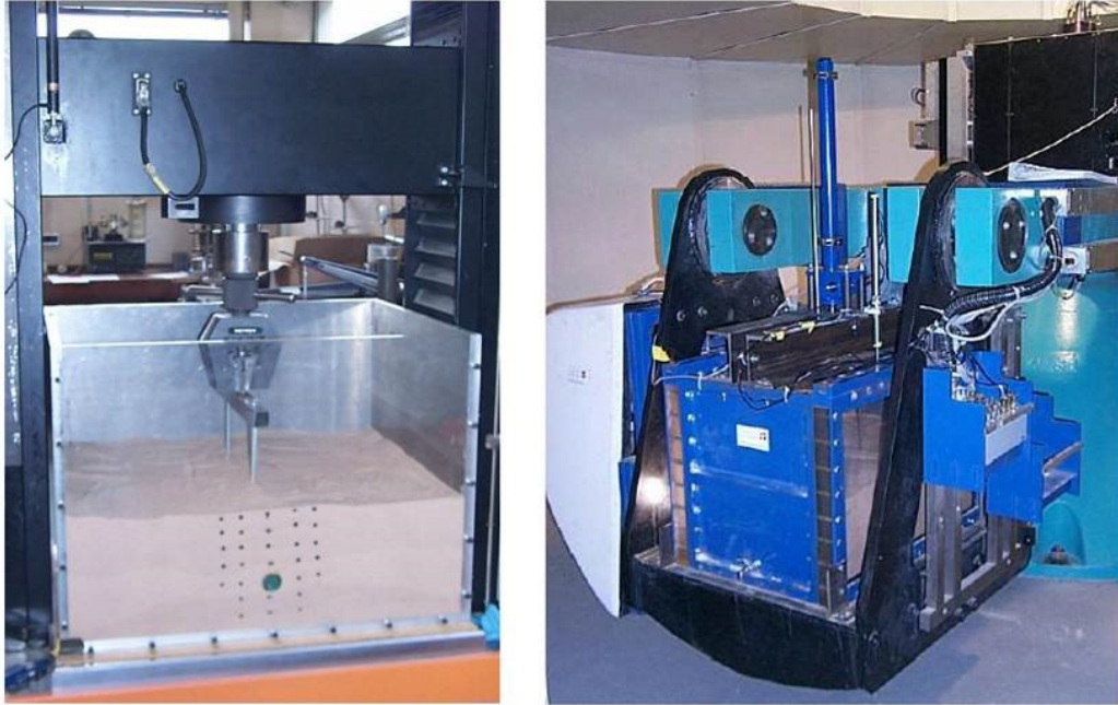
Figure 2-18 Laboratory test apparatus (left) and centrifuge model package (right) (Bransby, 2002).
