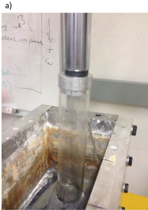
Figure 3-15 a) Shelby tube being pushed down into the kaolin block by hydraulic ram and b) five Shelby tubes pushed all the way down to the bottom of kaolin block.
