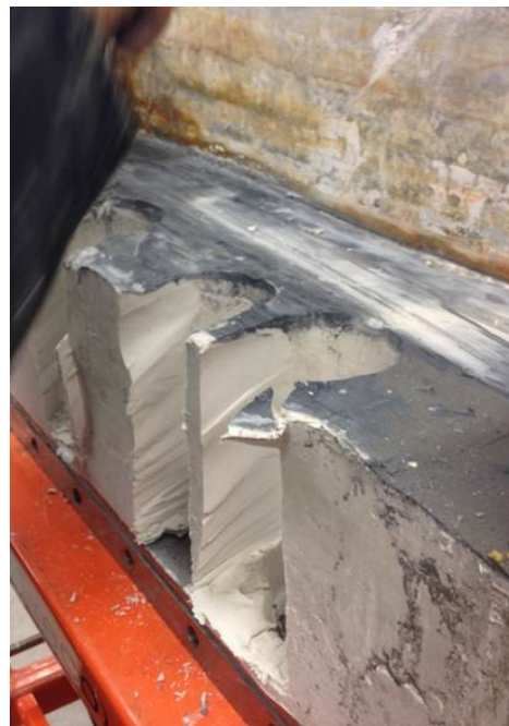
Figure 3-15 a) Shelby tube being pushed down into the kaolin block by hydraulic ram and b) five Shelby tubes pushed all the way down to the bottom of kaolin block.
