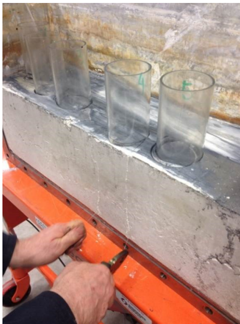
Figure 3-16 Cutting the Shelby tube out of the kaolin block.
