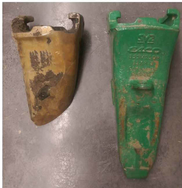
Figure 6-29: Tooth after 18 Hours of Service (Left) and New Tooth (Right)
