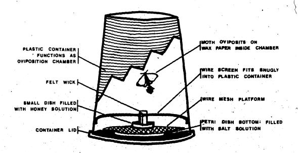
Figure IV-1. Diagram of oviposition chamber used for experiments, cut away to expose the interior.
