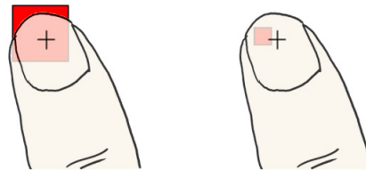
Figure 1.2: Finger input is restricted by the size of the target. The target should be bigger than the footprint of the fingertip (left). Otherwise, the target can be occluded, thus being difficult to select (right). The crosshair indicates the location of the touch.
