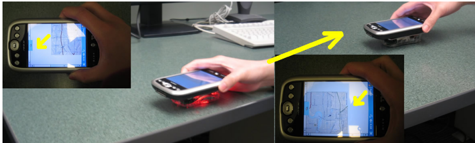
Figure 4.6: Panning a map by moving the device against a table. The device was moved in the NE direction, and the map was panned in the SW direction.
