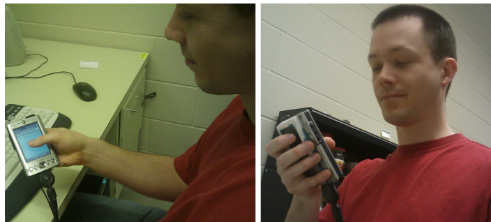
Figure 4.7: In the experiment, we asked participants to sit in a chair, and perform the target selection task using one hand. The touchpad on the back is operated using the index finger.
