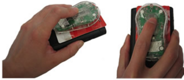
Figure 4.1: With LucidCursor, users can move the index fingertip over the optical sensor to control the movement of a cursor.
