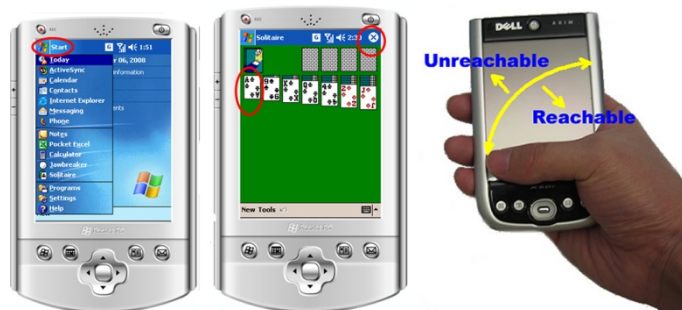
Figure 4.5: It is common that targets to be selected are located in places that are difficult to reach by the thumb (right).
