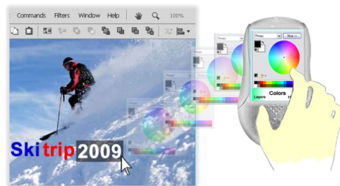
Figure 3.3: LensMouse shows the floating color panel window of a drawing application. This reduces window management and minimizes on-screen occlusion.
