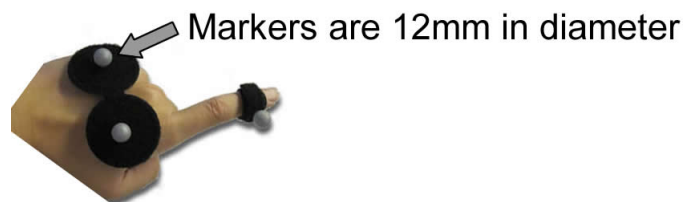
Figure 6.7: Reflective marker placement.
