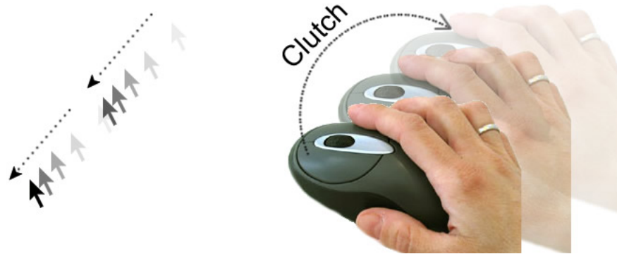
Figure 1.1: Illustration of mouse clatching. The straight, dashed arrow lines indicate the movement of the cursor every time the user clutches the mouse.
