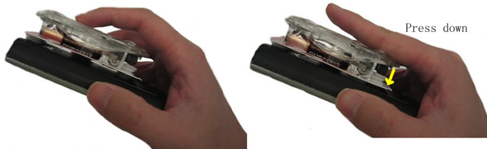
Figure 4.4: The user navigates the cursor to the target location (left). Releases the index fingertip, and clicks the mouse button by pressing on the corner of the mouse, using the base of the index finger (right).
