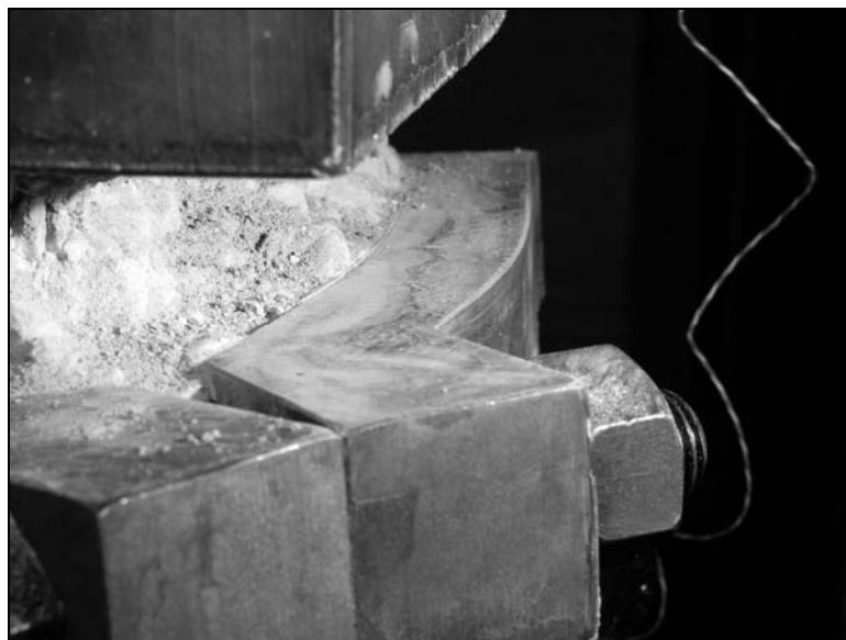
Figure 4.13: Deformed Shape of Collar During Loading
