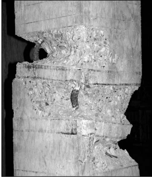
Figure 4.16: Specimen CE03 - Buckling of Longitudinal Reinforcing
