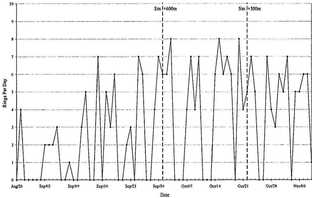
Figure 4-11 Rings built per day during construction of Southbound LRT Tunnel (2004).
