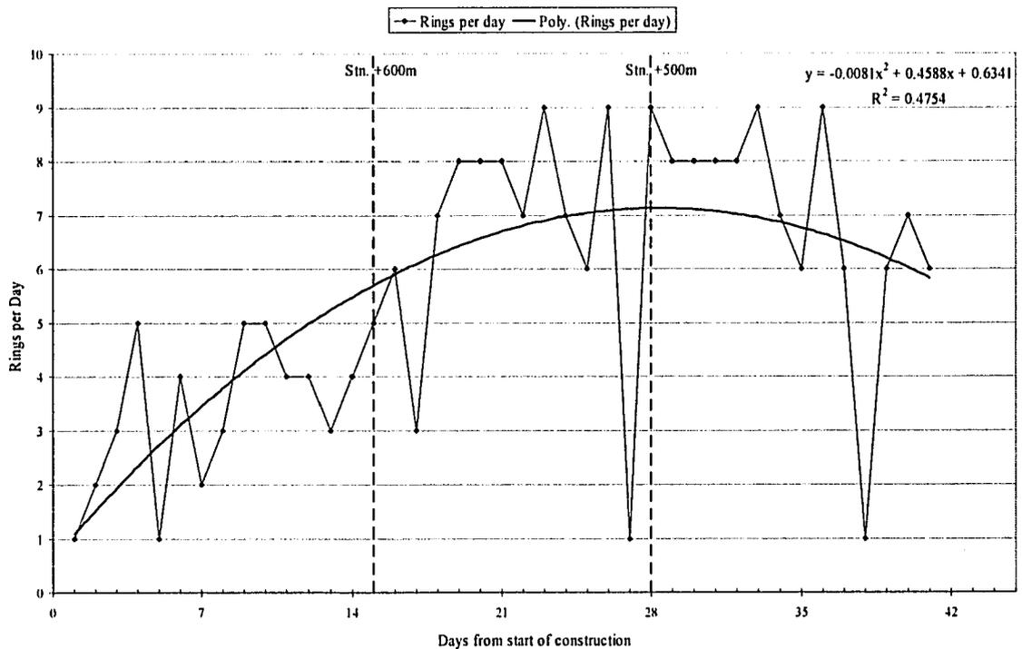
Figure 4-14 Rings built per day during construction of Northbound LRT Tunnel (2005).
