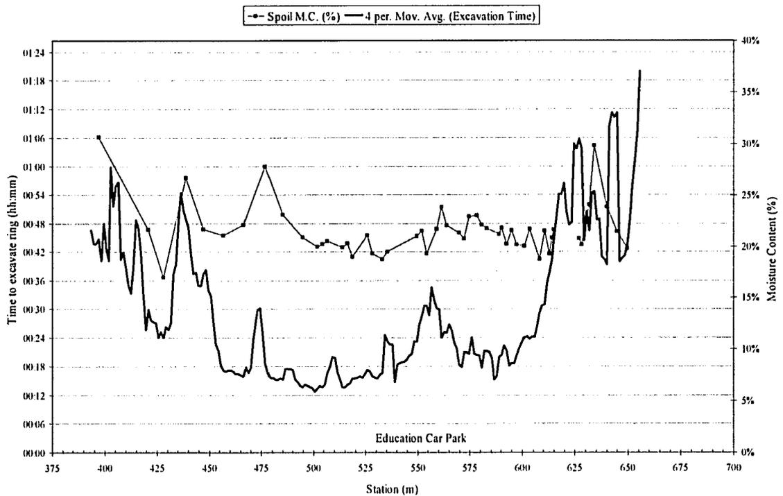
Figure 5-10 Correlation between process upsets as shown by TBM spoil moisture content and average mine times during Northbound construction.
