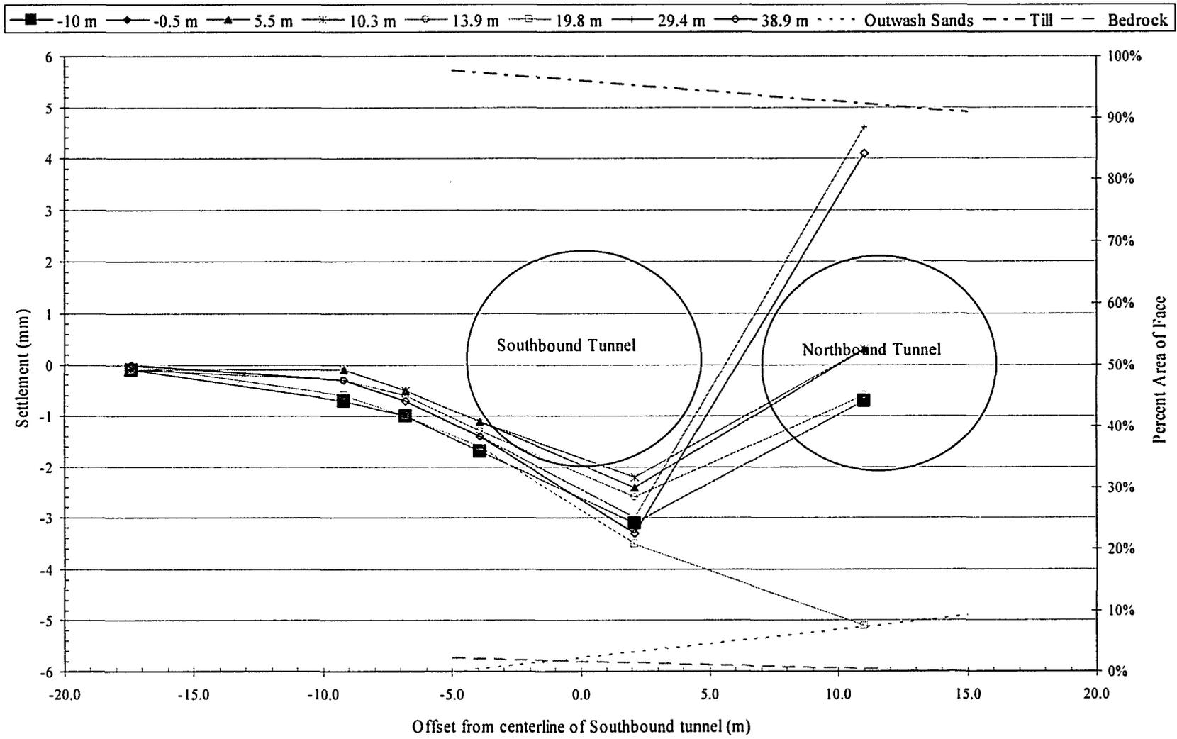
Figure H-6 Observed deep settlement at Array B during construction of Northbound Tunnel.
