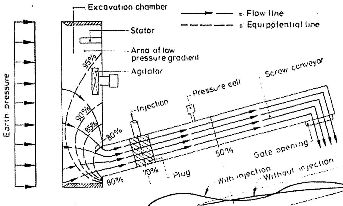
Figure 2-2 Generalised pressure drop in EPB-TBM machine from the face through the screw conveyor (Maidl et al., 1996.)
