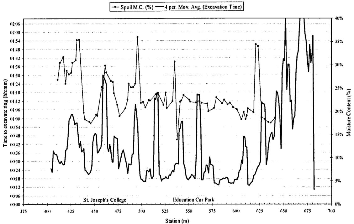
Figure 5-9 Correlation between process upsets as shown by TBM spoil moisture content and average mine times during Southbound construction.
