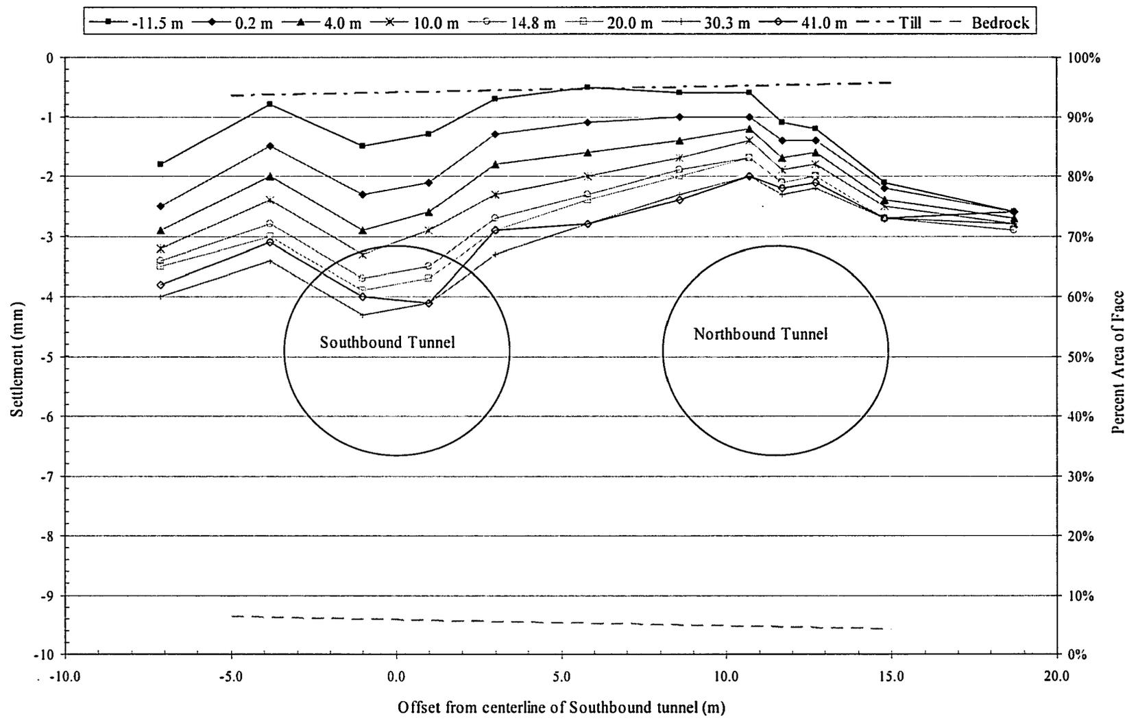
Figure 4-47 Observed shallow settlement at Array A during construction of Southbound Tunnel.
