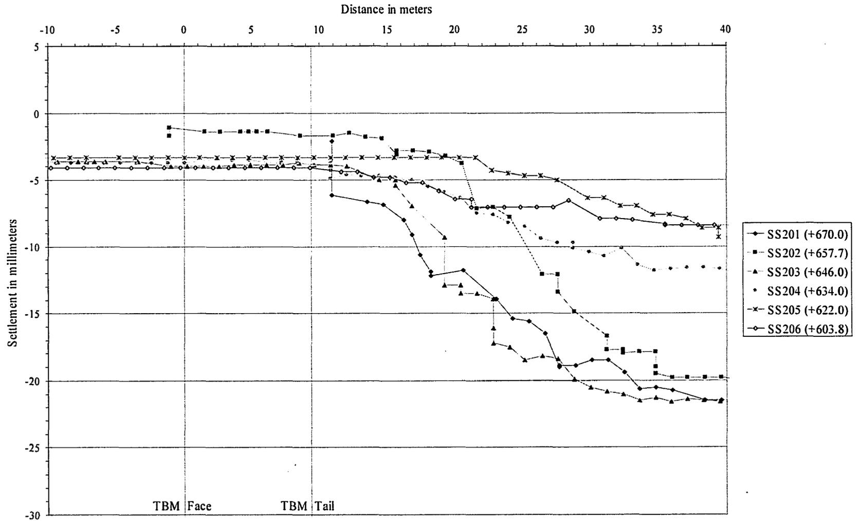
Figure 4-31 Observed shallow settlements during construction of Northbound Tunnel with proximity to TBM face, from Portal to Education Car Park.
