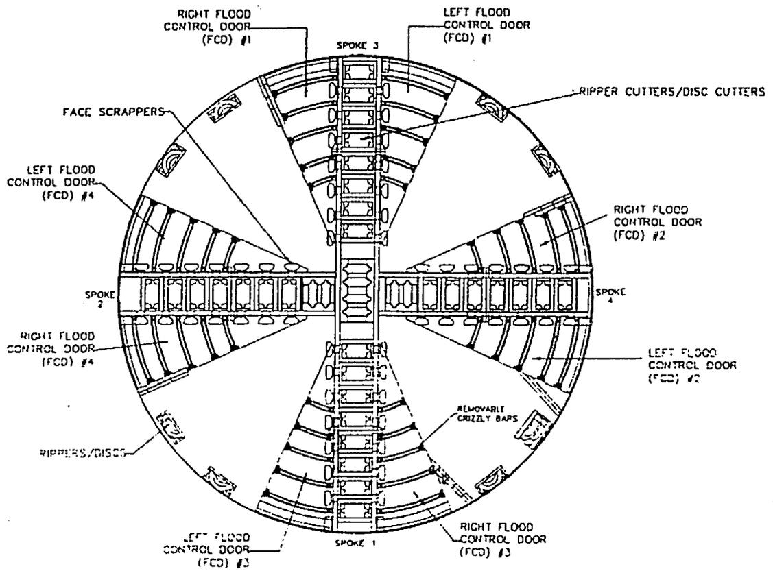
Figure 2-9 Cutting Head of EPB-TBM used for construction of Edmonton SLRT (Lovat)
