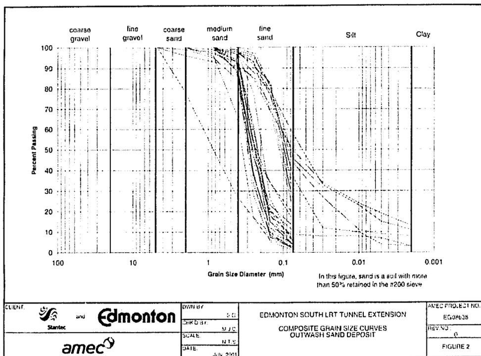
Figure 3-18 Composite grain size distributions for Outwash Sands (AMEC).
