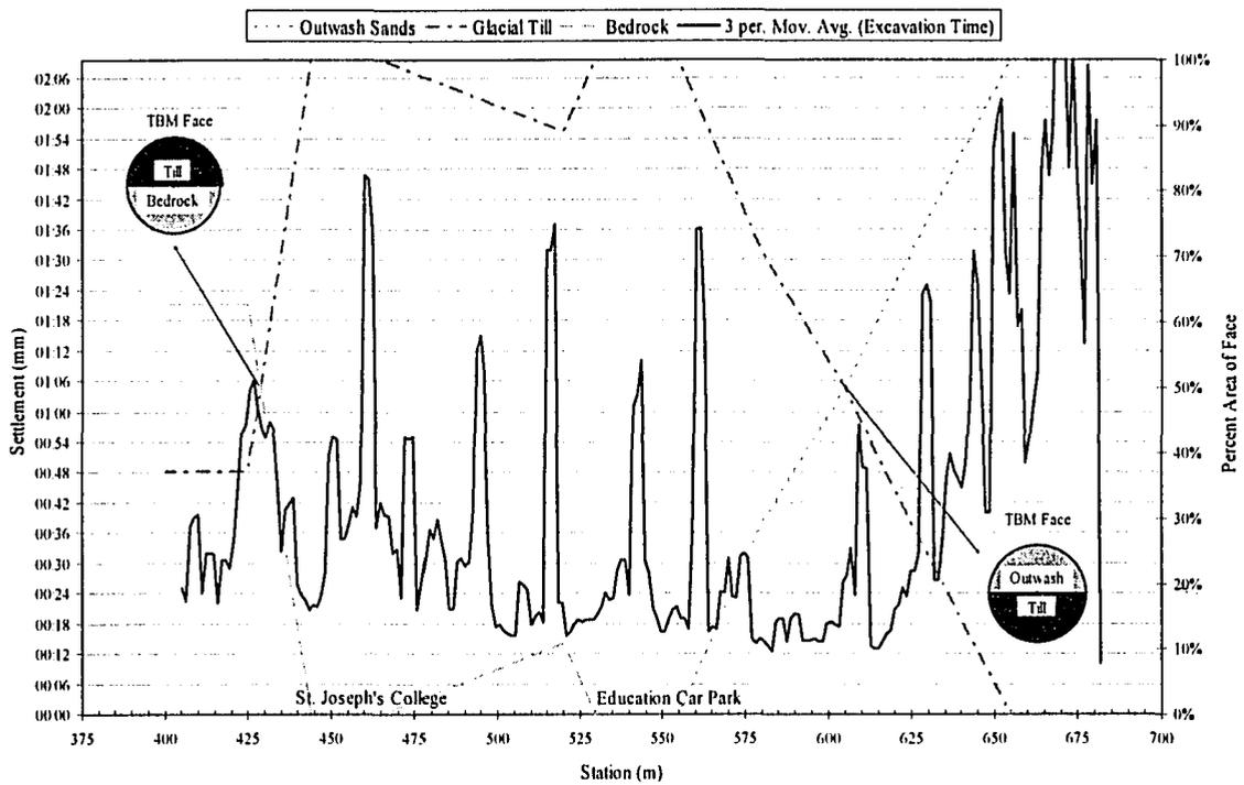
Figure 5-7 Excavation time per ring for construction of Southbound Tunnel with inferred
