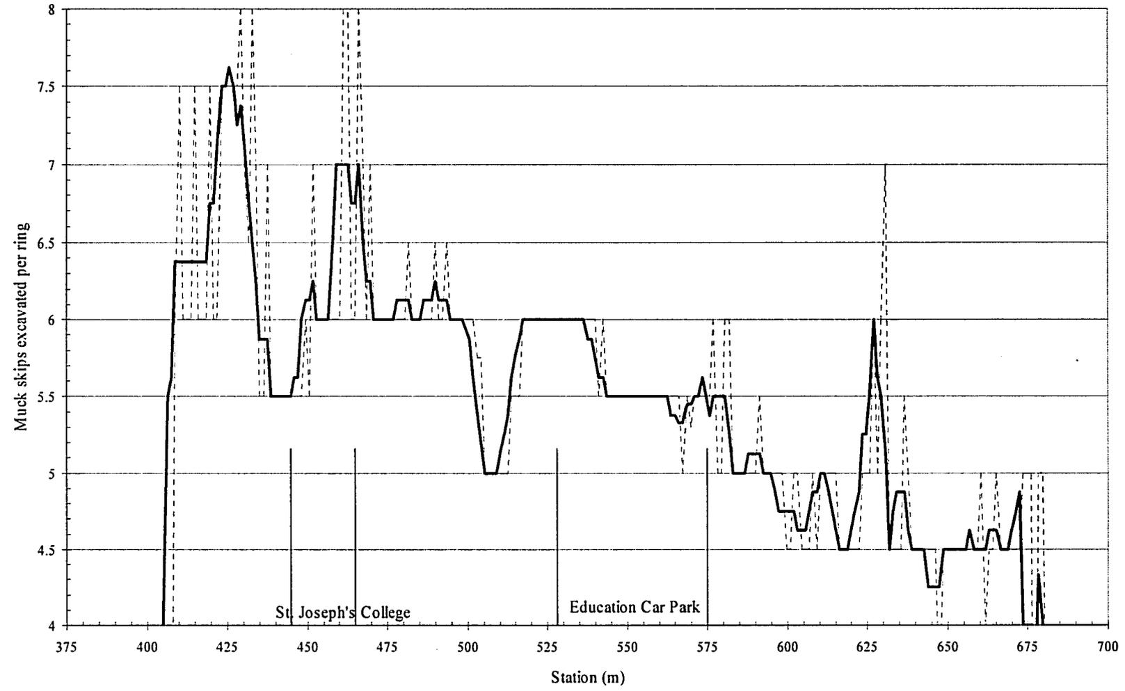
Figure 4-19 Muck cars needed per ring of excavation during construction of Southbound LRT Tunnel.
