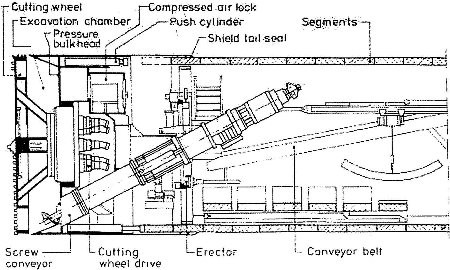
Figure 2-1 Generalised cross-section of an Equalised Pressure Balance Tunnel Boring Machine (Maidl et al., 1996)
