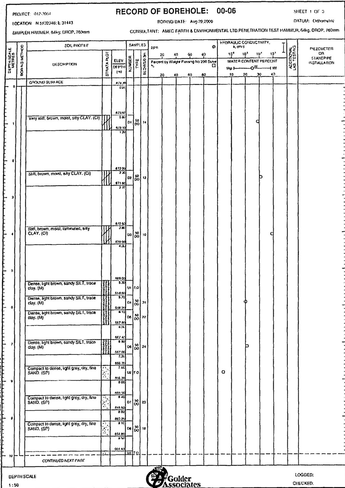
Figure B-1 A selection of the borehole log for Borehole 00-06 focusing on the Lake Edmonton Clay (AMEC)
