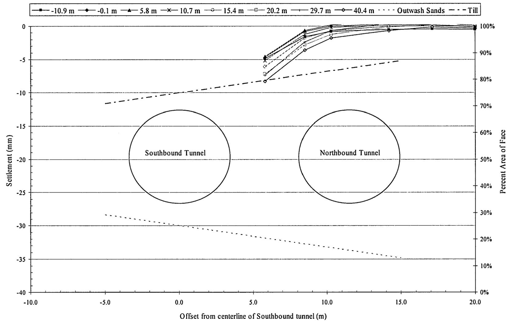
Figure 4-44 Observed shallow settlement at Array C during construction of Northbound Tunnel.
