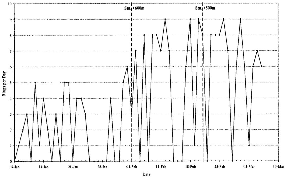
Figure 4-13 Rings built per day during construction of Northbound LRT Tunnel (2005).
