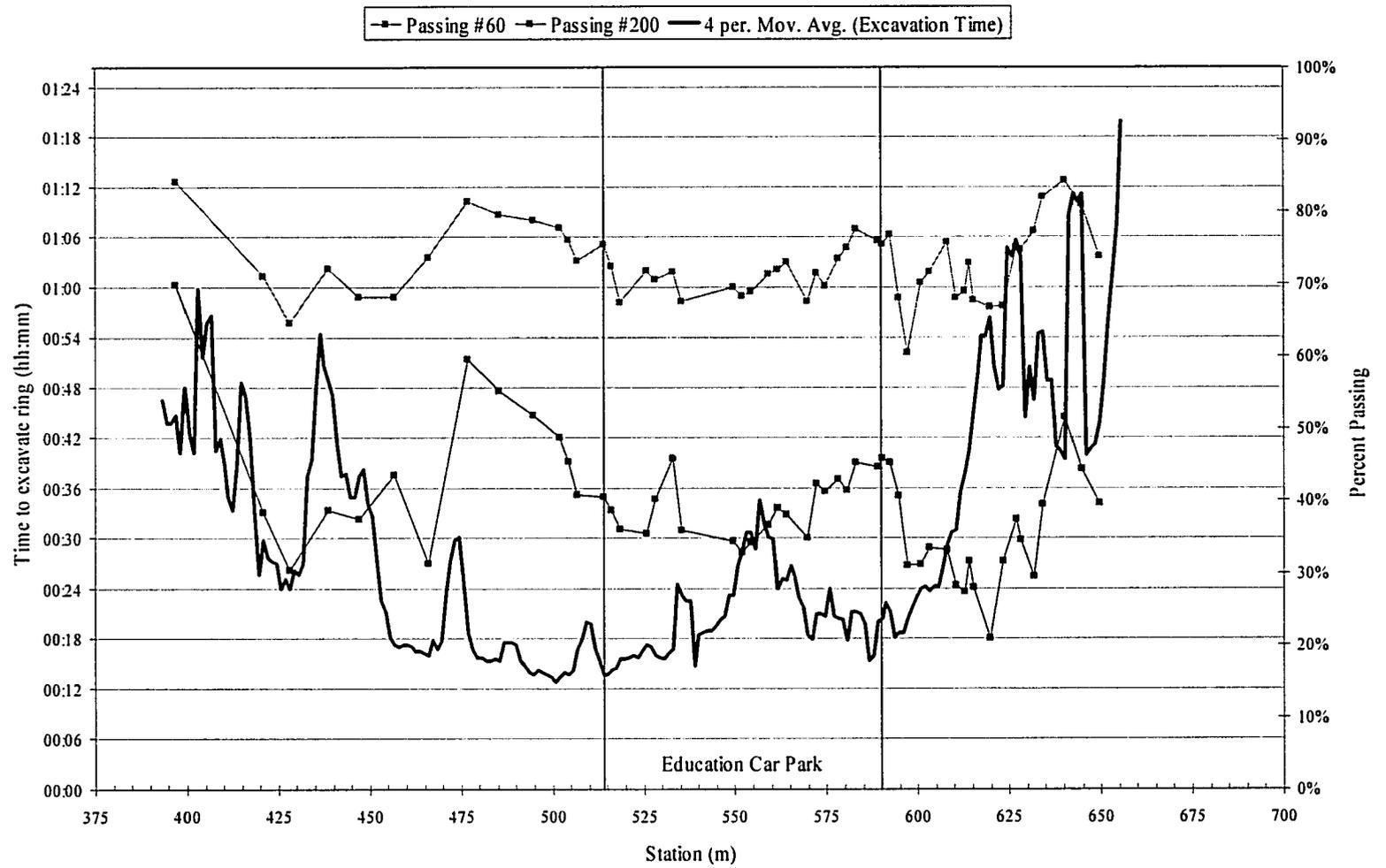
Figure 5-6 Excavation time per ring for construction of Northbound Tunnel with the fraction of TBM spoil passing the #60 and #200 sieve.
