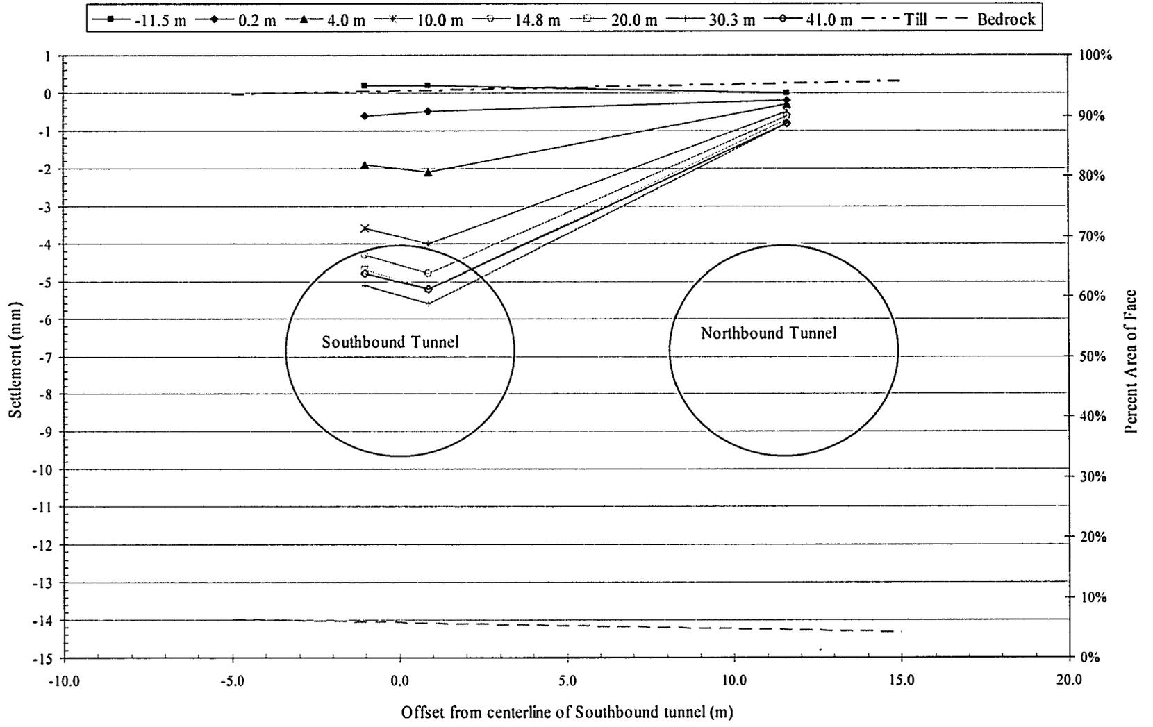
Figure H-7 Observed deep settlement at Array A during construction of Southbound Tunnel.
