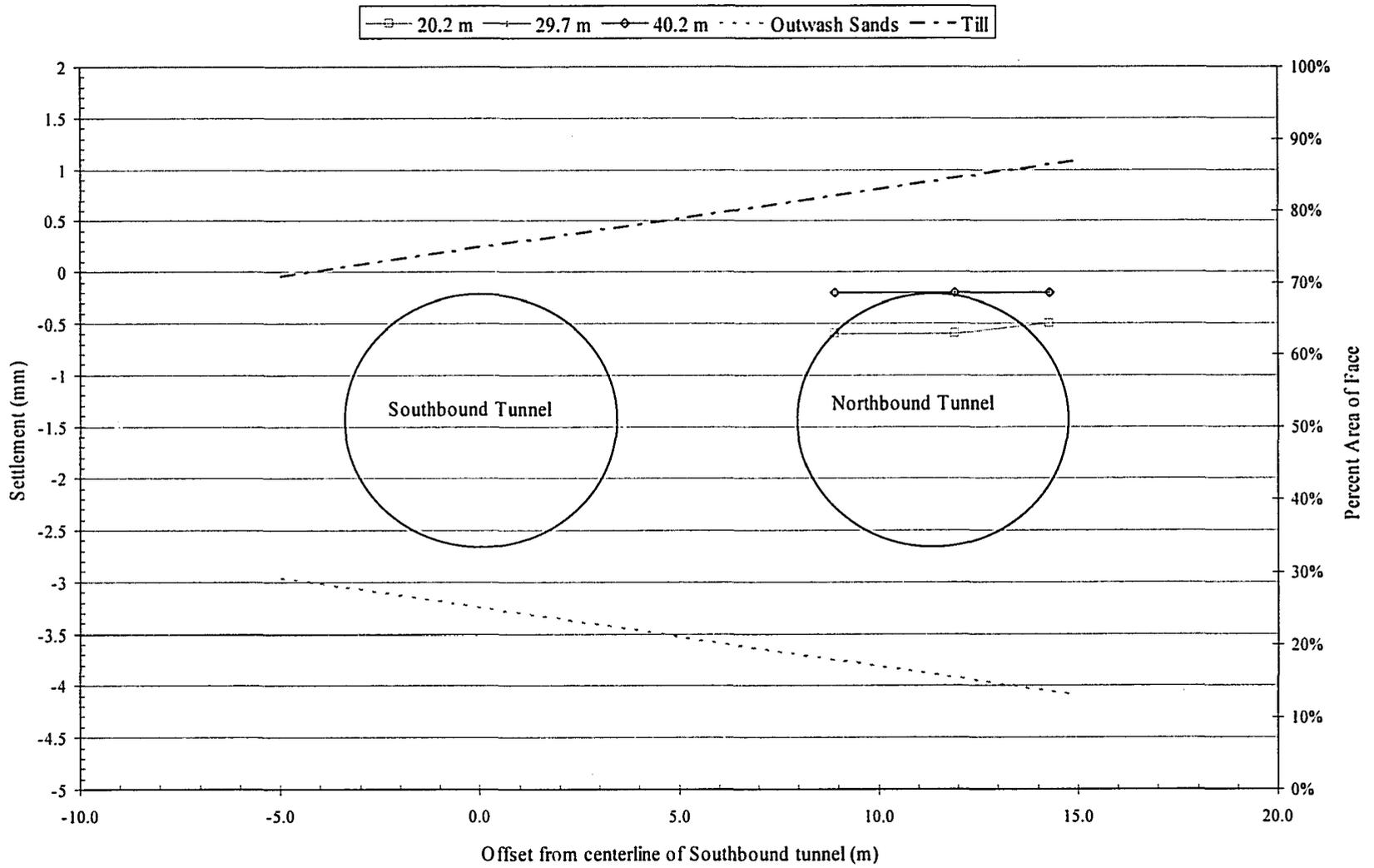
Figure H-3 Observed deep settlement at Array C during construction of Southbound Tunnel.
