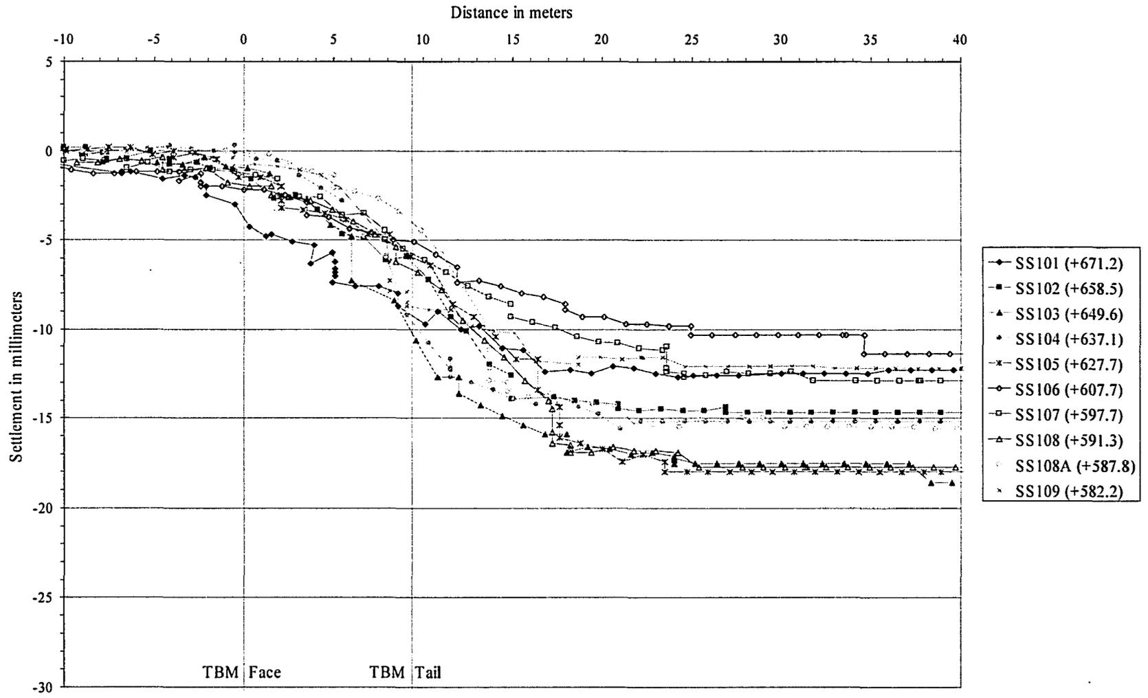
Figure 4-27 Observed shallow settlements during construction of Southbound Tunnel with proximity to TBM face, from Portal to Education Car Park.
