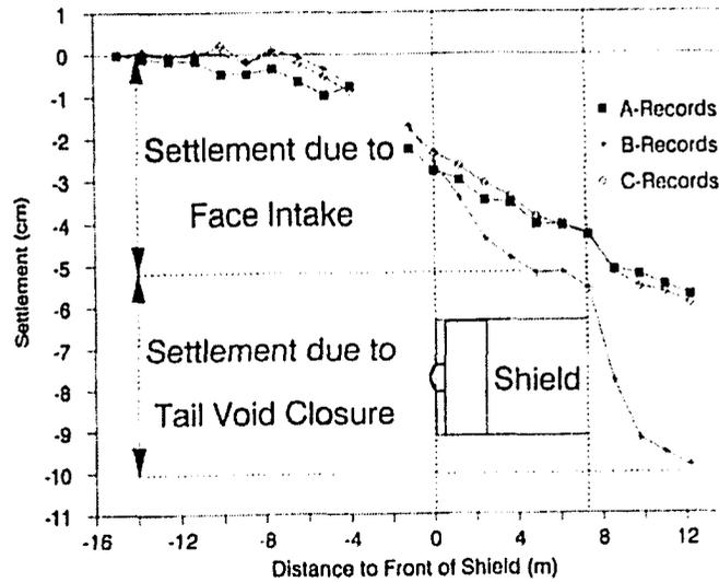
Figure 2-6 Settlement with proximity to EPB-TBM – Tunnel crown in sand, invert in clay (Clough and Leca, 1993)
