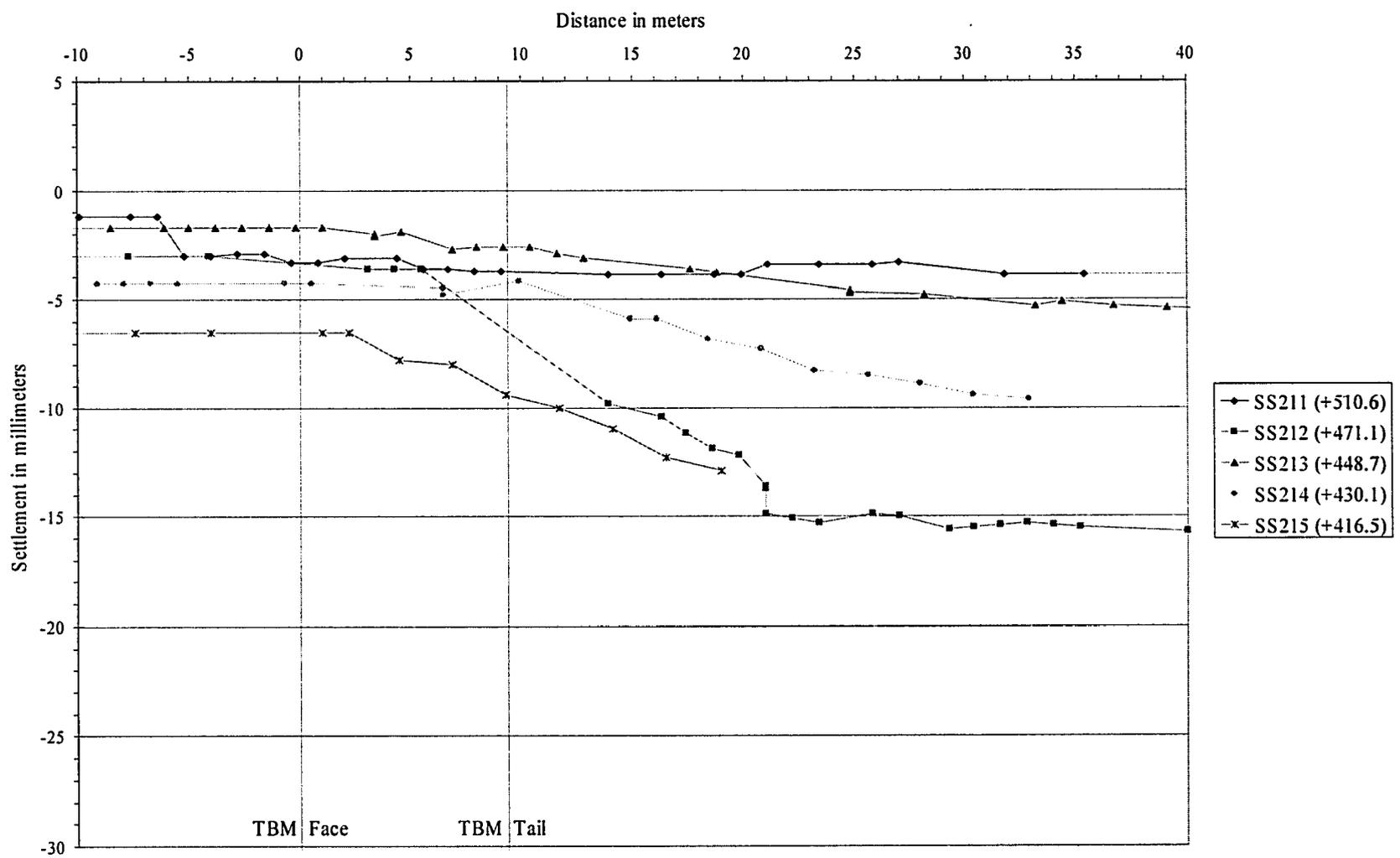
Figure 4-33 Observed shallow settlements during construction of Northbound Tunnel with proximity to TBM face, from Education Car Park to breakthrough.
