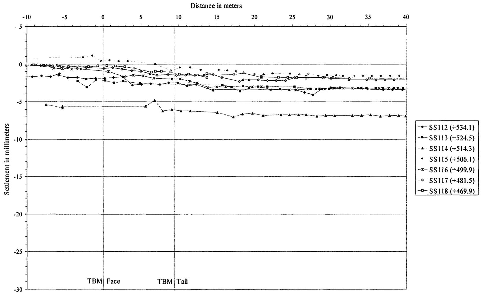
Figure 4-29 Observed shallow settlements during construction of Southbound Tunnel with proximity to TBM face, Education Car Park to St. Joseph's College.
