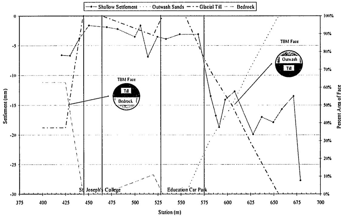
Figure 5-17 Observed shallow settlements during Southbound construction contrasted with inferred stratigraphy.
