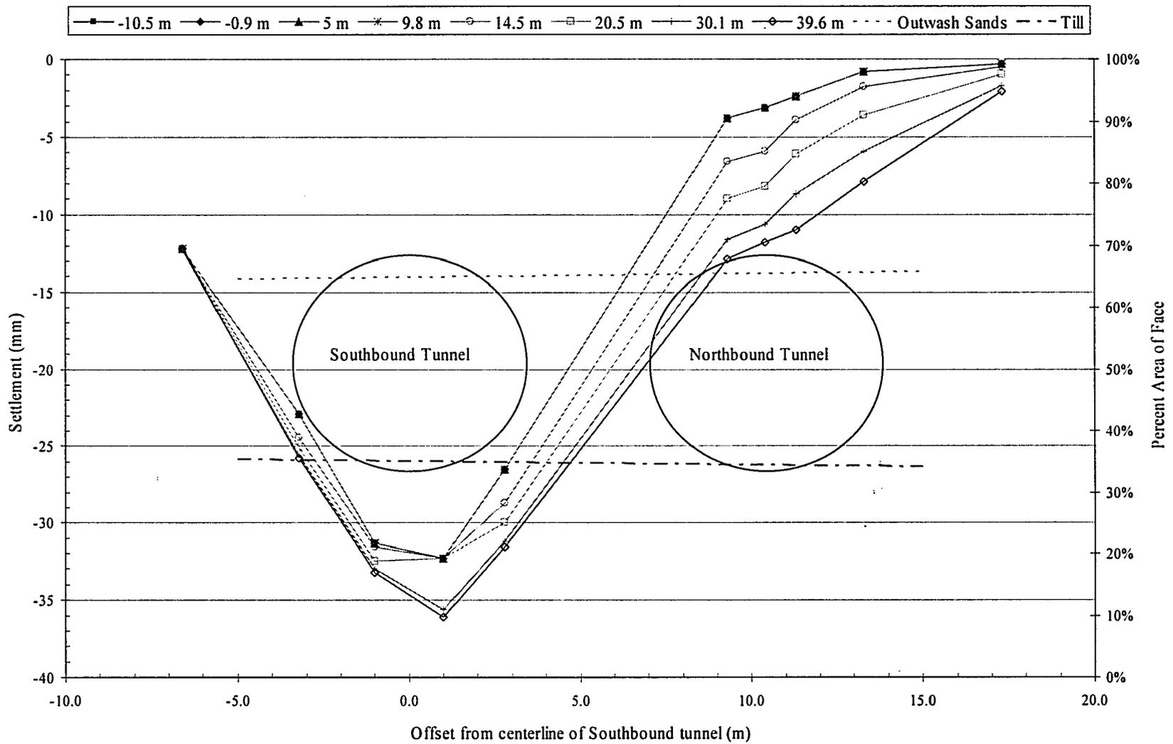
Figure 4-42 Observed shallow settlement at Array D during construction of Northbound Tunnel.
