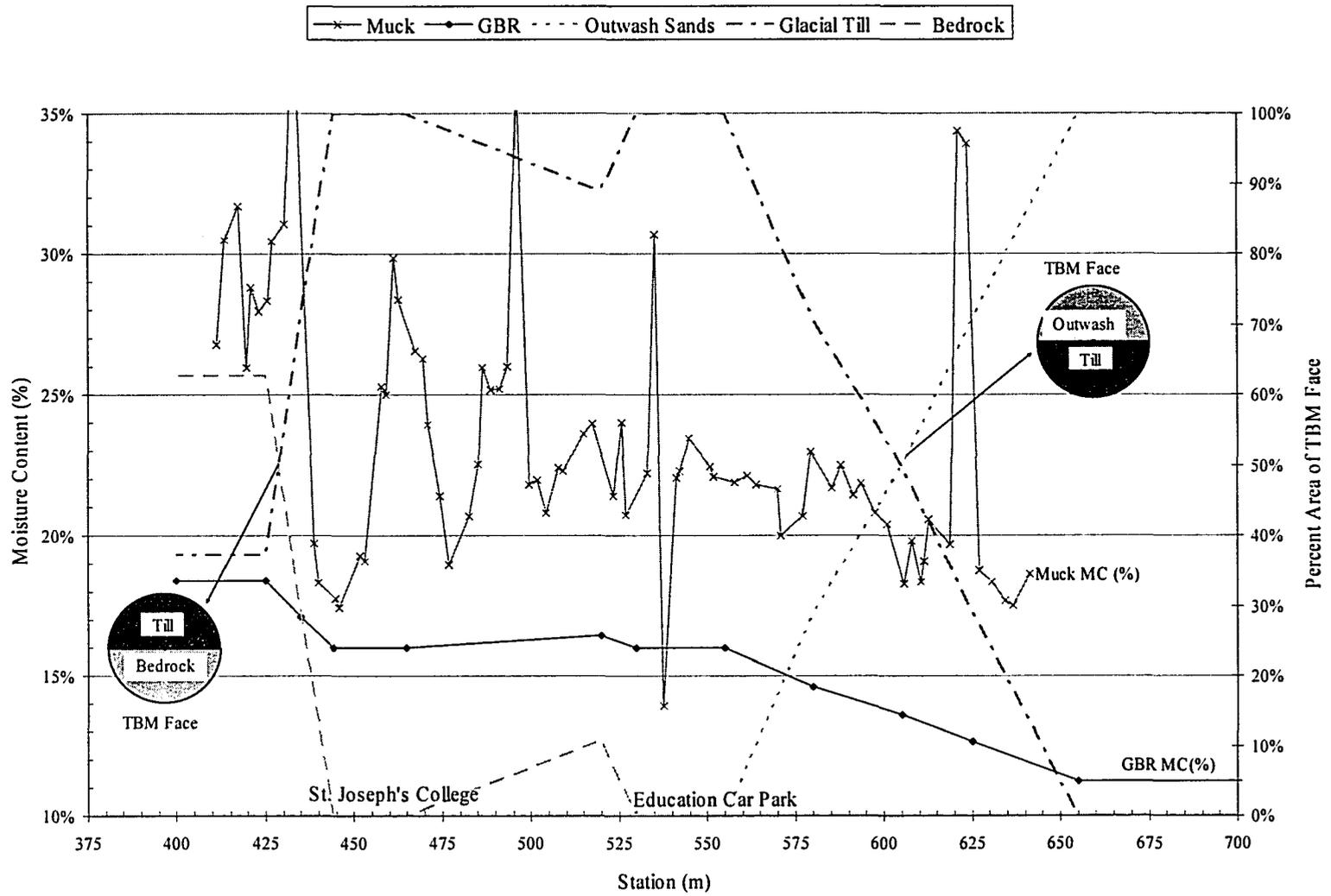
Figure 4-3 Moisture content of material excavated during construction of the Southbound LRT Tunnel and the inferred in-situ moisture content of the soil.
