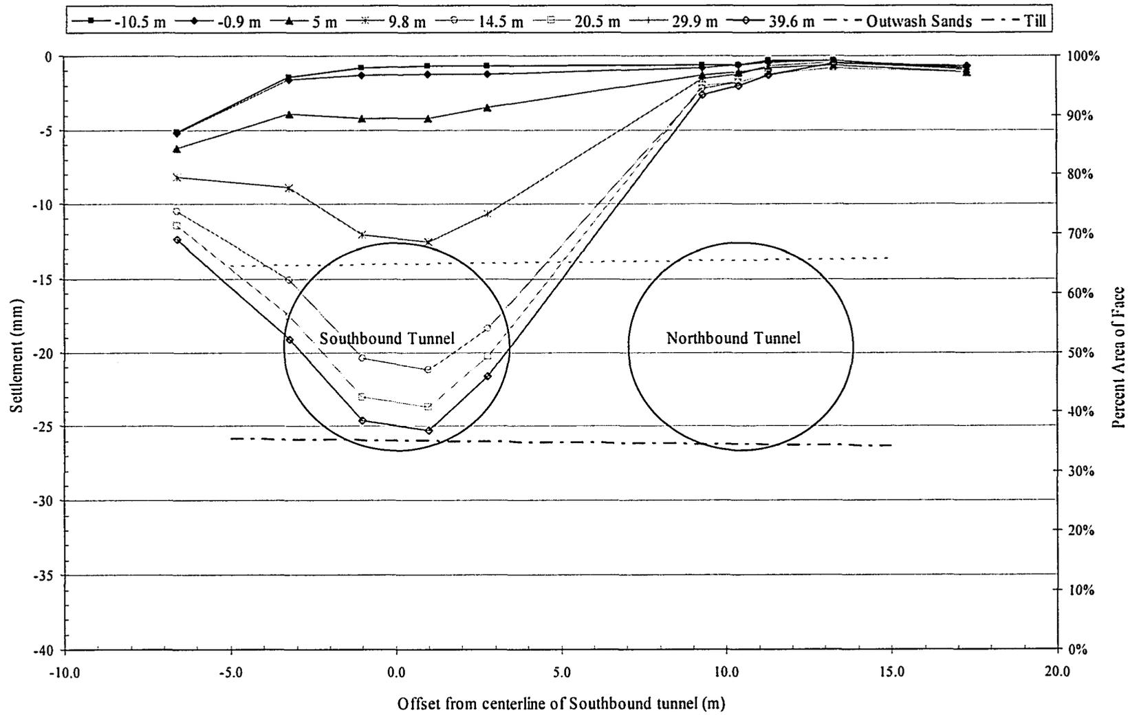
Figure 4-41 Observed shallow settlement at Array D during construction of Southbound Tunnel.
