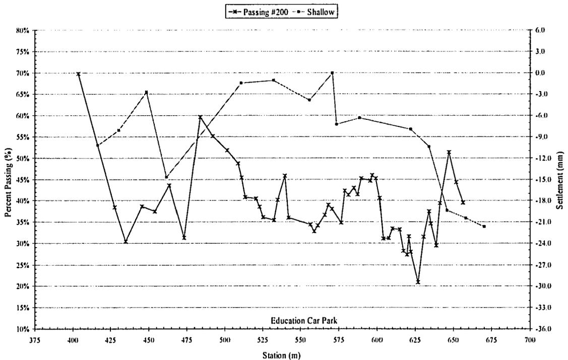
Figure 5-20 Observed shallow settlements during Northbound construction contrasted with grain size distribution of TBM spoil.
