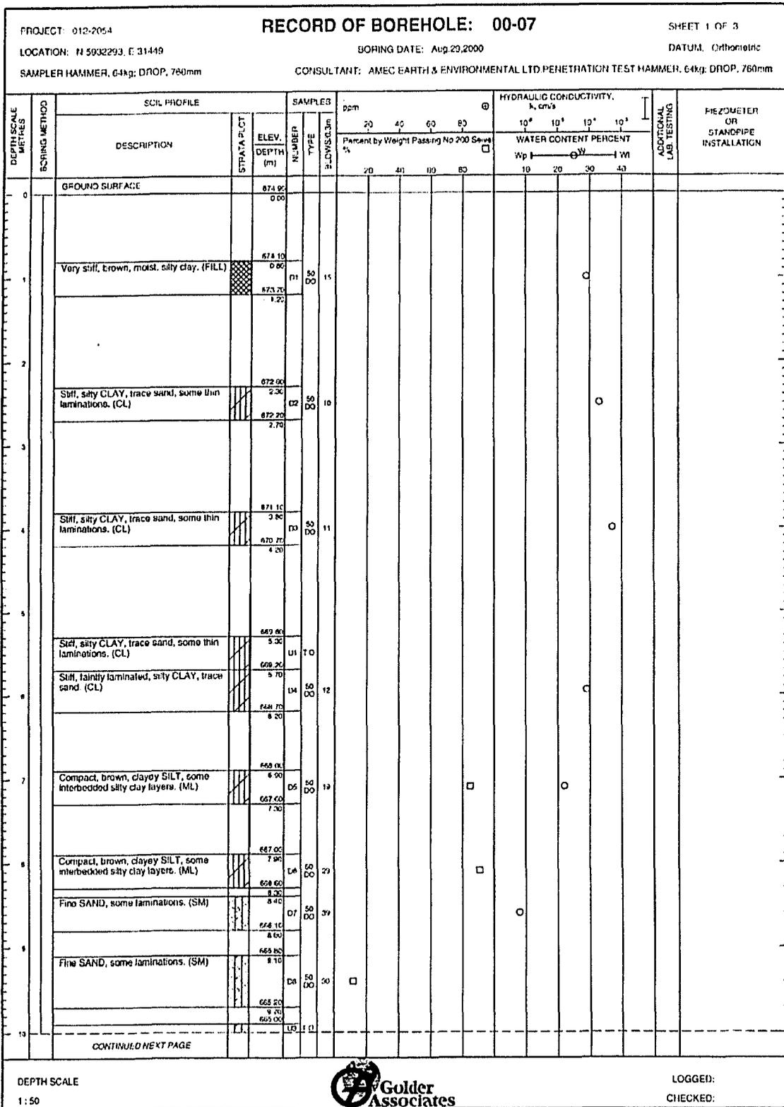
Figure B-2 A selection of the borehole log for Borehole 00-07 focusing on the Lake Edmonton Clay (AMEC).
