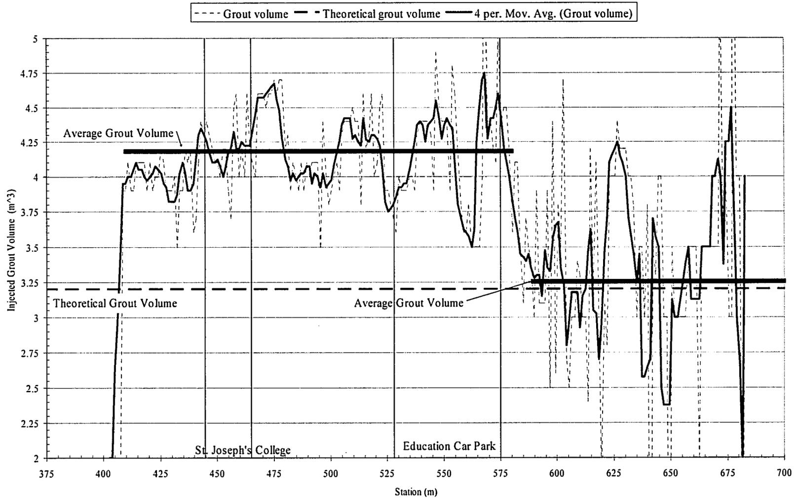
Figure 4-15 Injected grout volume per ring of excavation during construction of Southbound LRT Tunnel.
