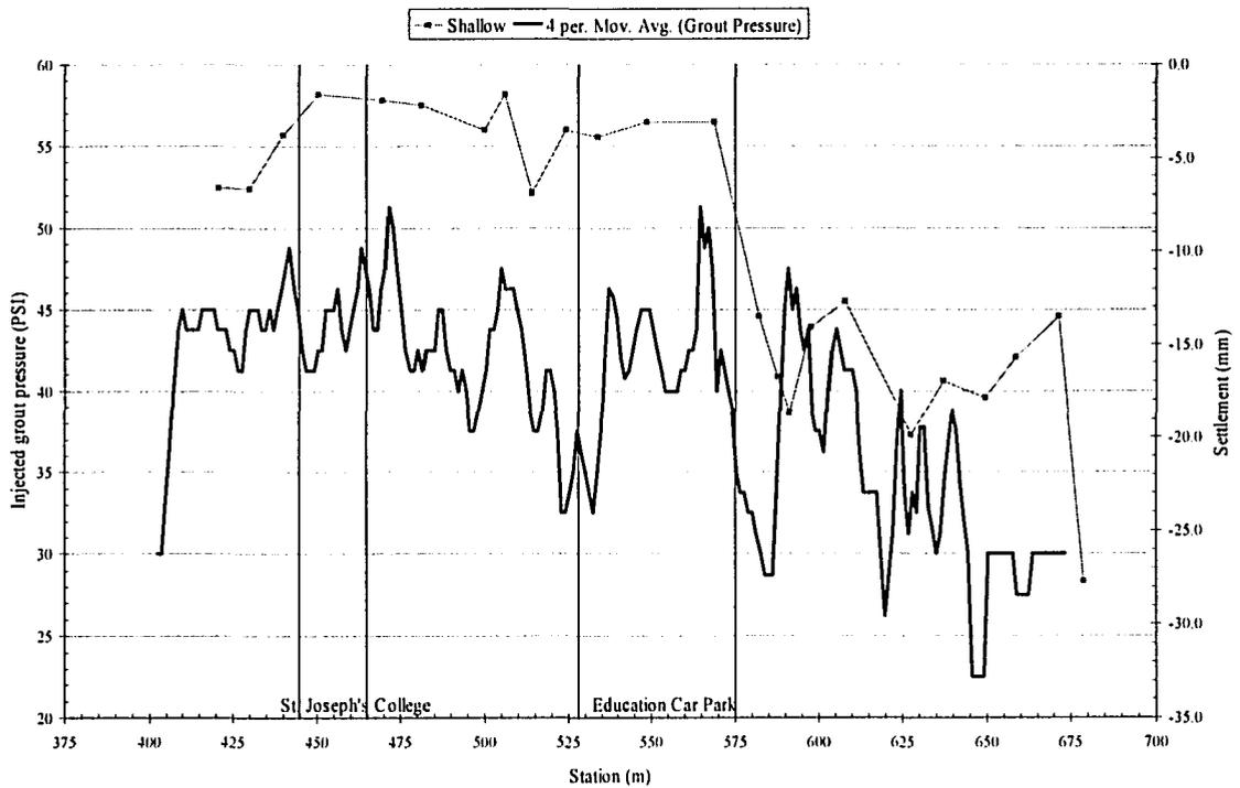
Figure 5-14 Injected grout pressure per ring of advance during Southbound construction contrasted with observed shallow settlements.
