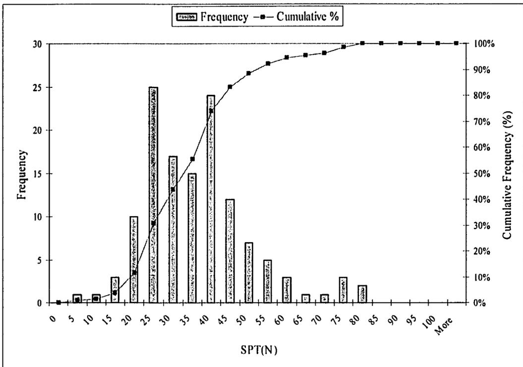
Figure 3-15 Histogram of SPT(N) blows per 300mm in Outwash Sands and Silts.
