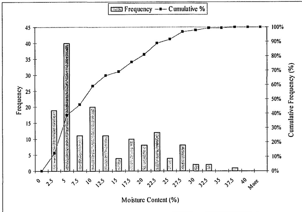
Figure 3-20 Histogram of observed Moisture Contents of the Outwash Sands and Silts.
