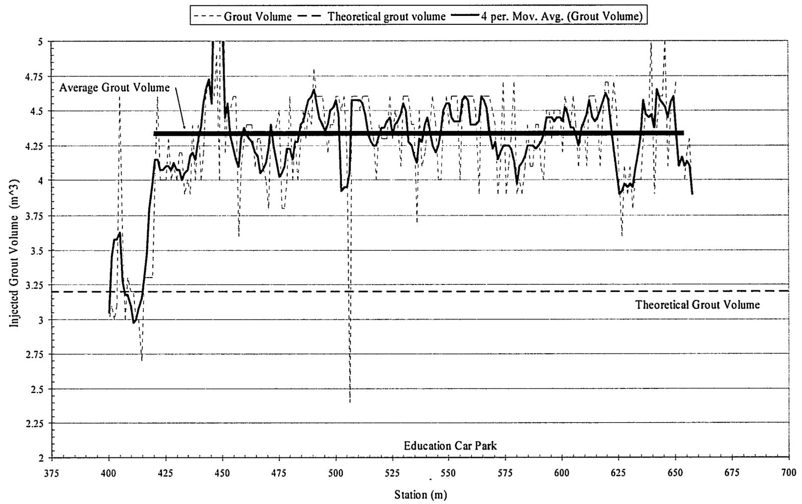
Figure 4-16 Injected grout volume per ring of excavation during construction of Northbound LRT Tunnel.
