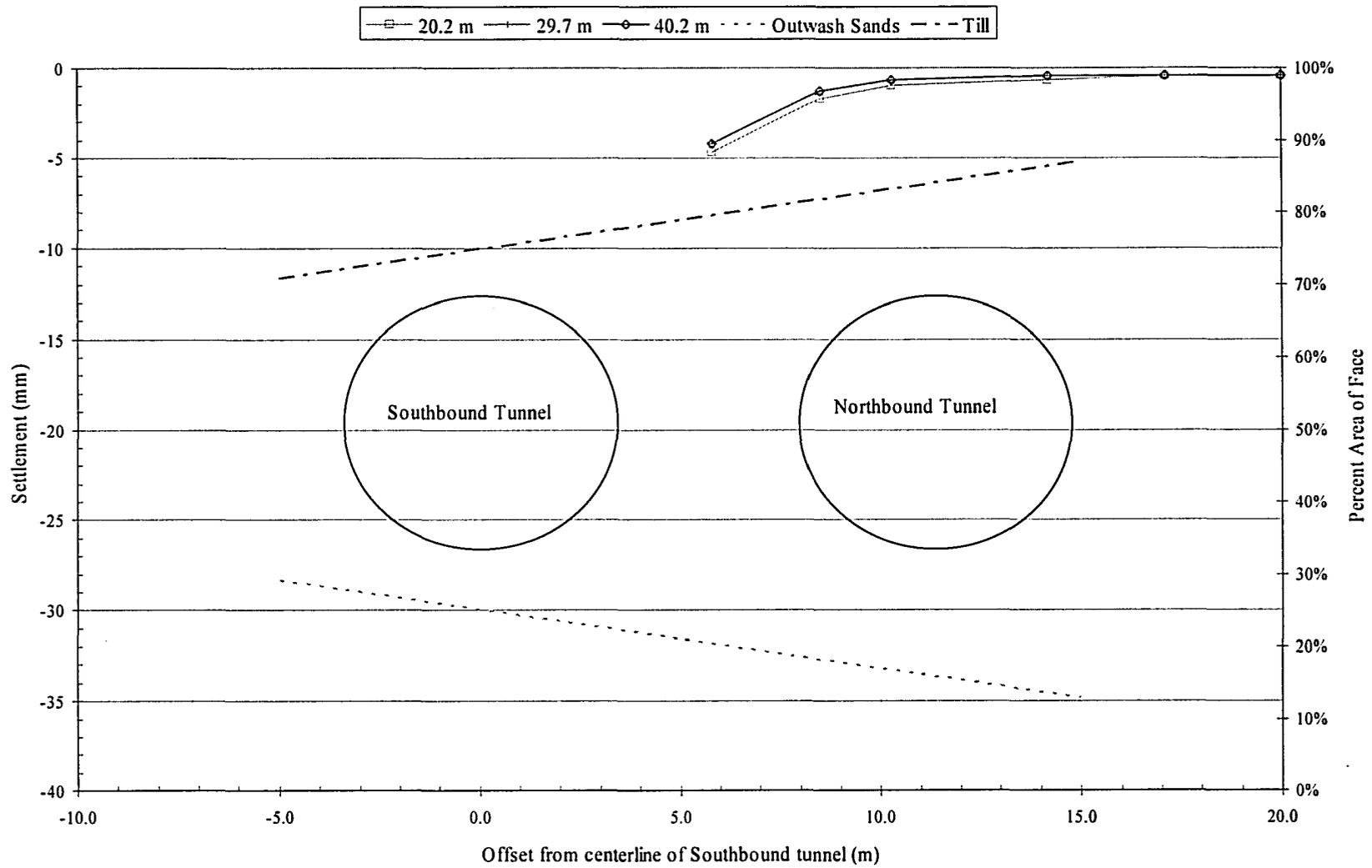
Figure 4-43 Observed shallow settlement at Array C during construction of Southbound Tunnel.
