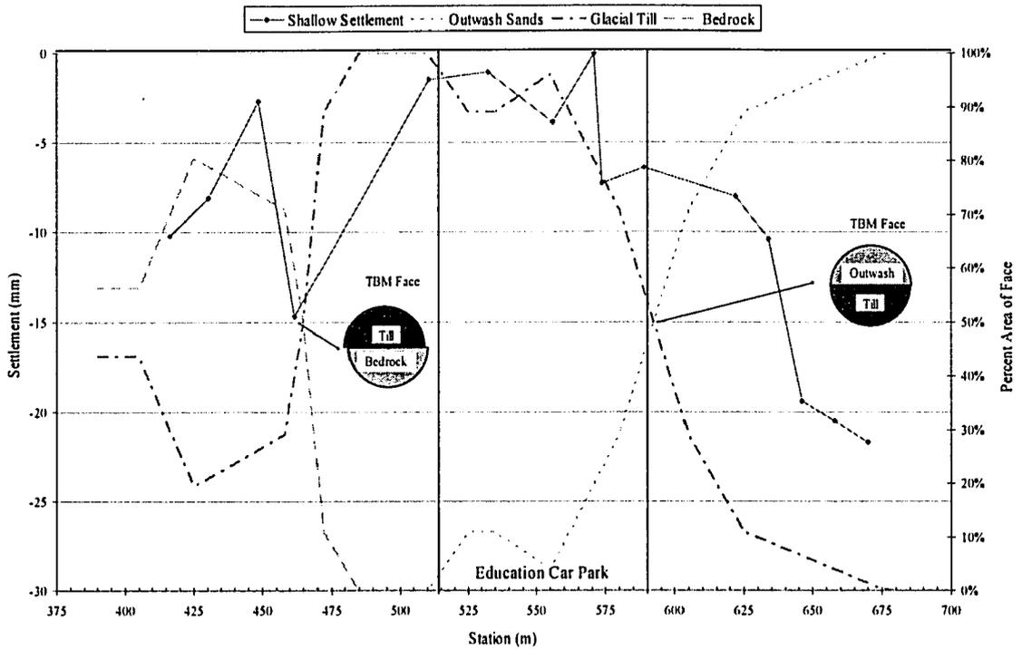
Figure 5-19 Observed shallow settlements during Northbound construction contrasted with the inferred stratigraphy.
