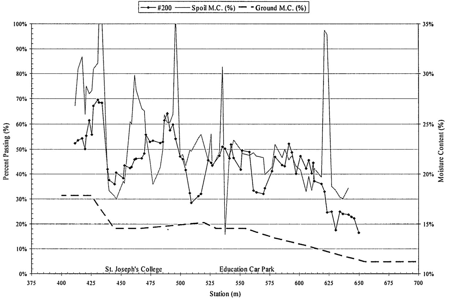
Figure 5-1 TBM spoil moisture content with inferred in-situ moisture content with the percentage of TBM spoil passing the #200 Sieve during Southbound construction.
