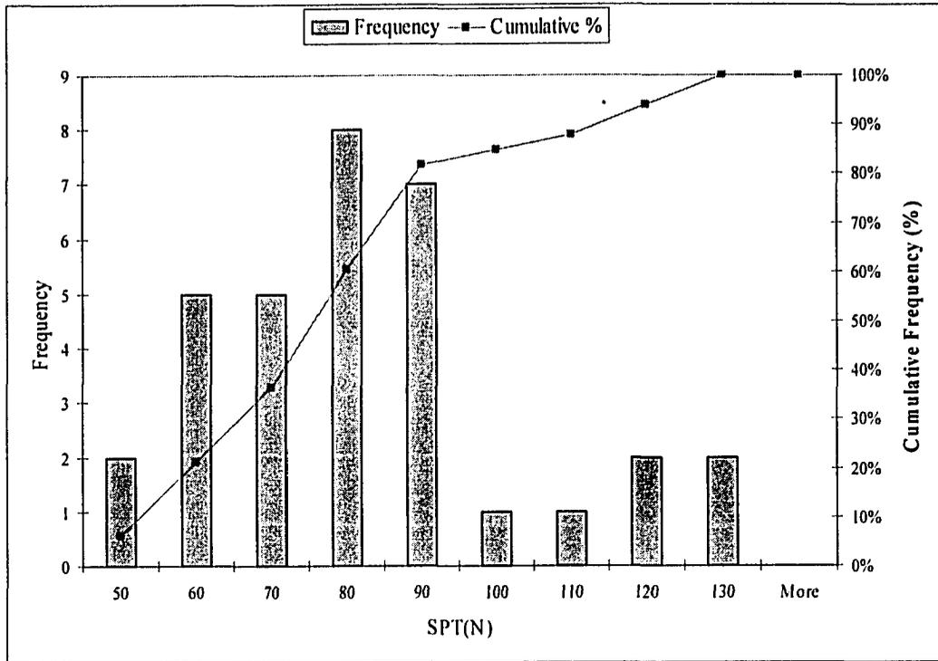
Figure 3-32 Histogram of SPT(N) values per 300mm in Bedrock.
