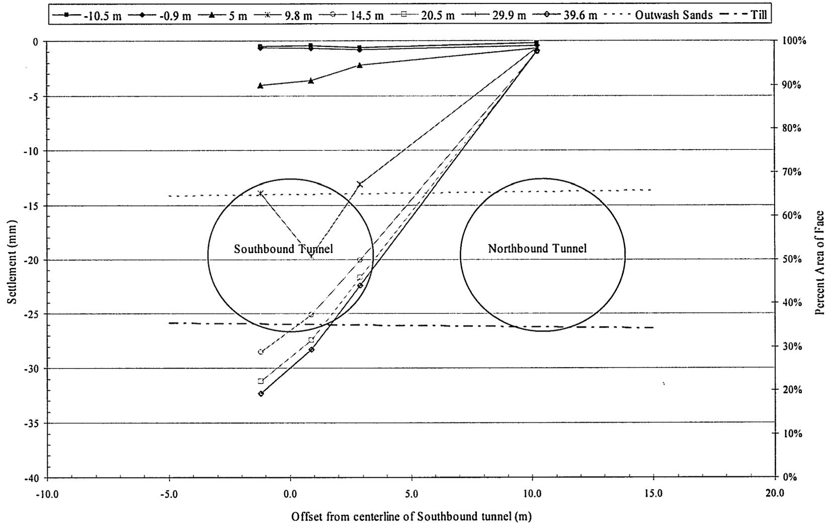
Figure H-1 Observed deep settlement at Array D during construction of Southbound Tunnel.
