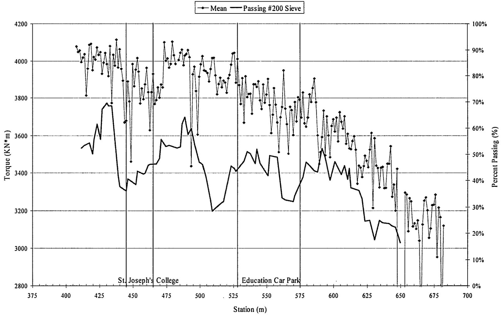
Figure 5-12 Mean operational torque during construction of the Southbound Tunnel.
