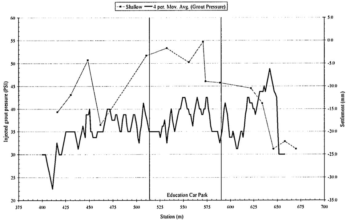
Figure 5-16 Injected grout pressure per ring of advance during Northbound construction contrasted with observed shallow settlements.
