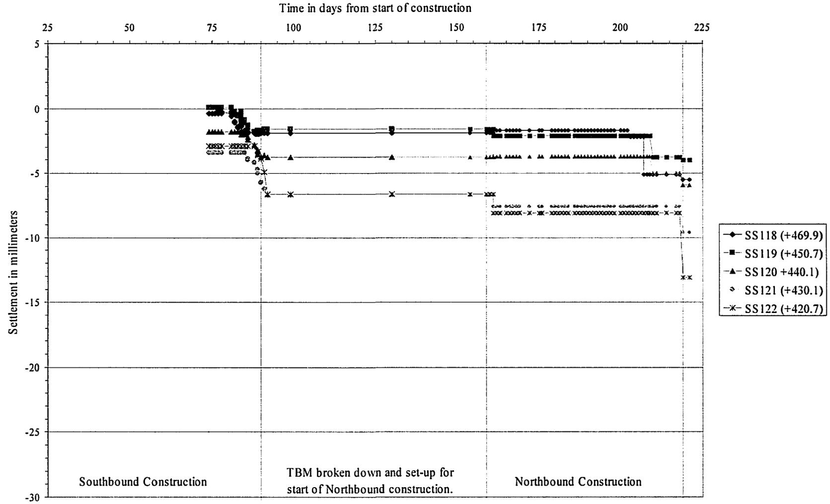
Figure 4-37 Observed shallow settlements in Southbound alignment instruments over the course of construction with respect to time, from St. Joseph's College to breakthrough.
