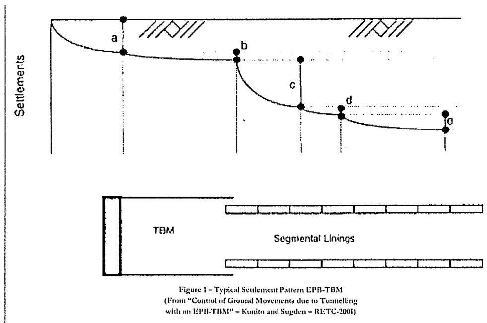
Figure 2-4 Generalised settlement profile for EPB-TBM, by region (Kunito and Sugden, 2001)
