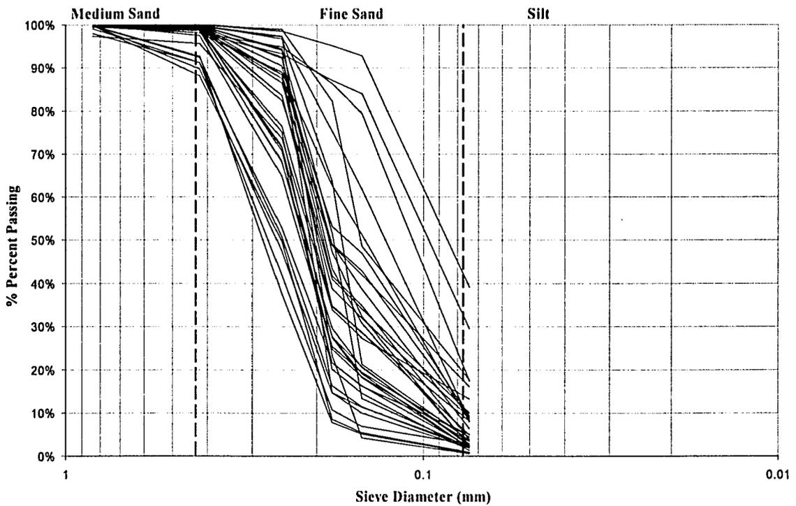
Figure 3-16 Grain size distributions of Outwash Sands and Silts collected during mapping of open cut excavation.
