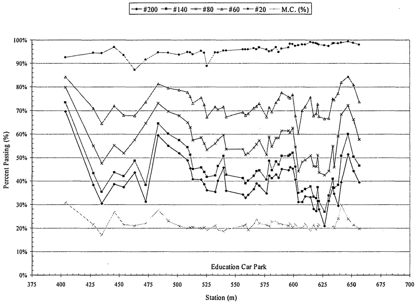
Figure 4-6 Grain size distribution and moisture content of material excavated during construction of Northbound LRT Tunnel.
