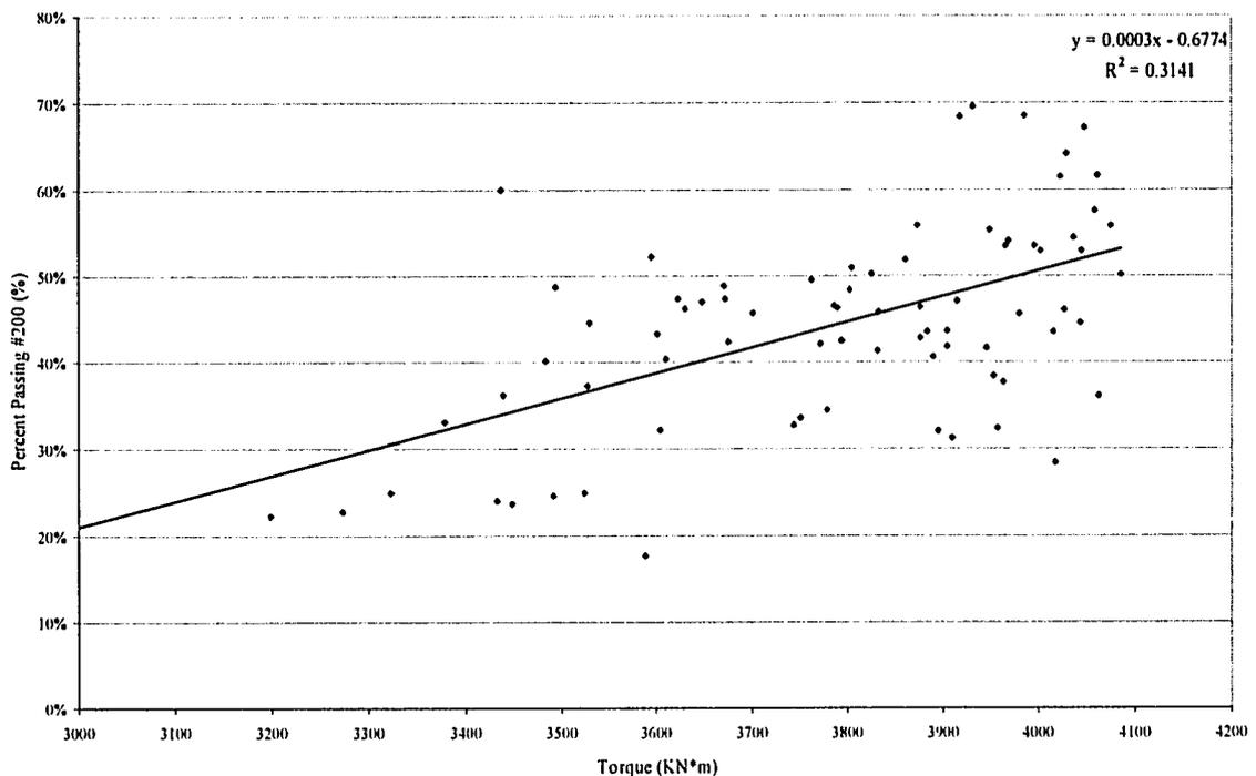
Figure 5-11 Correlation between percent passing #200 and mean operational torque for the construction of the Southbound Tunnel.
