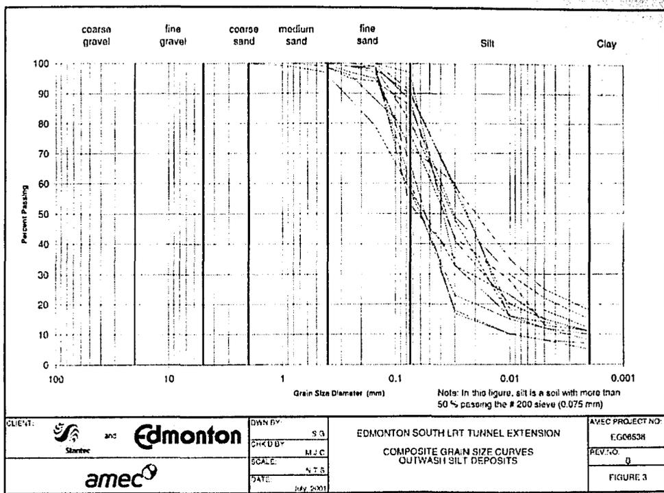
Figure 3-19 Composite grain size distributions for Outwash Silts (AMEC)
