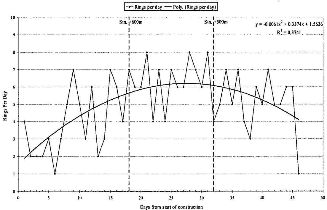
Figure 4-12 Rings built per day during construction of Southbound LRT Tunnel (2004).
