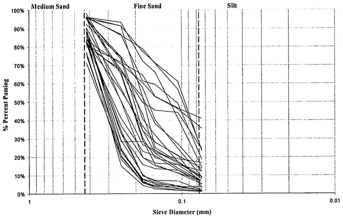
Figure 3-17 Grain size distributions of Outwash Sands and Silts collected from hollow and solid stem augurs during installation of settlement points.
