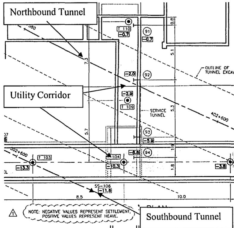
Figure 4-26 Layout of utility corridor and the location of survey points.
