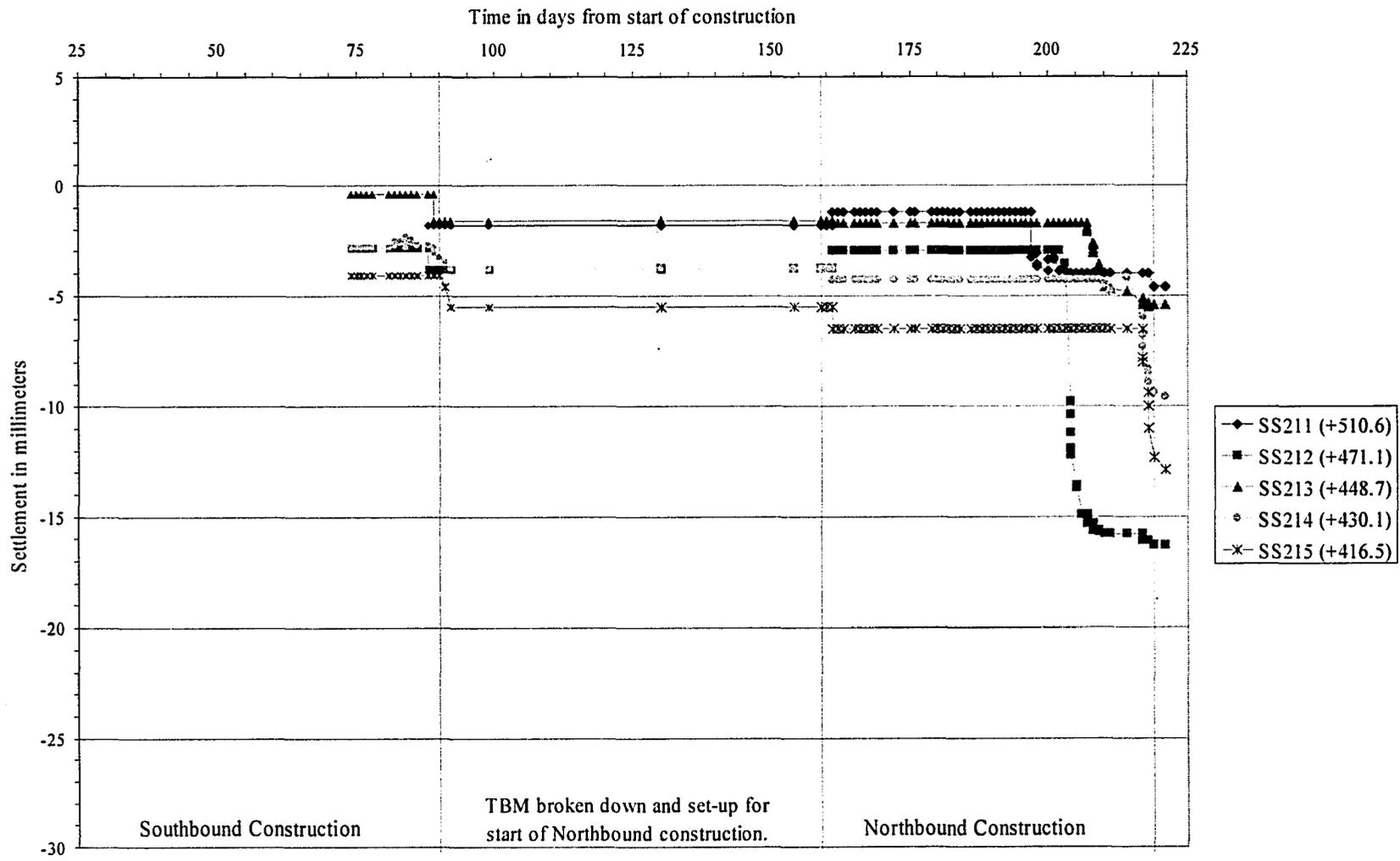
Figure 4-40 Observed shallow settlements in Northbound alignment instruments over the course of construction with respect to time, from the Education Car Park to removal shaft.
