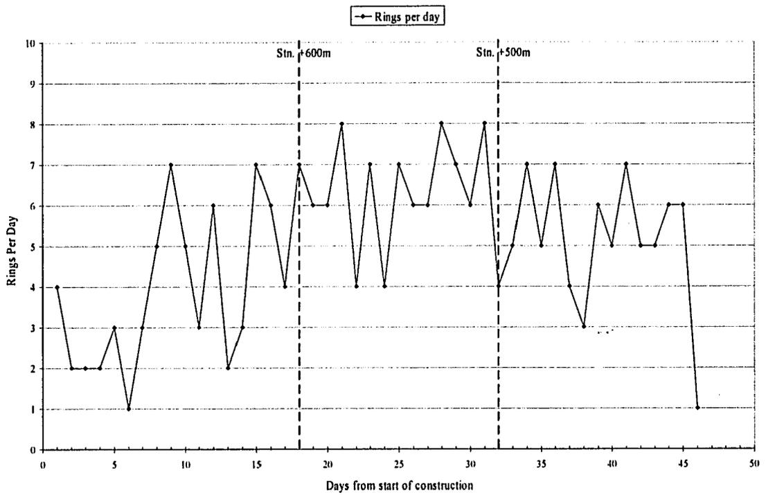
Figure 5-3 Rings constructed per day during construction of the Southbound Tunnel.
