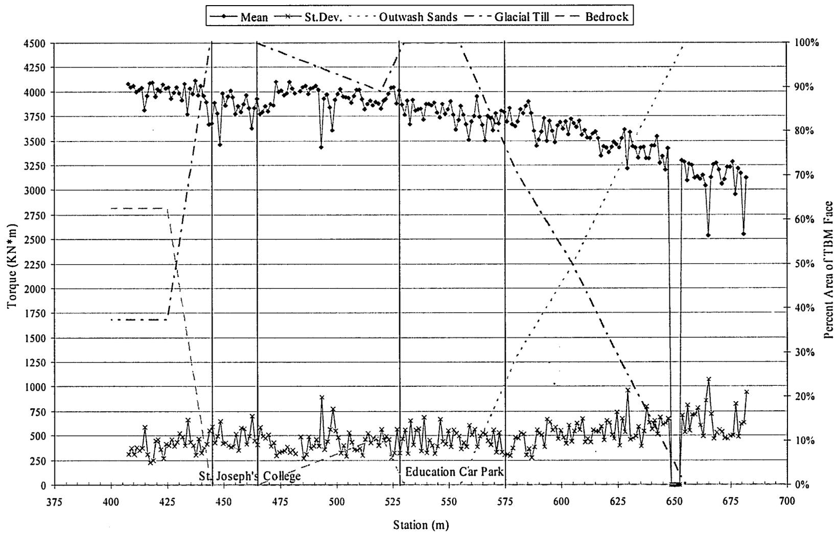
Figure 4-7 Cutting-head torque recorded during advance of TBM, Southbound Tunnel.
