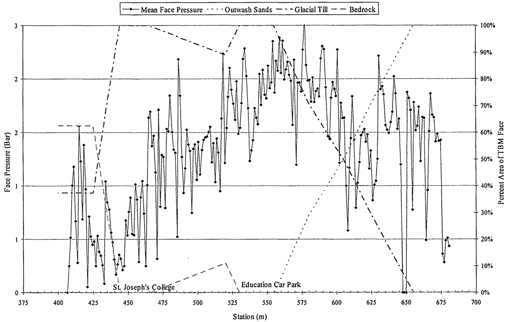
Figure 4-8 Face Pressure recorded during advance, Southbound Tunnel.
