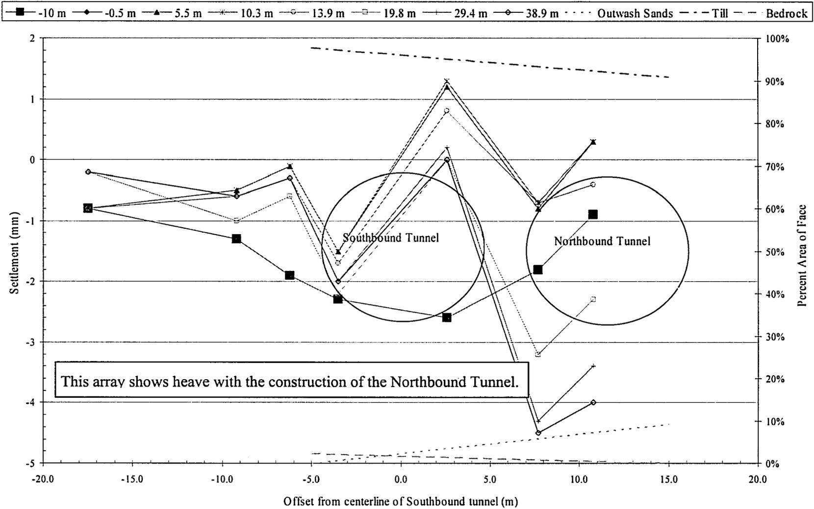
Figure 4-46 Observed shallow settlement at Array B during construction of Northbound Tunnel.
