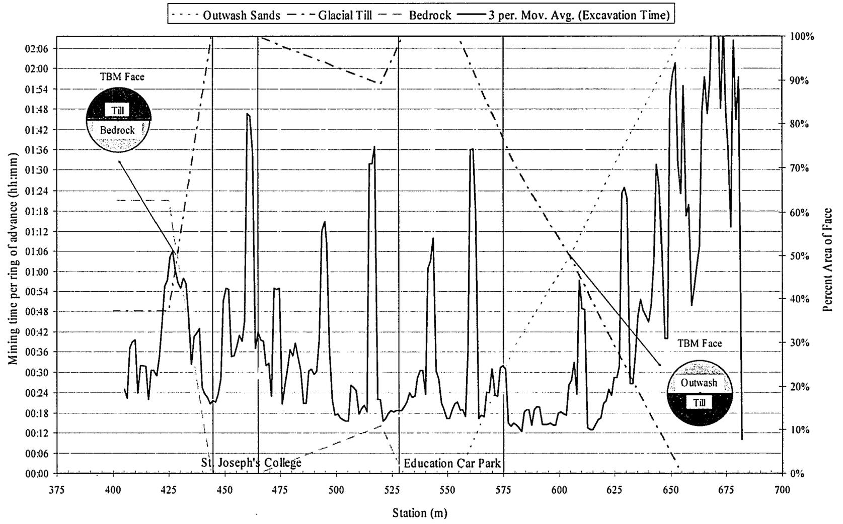
Figure 4-9 Time needed to excavate one ring during construction of Southbound LRT Tunnel.
