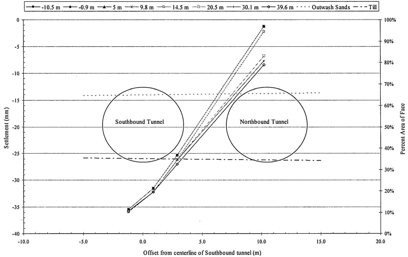
Figure H-2 Observed deep settlement at Array D during construction of Northbound Tunnel.
