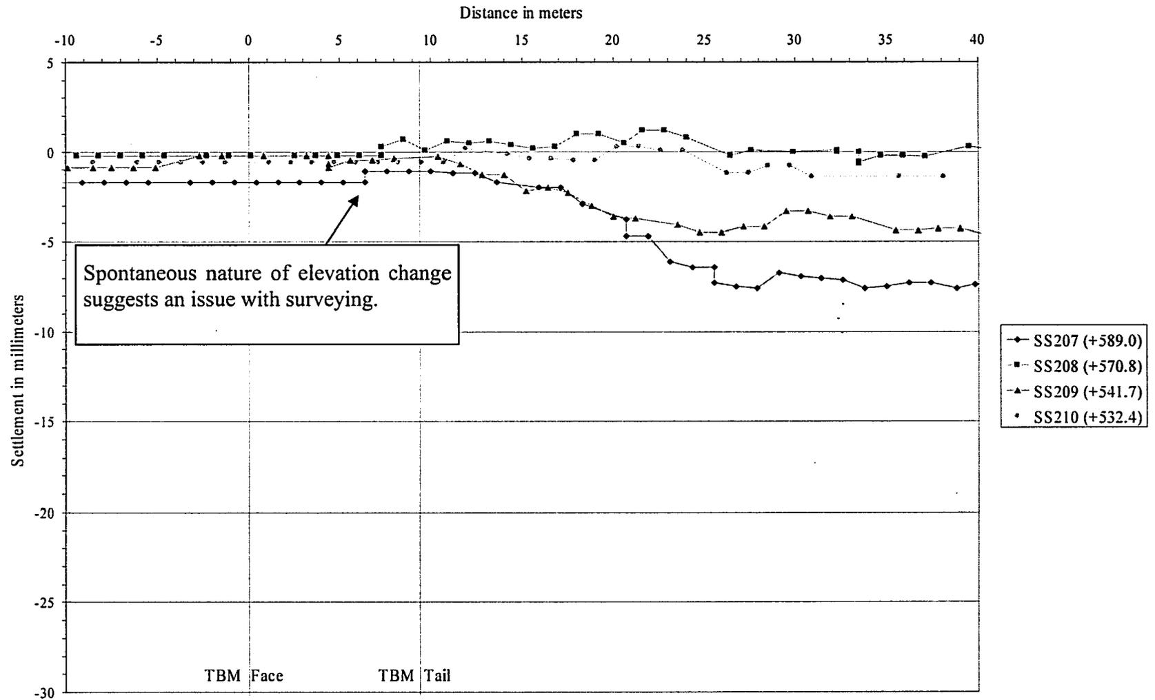
Figure 4-32 Observed shallow settlements during construction of Nouthbound Tunnel with proximity to TBM face, Education Car Park.
