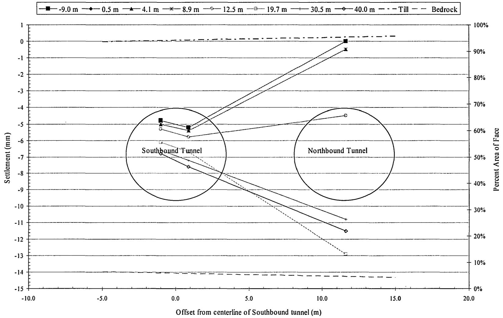
Figure H-8 Observed deep settlement at Array A during construction of Northbound Tunnel.
