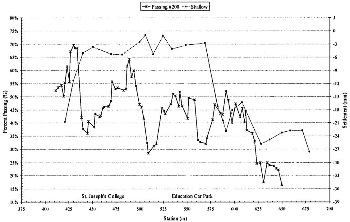
Figure 5-18 Observed shallow settlements during Southbound construction contrasted with grain size distribution of TBM spoil.
