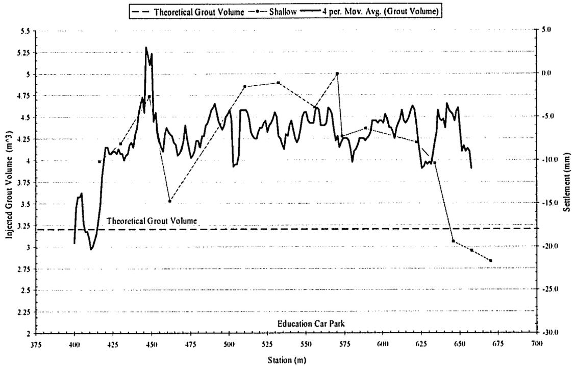
Figure 5-15 Injected grout volume per ring of advance during Northbound construction contrasted with observed shallow settlements.
