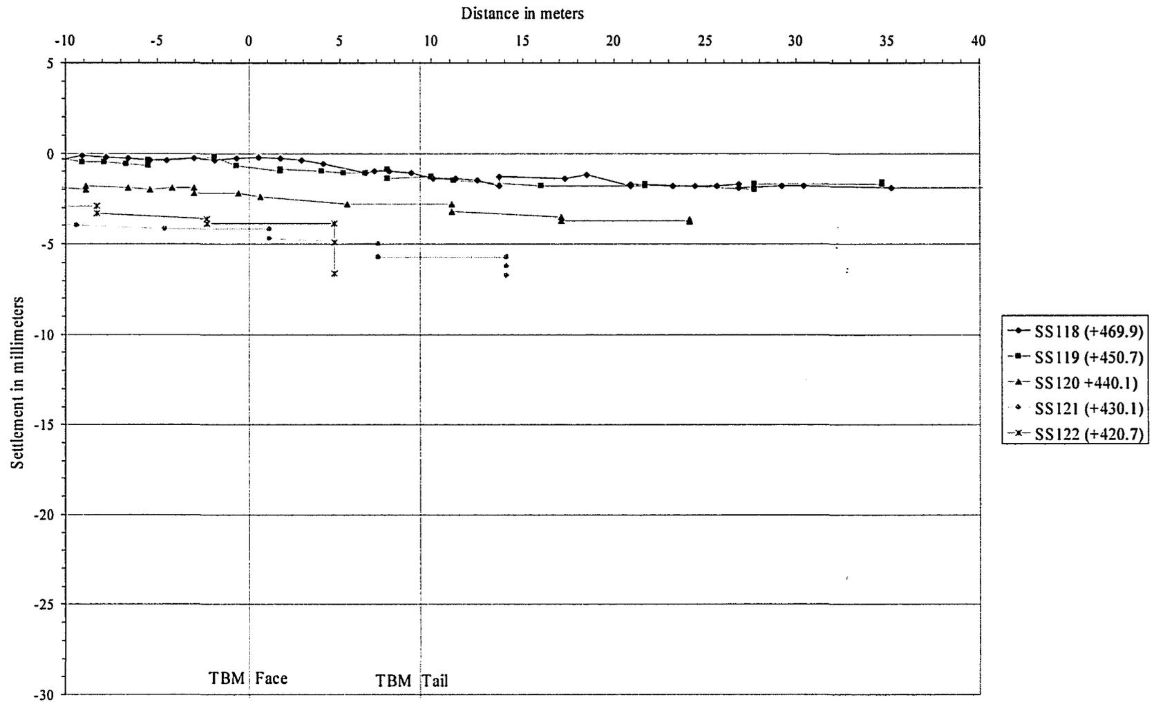
Figure 4-30 Observed shallow settlements during construction of Southbound Tunnel with proximity to TBM face, St. Joseph's College to breakthrough.
