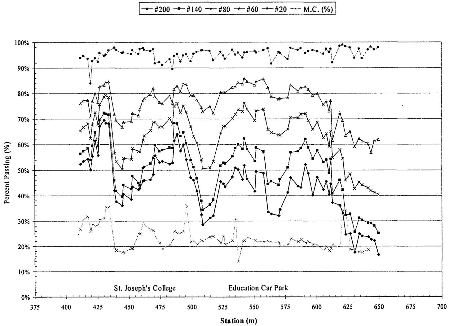
Figure 4-5 Grain size distribution and moisture content of material excavated during construction of Southbound LRT Tunnel.
