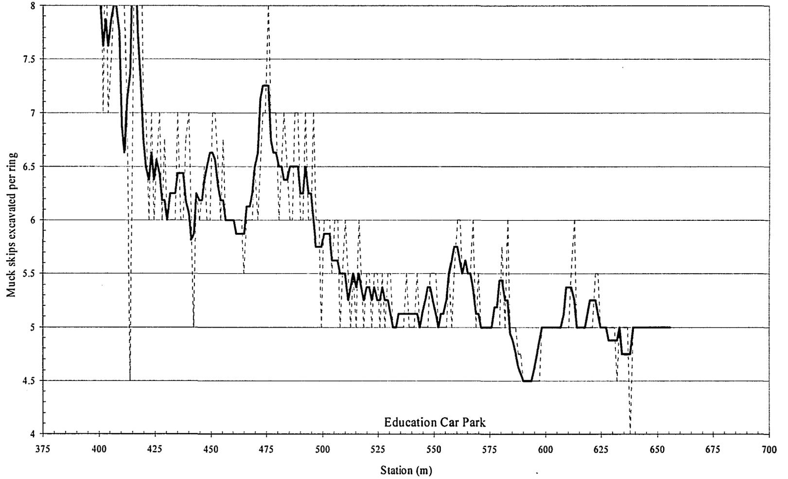
Figure 4-20 Muck cars needed per ring of excavation during construction of Northbound LRT Tunnel.
