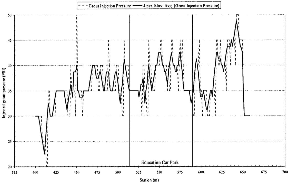
Figure 4-18 Injected grout pressure during Northbound construction.
