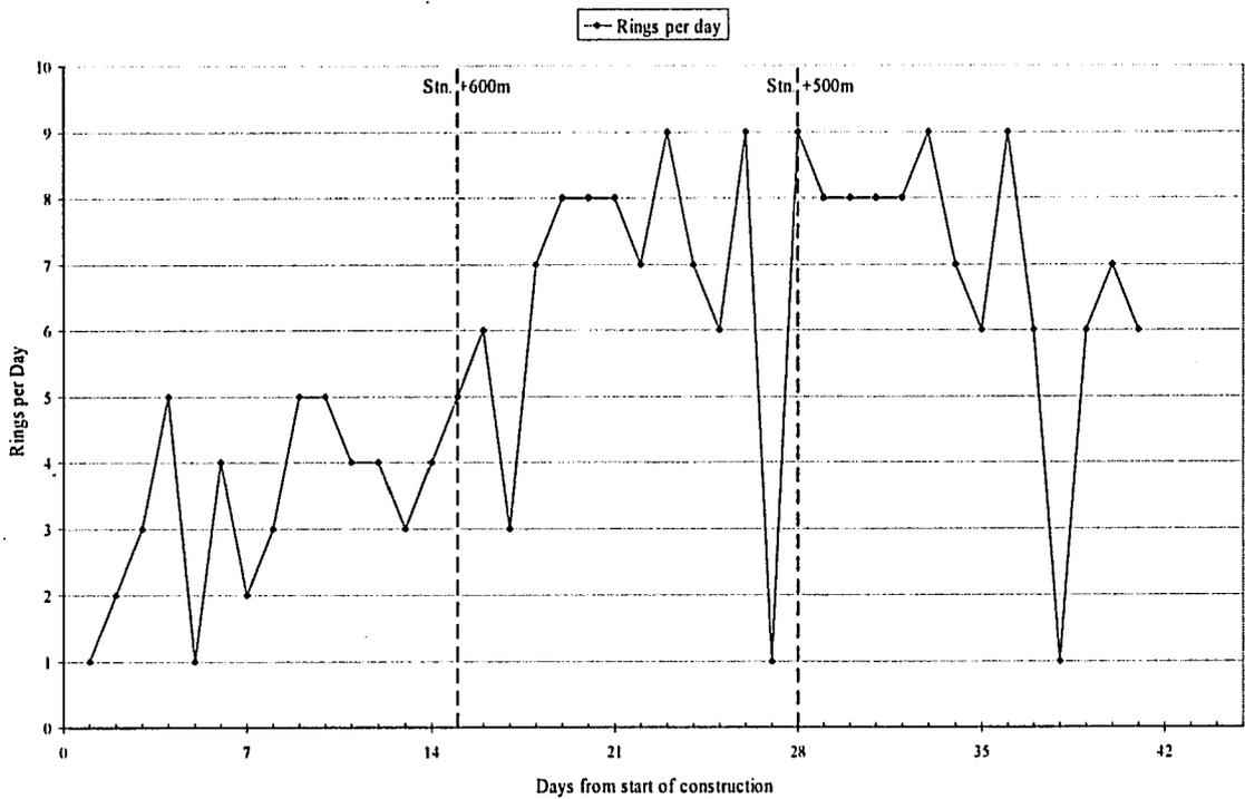
Figure 5-4 Rings constructed per day during construction of the Northbound Tunnel.
