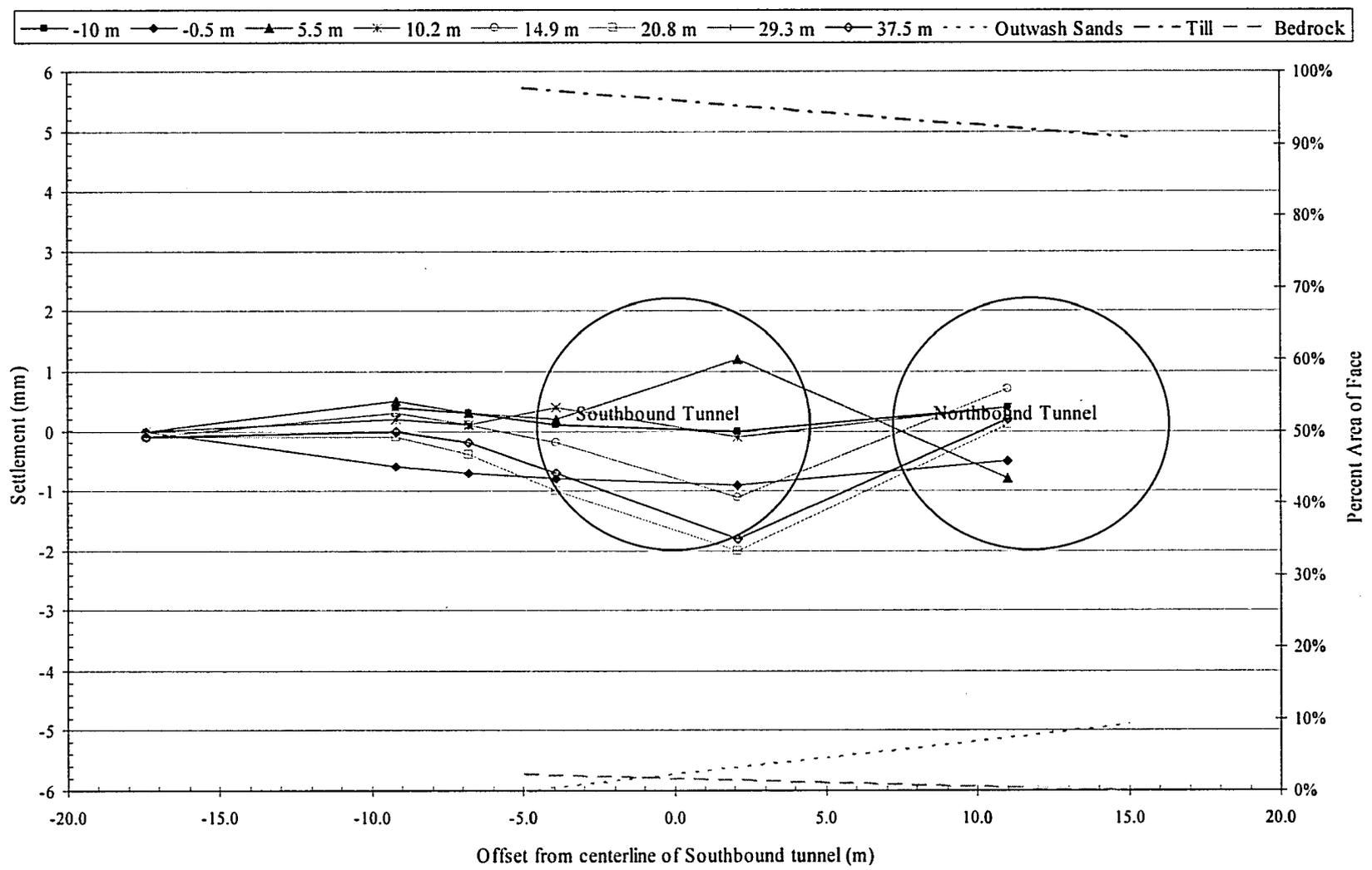
Figure H-5 Observed deep settlement at Array B during construction of Southbound Tunnel.
