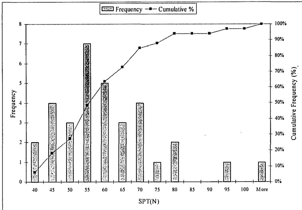
Figure 3-25 Histogram of SPT(N) blows per 150mm in Glacial Till.
