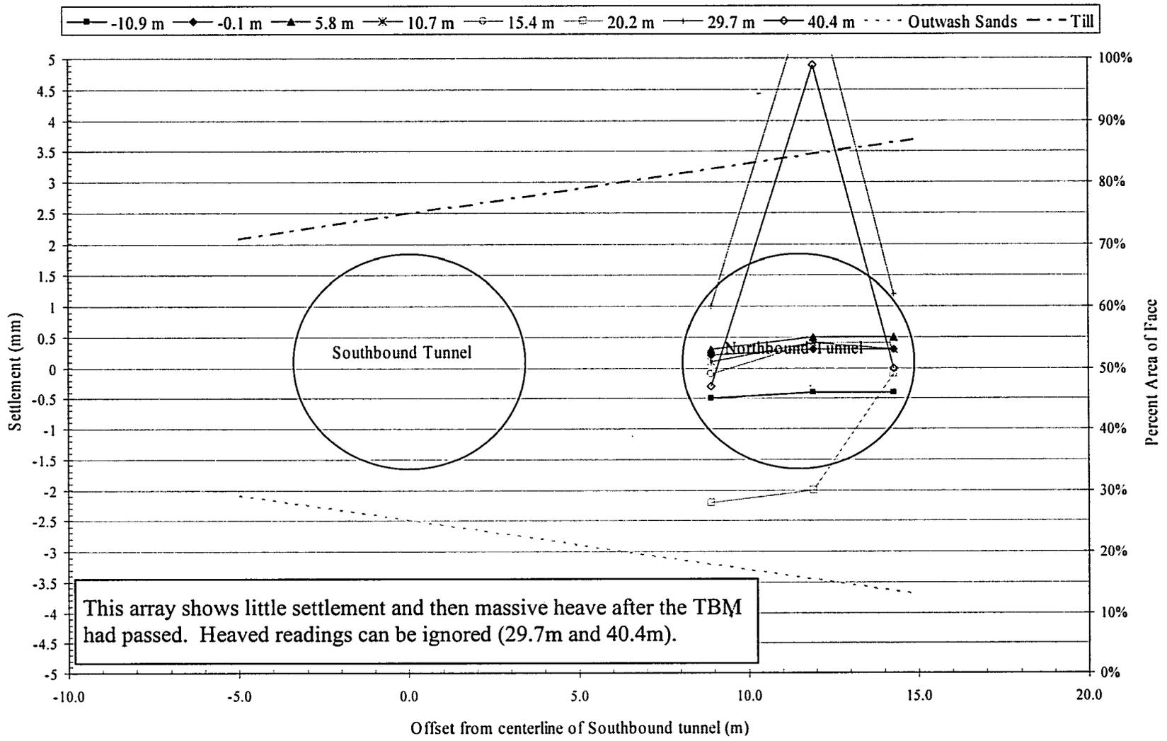
Figure H-4 Observed deep settlement at Array C during construction of Northbound Tunnel.
