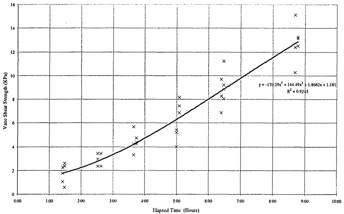
Figure 4-51 Strength development of grout sample.
