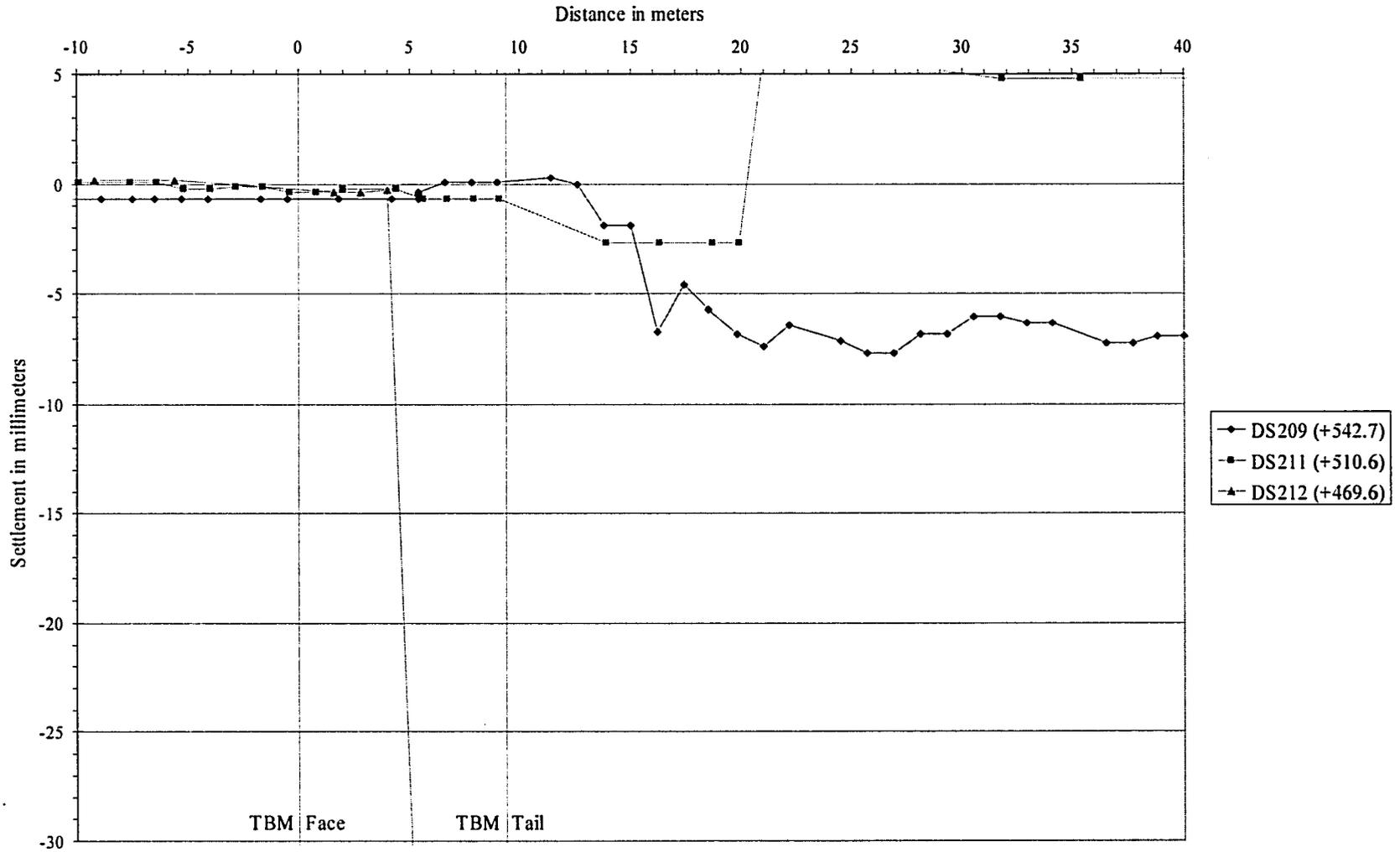
Figure G-5 Observed deep settlements during construction of Northbound Tunnel with proximity to TBM face, from Education Car Park to breakthrough.
