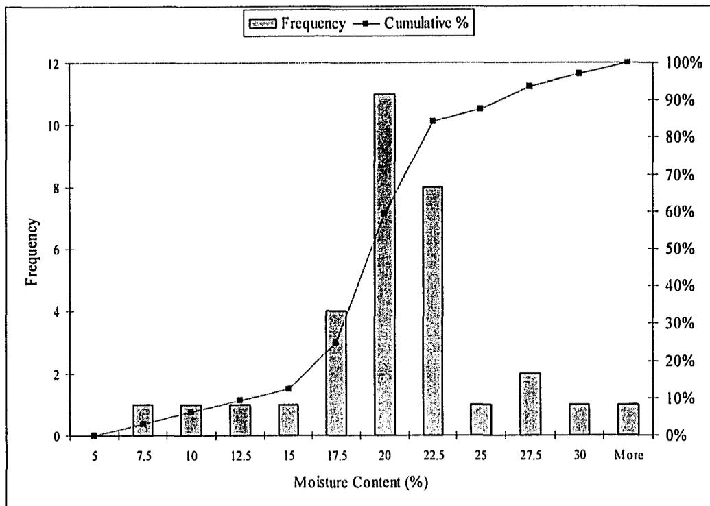
Figure 3-33 Histogram of observed Moisture Contents of the Bedrock.
