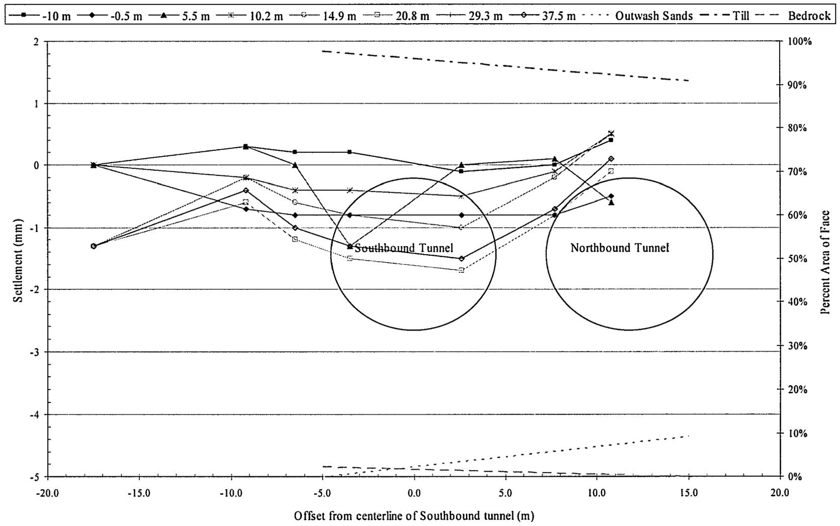
Figure 4-45 Observed shallow settlement at Array B during construction of Southbound Tunnel.
