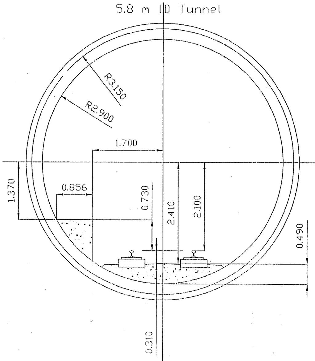
Figure 2-8 Dimensions of Finished Tunnel Cross Section
