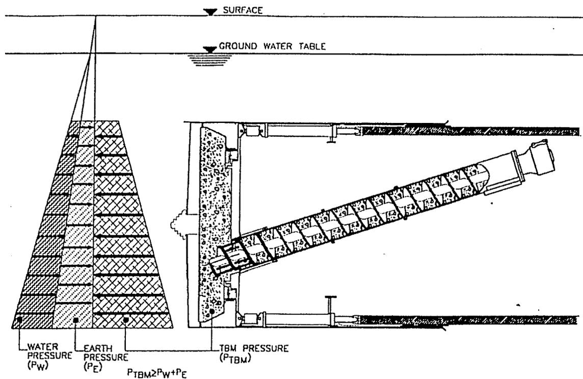
Figure 2-5 Principle of Equalised Pressure Balance (Lovat)
