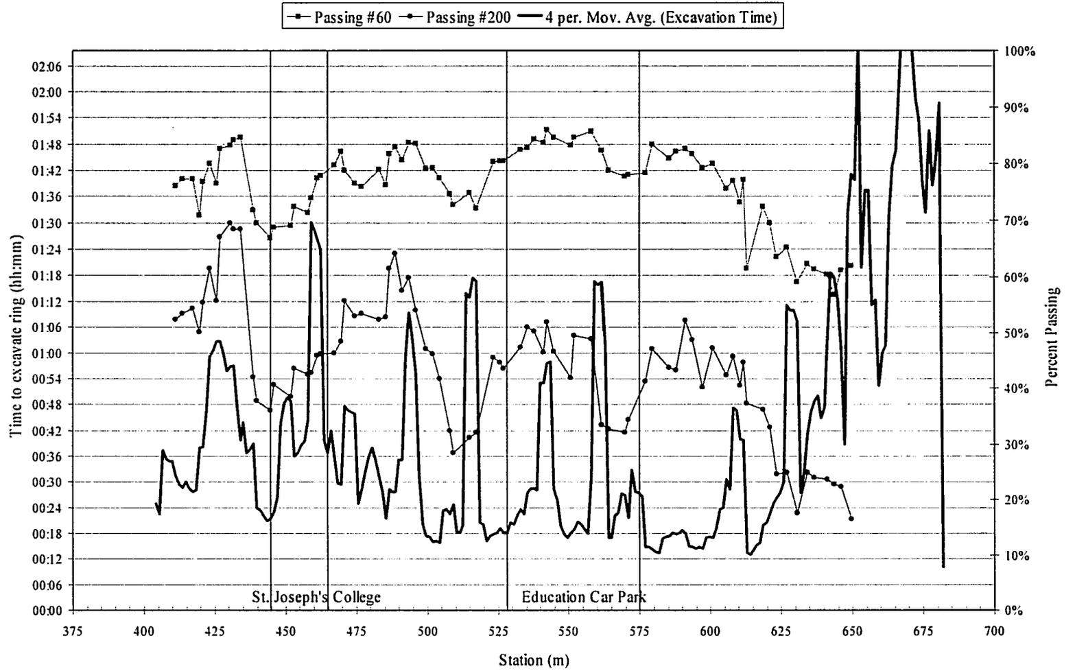
Figure 5-5 Excavation time per ring for construction of Southbound Tunnel with the fraction of soil passing the #60 and #200 sieve.
