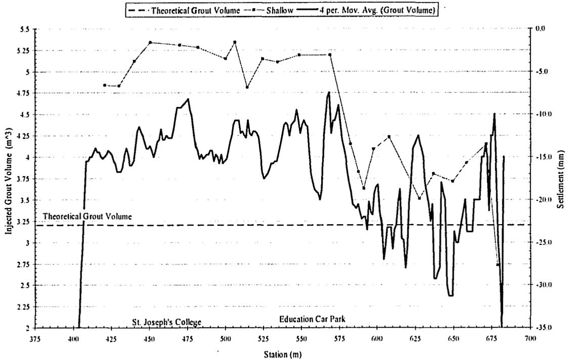
Figure 5-13 Injected grout volume per ring of advance during Southbound construction contrasted with observed shallow settlements.
