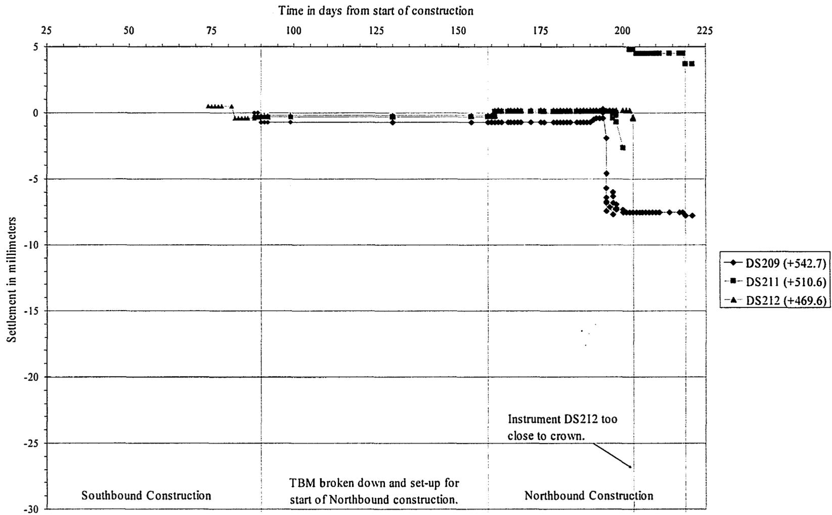
Figure G-10 Observed deep settlements in Northbound alignment instruments over the course of construction with respect to time, from Education Car Park to breakthrough.
