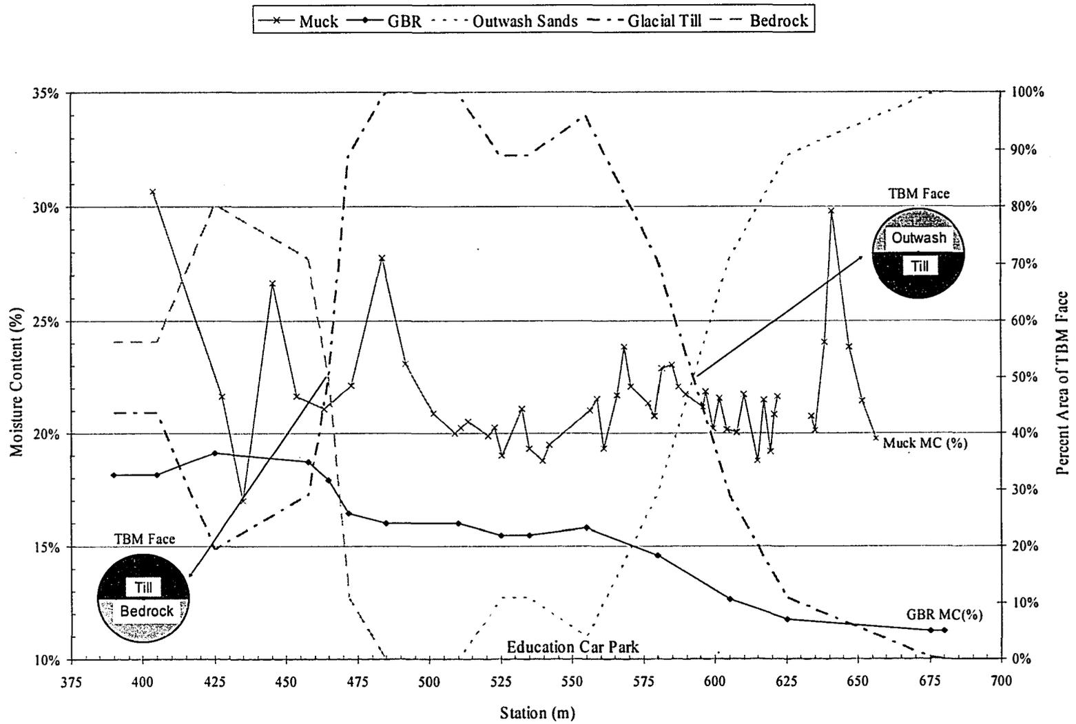
Figure 4-4 Moisture content of material excavated during construction of the Northbound LRT Tunnel and the inferred in-situ moisture content of the soil.
