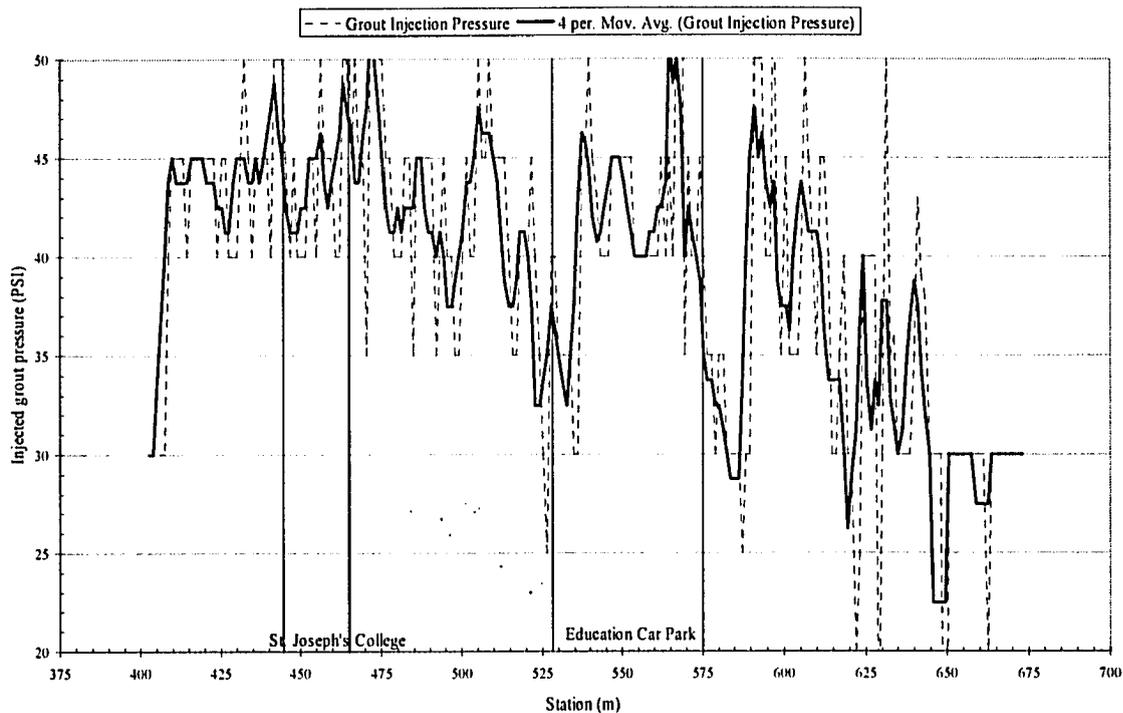
Figure 4-17 Injected grout pressure during Southbound construction.
