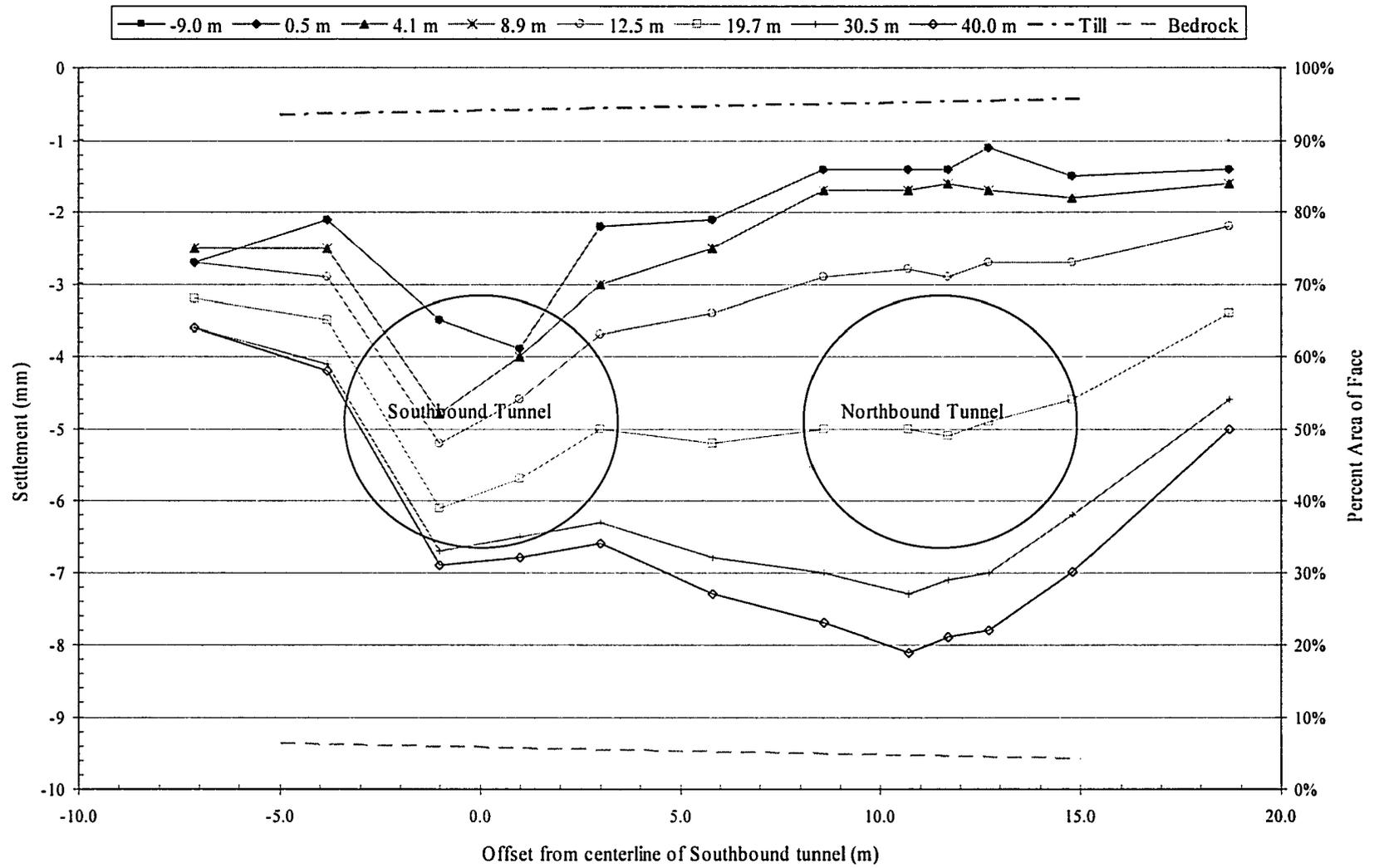
Figure 4-48 Observed shallow settlement at Array A during construction of Northbound Tunnel.
