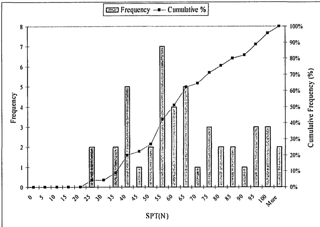
Figure 3-24 Histogram of SPT(N) blows per 300mm in Glacial Till.
