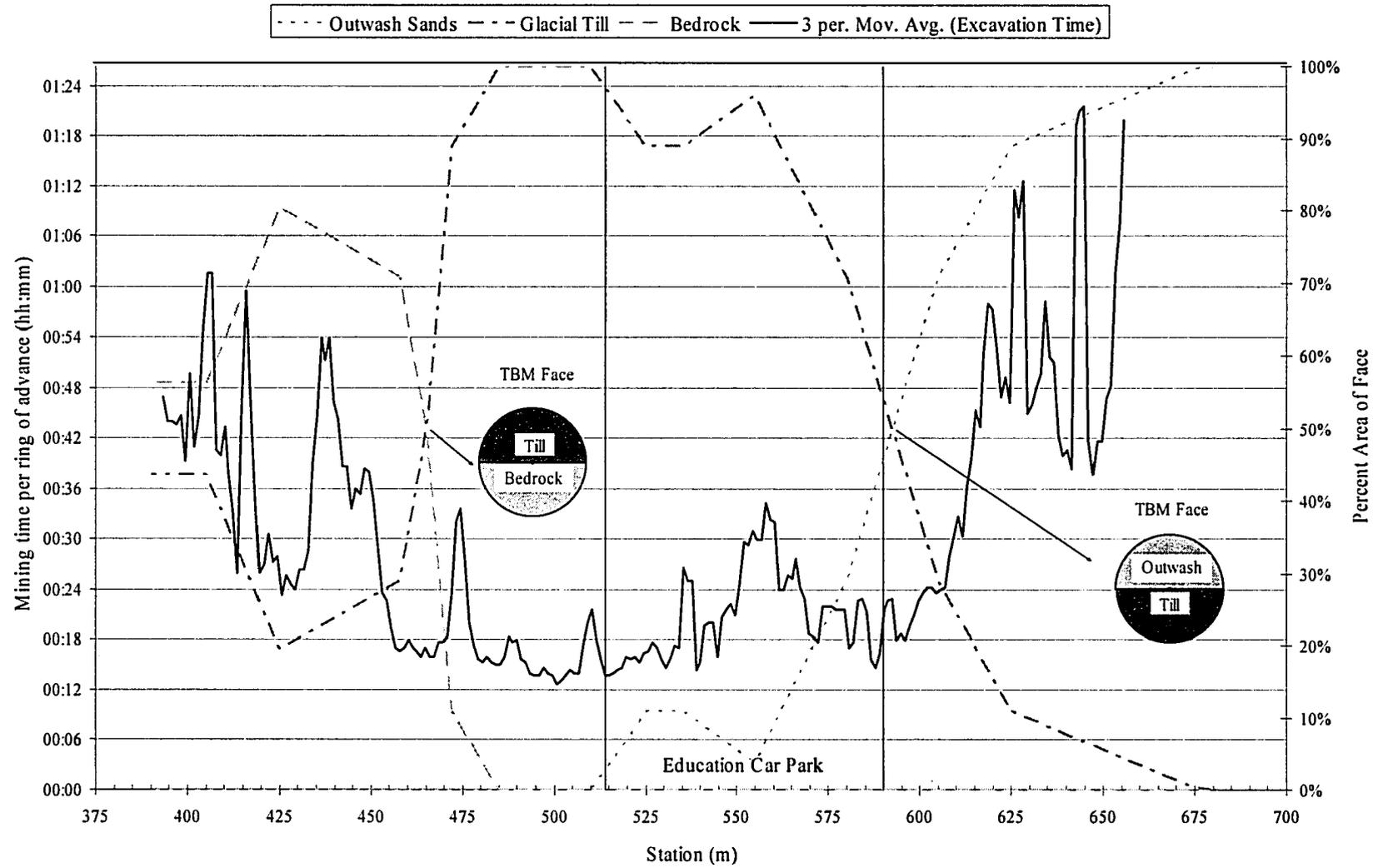
Figure 4-10 Time needed to excavate one ring during construction of Northbound LRT Tunnel.
