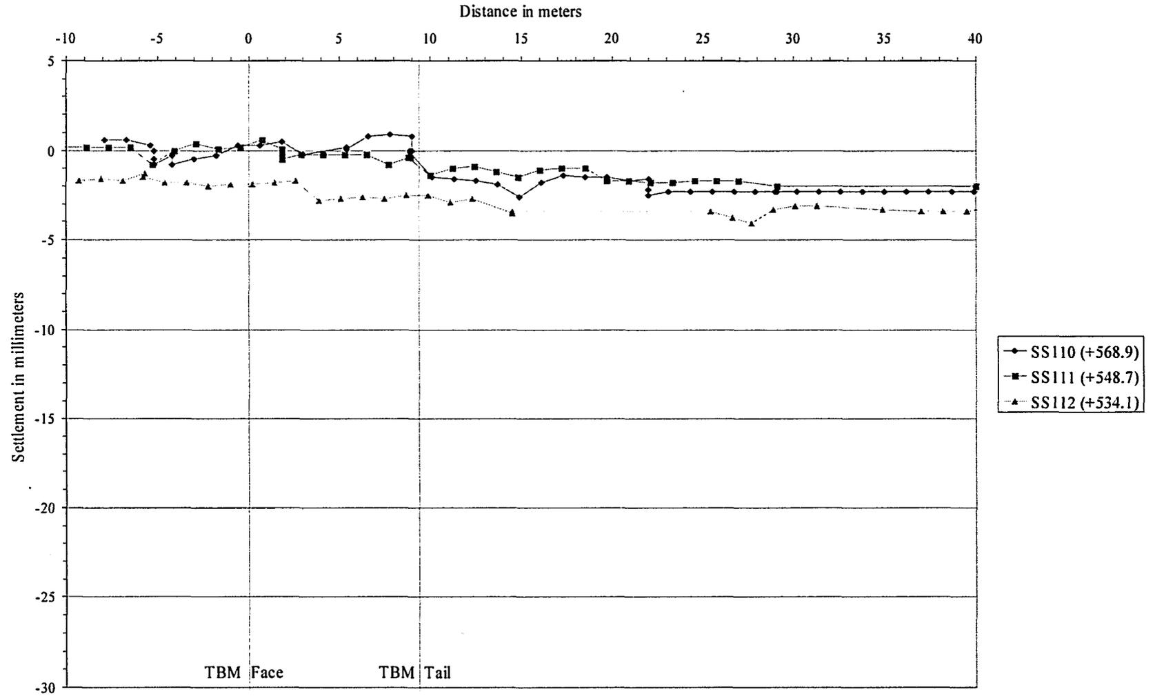
Figure 4-28 Observed shallow settlements during construction of Southbound Tunnel with proximity to TBM face, Education Car Park.
