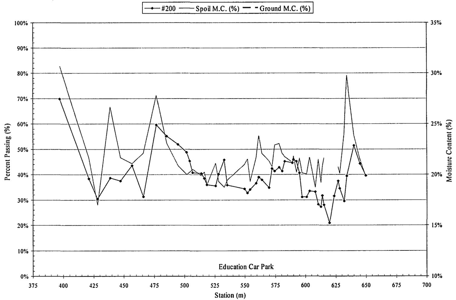
Figure 5-2 TBM spoil moisture content with inferred in-situ moisture content with the percentage of TBM spoil passing the #200 Sieve during Northbound construction.
