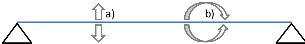
Figure 4.2 Flexion (a) and torsion (b) of an airfoil.
