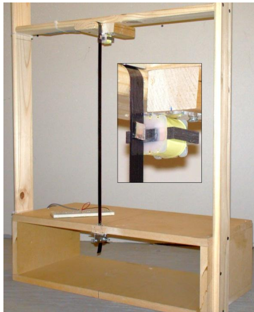
Figure 4.5 Picture of the wind flutter generator test bed.
