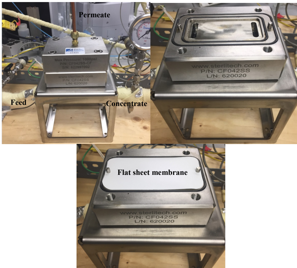
Figure 2.3: Images of filtration module
