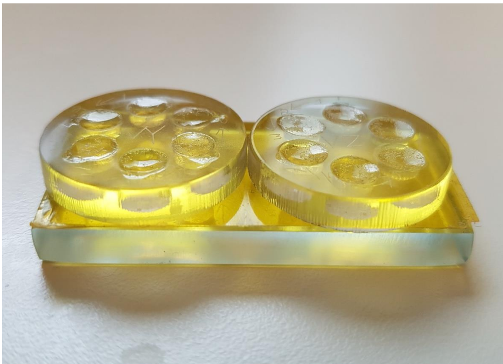
Figure 2.16: Two six-hole acrylic pucks placed on double-sided Kapton tape attached to a glass plate. Samples were individually placed into each hole, evaporated, covered in Specifix-20 epoxy, and labeled in a counter-clockwise orientation. Pucks are left at room temperature until fully cured (2-3 days for Specifix-20) before removing from tape.
