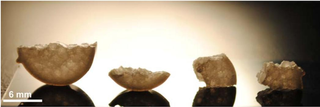
Fig. 4.7: Macrograph of the partially crystallized and quenched bioactive glass sample after it was **manually broken**.
