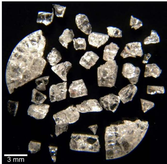
Fig. 4.4: Macrograph of shattered pieces of amorphous bioactive glass 45S5 after it was quenched from 680°C.
