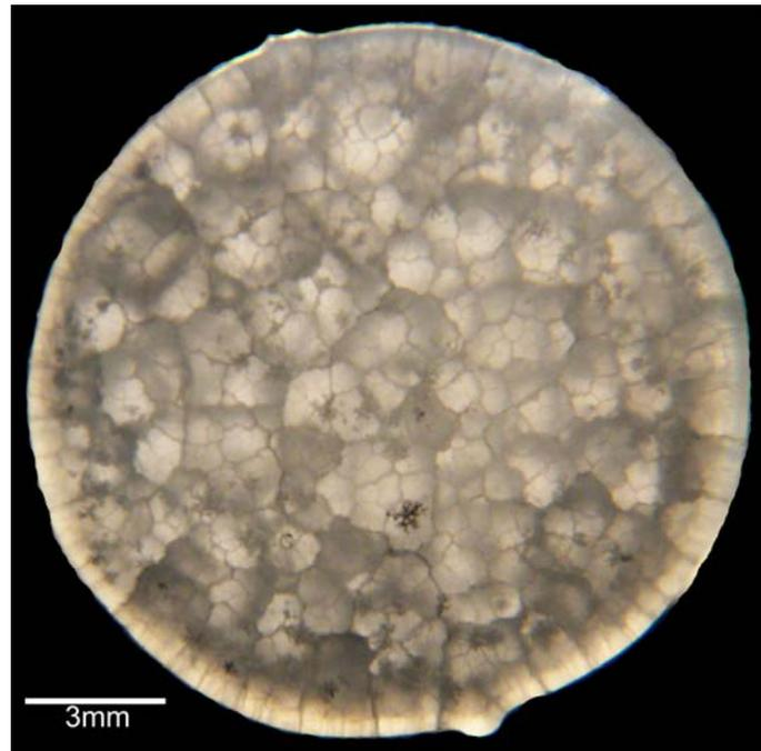
Fig. 4.6: Macrograph of a partially crystallized (crystallized at 680°C for 30 min, lower heating rate) bioactive glass 45S5 sample after it was quenched from 680°C.
