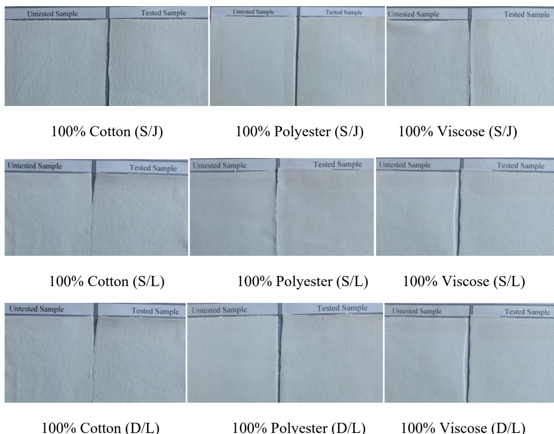
Figure-3. Picture of untested and tested sample during pilling test.
