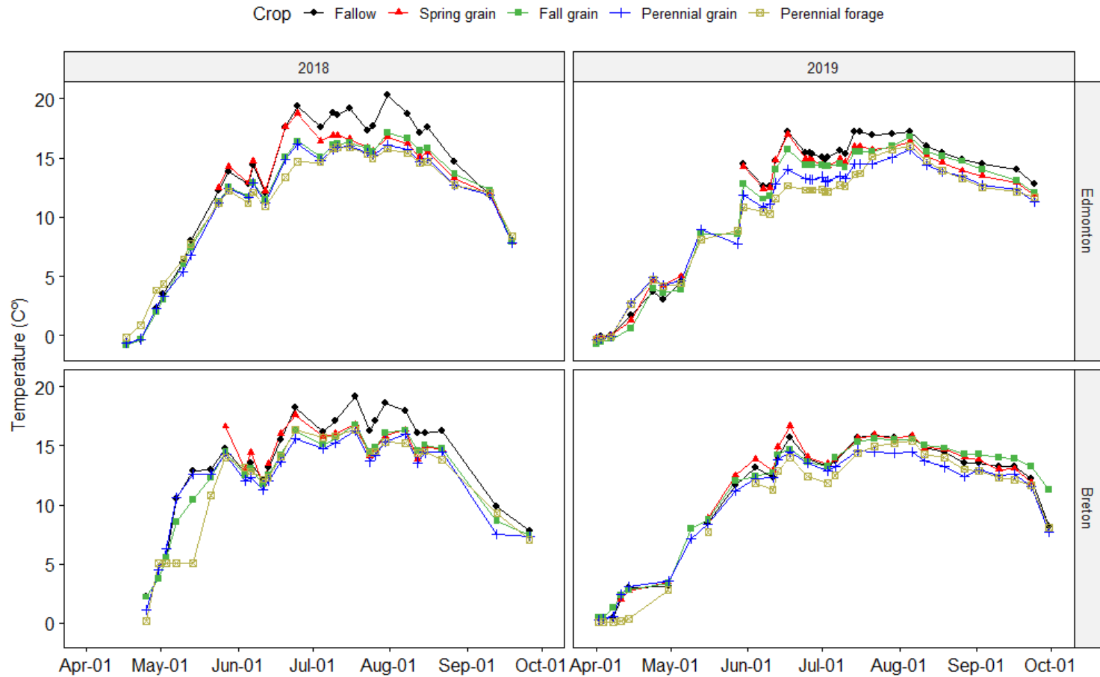
Fig. S1. 3. Soil temperature (40 cm depth) at the time of flux measurements over two consecutive growing seasons at the Edmonton and Breton sites.
