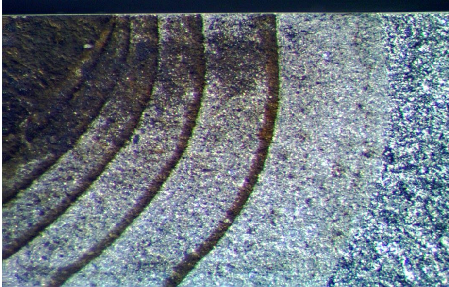
Figure 5-15 Close-up of a surface tip showing growth at the surface is lagging behind growth just beneath the surface.
