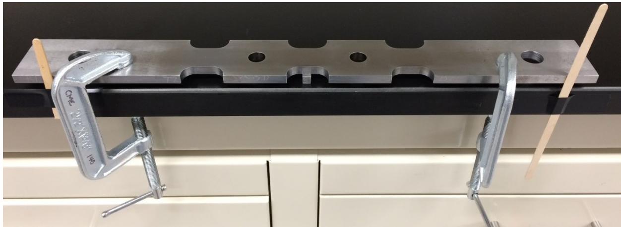
Figure 4-12 Demonstration of small bending load applied with clamps to open up the crack surface slightly so better replica cleaning results can be obtained.
