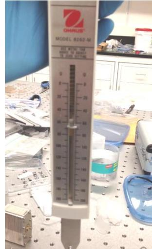
**Figure 5.34: Fiber array peel test method using fish scale.**
