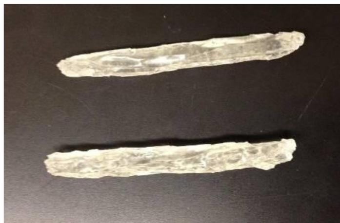
**Figure 2.6: Image of Kraton G1657 sticks for glue gun processing.**
