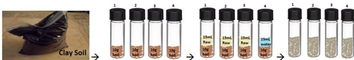
Figure 4-1 Sequence to produce vials with soil-sewage or soil-water, then mixed for HF183 decay study
