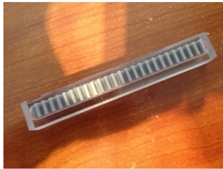
Figure 3.2. Plastic rack used to create strain relief in leads
