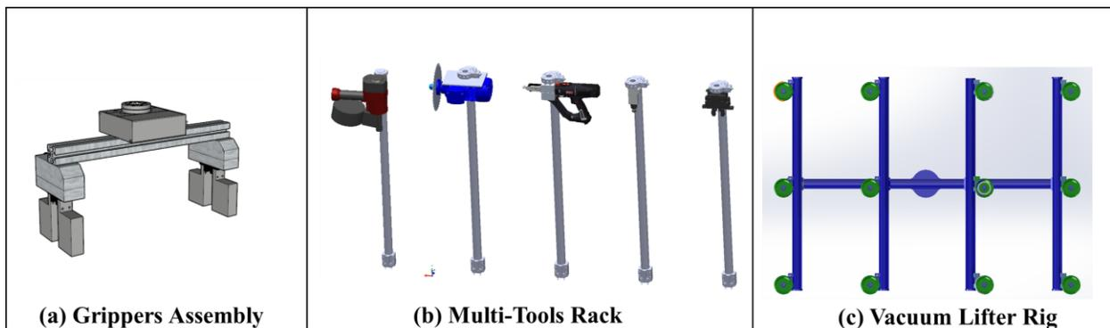
Figure 78. Robot End-Effectors
