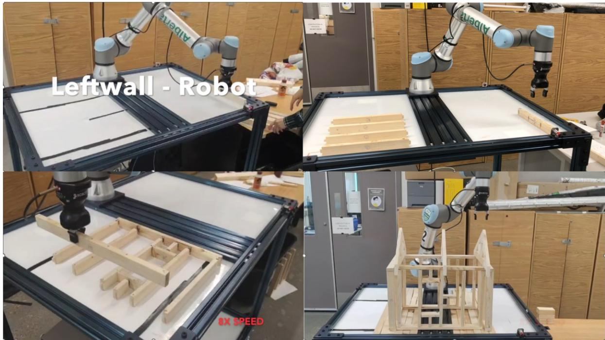
Figure 149. In-Lab Scaled Testing Experiment of the Developed RMP for Obstacle Avoidance
