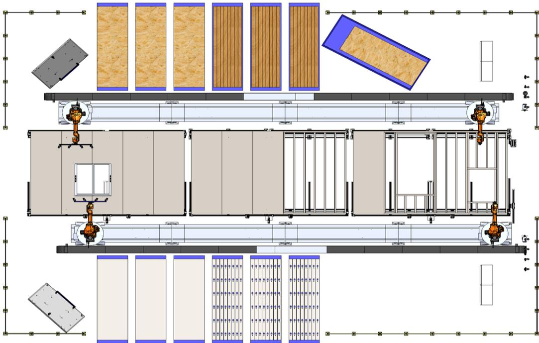
Figure 85. Simulation Result for Robotic Cell with LGS Framing and Sheathing
