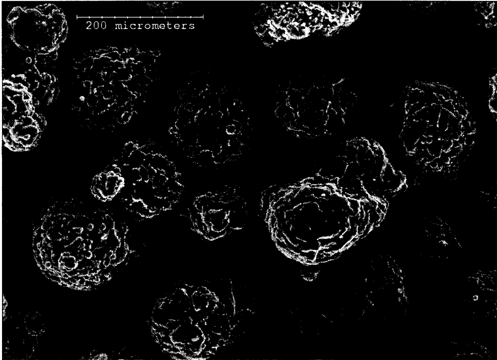
Figure C.1 SEM of Pharmatose. Scale bar is 200 \mu m.
